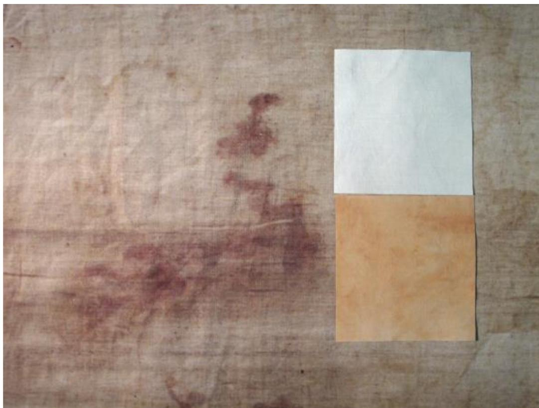
**Figure 4.** Photo of the foot on the dorsal image of the TS onto which are superimposed for comparison a white fabric and the same white fabric colored with iron oxide having an areal density of iron of  $58 \mu\text{g}/\text{cm}^2$ .
