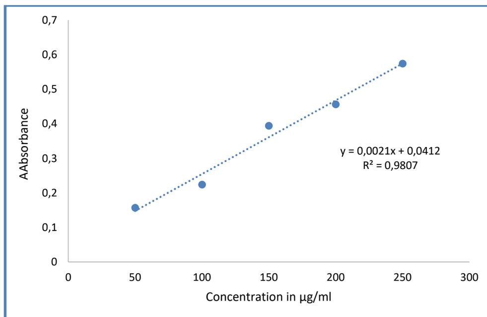
**Figure 7.** Calibration line for standard Ascorbic acid.
