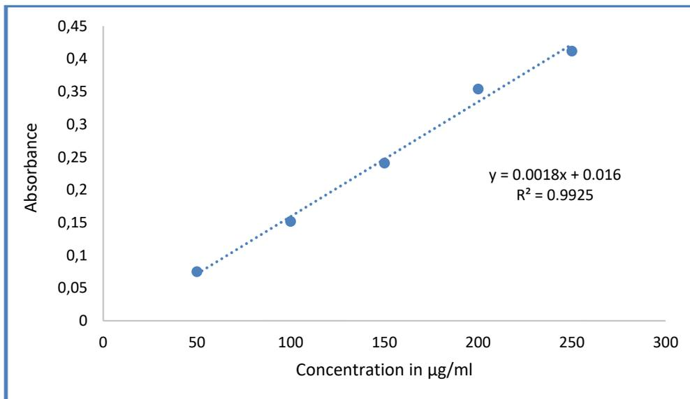
Figure 2. Calibration line for standard Ajmalicine.
