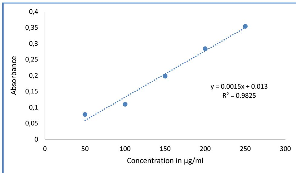
Figure 3. Calibration line for standard Quercetin.
