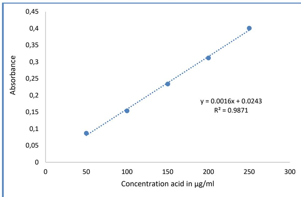
**Figure 5.** Calibration line for standard Tannic acid.
