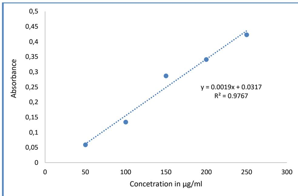
**Figure 6.** Calibration line for standard Oleanolic acid.
