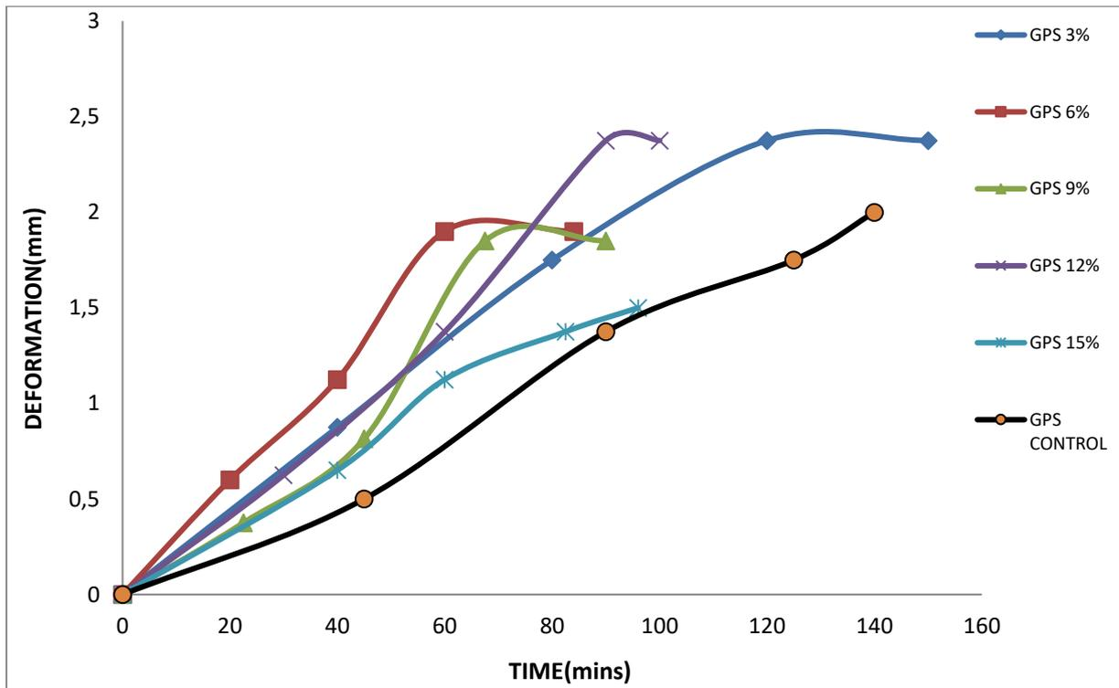
**Fig. 2a.** Deformation Curves of the Control (PS) and PS-Coconut Shell Composites at 3% - 15% Filler Levels
