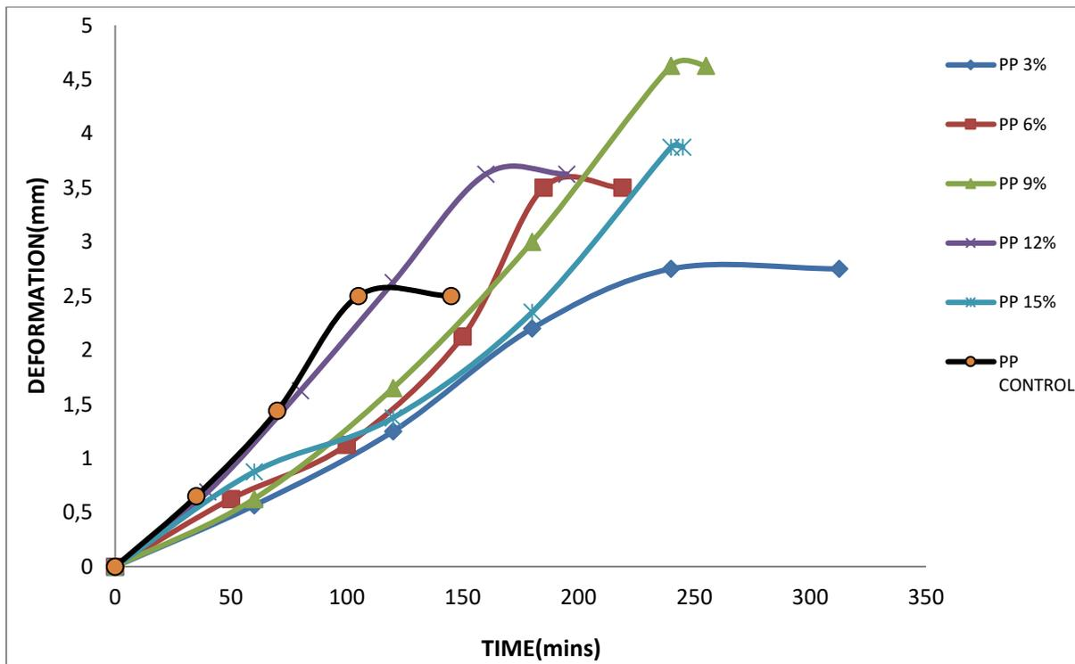
**Fig. 3a.** Deformation Curves of the Control (PP) and PP-Coconut Shell Composites at 3% - 15% Filler Levels
