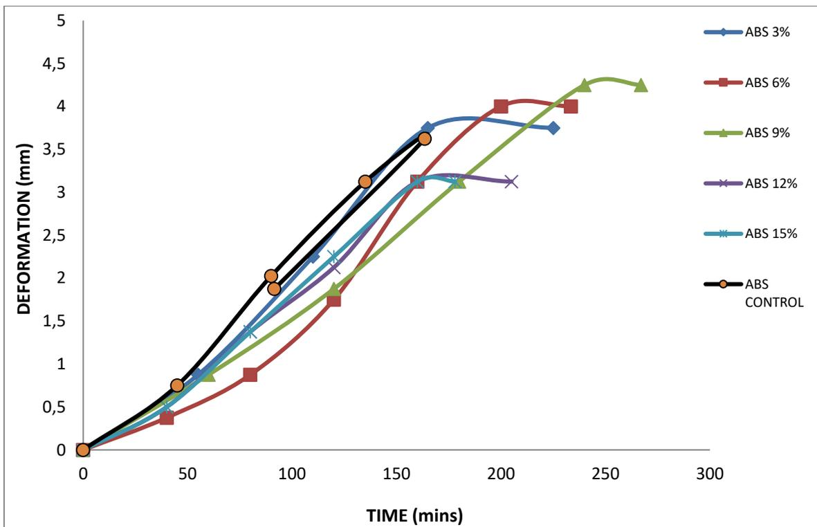
**Fig. 4a.** Deformation Curves of the Control (ABS) and ABS-Coconut Shell Composites at 3% - 15% Filler Levels
