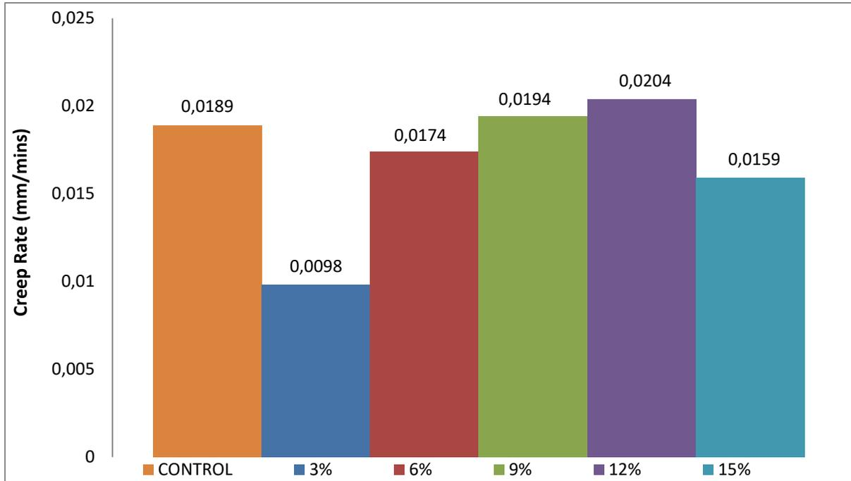
**Fig. 3b.** Creep Rate Values of the Control (PP) and PP-Coconut Shell Composites at 3% - 15% Filler Levels
