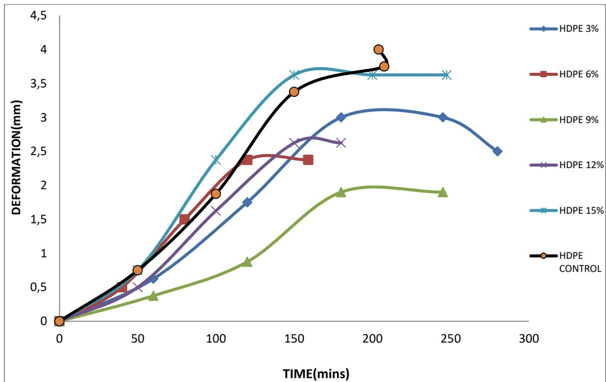
**Fig. 1a.** Deformation Curves of the Control (HDPE) and HDPE-Coconut Shell Composites at 3% - 15% Filler Levels
