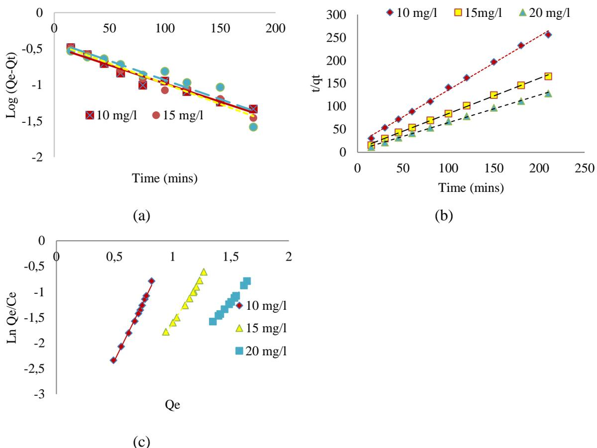
**Figure 6.** (a) Pseudo-first order kinetics (b) Pseudo-second order (c) Elovich model of the adsorption of BB on modified BAG
