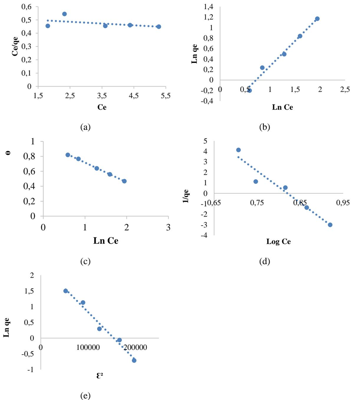
**Figure 5.** (a) Langmuir (b) Freundlich (c) Temkin (d) Harkins- (d) Hill-de Boer (e) Dubinin-Radushkevich Isotherm models of the adsorption of BB on modified BAG
