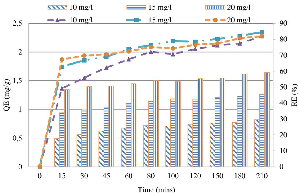
**Figure 4.** Effect of concentration on the adsorption of BB on modified BAG.
