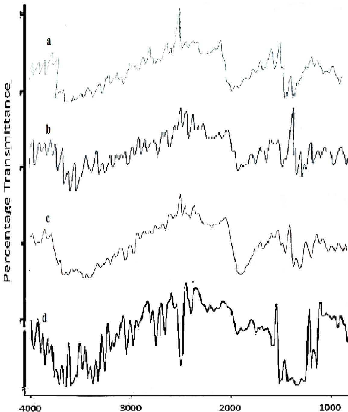
**Figure 3.** FTIR spectra of (a) *Gliricidia sepium* unmodified, (b) *Gliricidia sepium* modified (c) *Acacia* unmodified, (d) *Acacia* modified.
