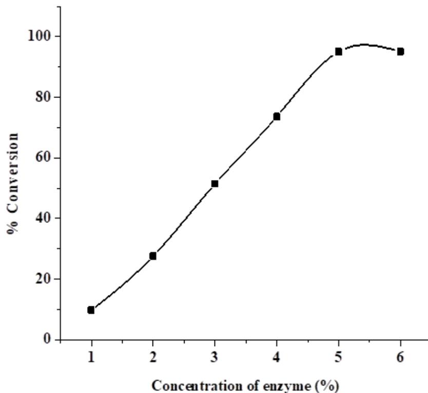
Figure 6. Analysis of enzyme concentration for % conversion of biodiesel
