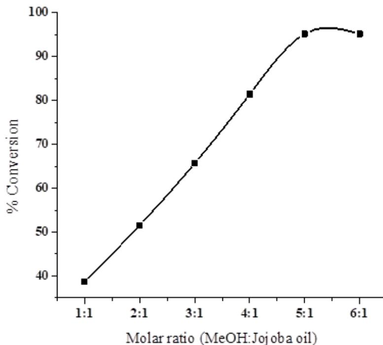
**Figure 2.** Analysis of molar ratio of alcohol to jojoba oil vs % conversion of biodiesel
