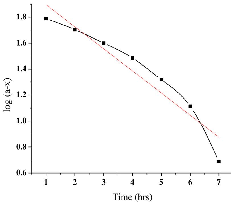
**Figure 3.** Kinetic analysis of plot of log(a-x) vs time (hrs) with molar ratio 5:1 (MeOH : Jojoba oil)
