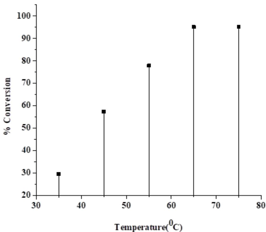
**Figure 4.** Analysis of temperature for % conversion of biodiesel
