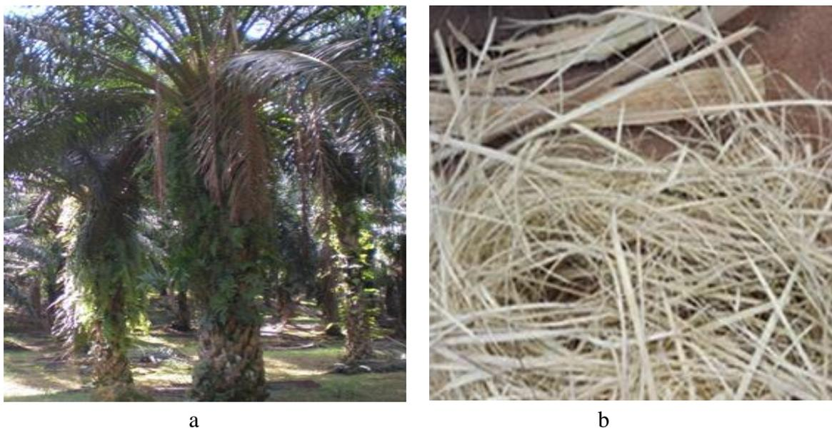
**Figure 1(a,b).** (a) Oil palm tree and (b) mechanically extracted oil palm petiole fiber (OPPF)
