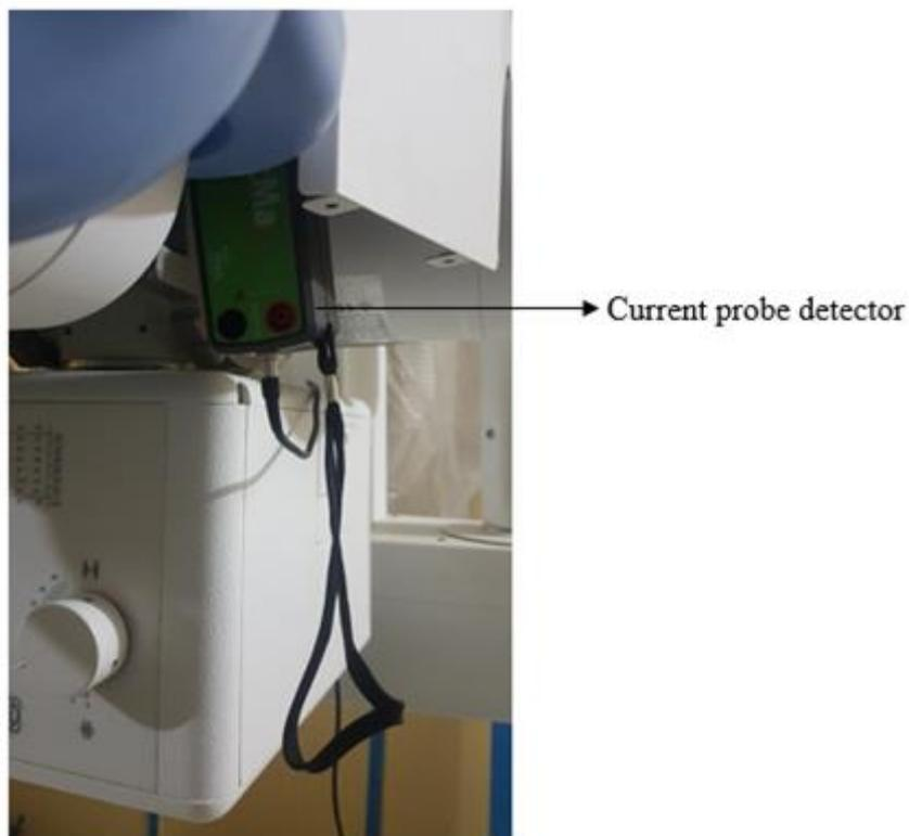
**Figure 2.** Attachment of the current probe detector to the cathode cable
