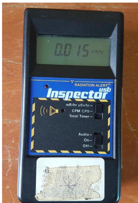
**Figure 3.** Calibrated survey meter used for leakage test
