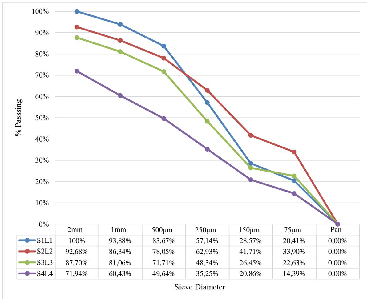
**Figure 3.** Particle Size Distribution Curve of Okpe Schist
