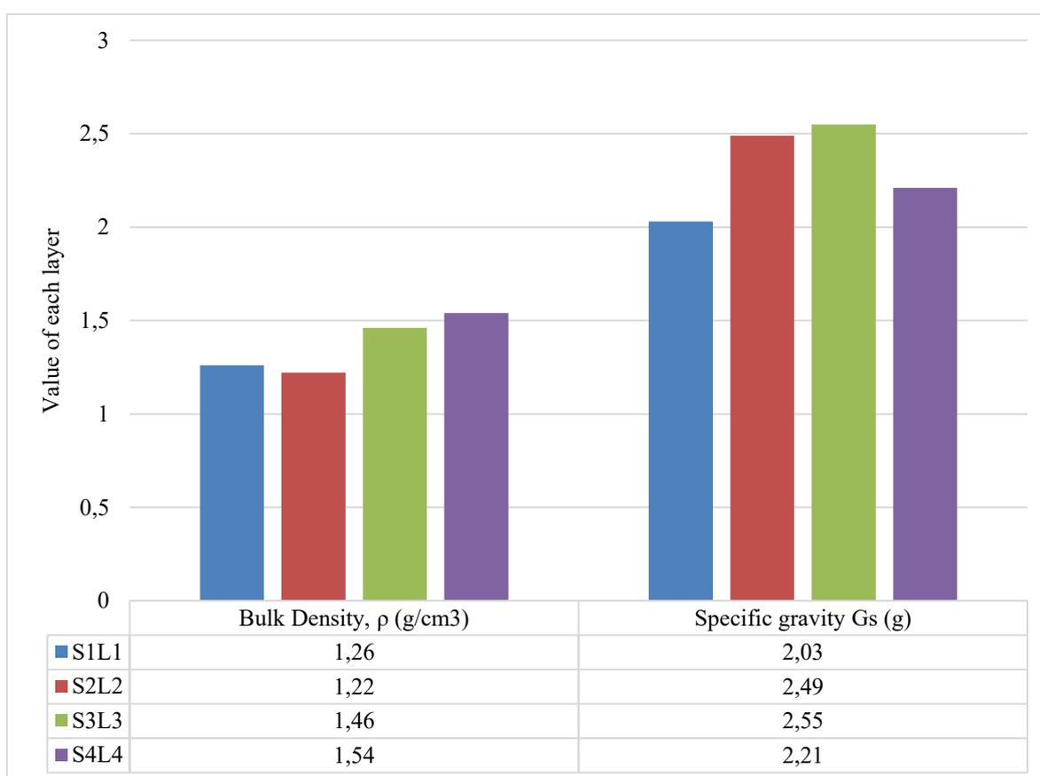
**Figure 4.** Bulk Density and Specific Gravity of Okpe Schist
