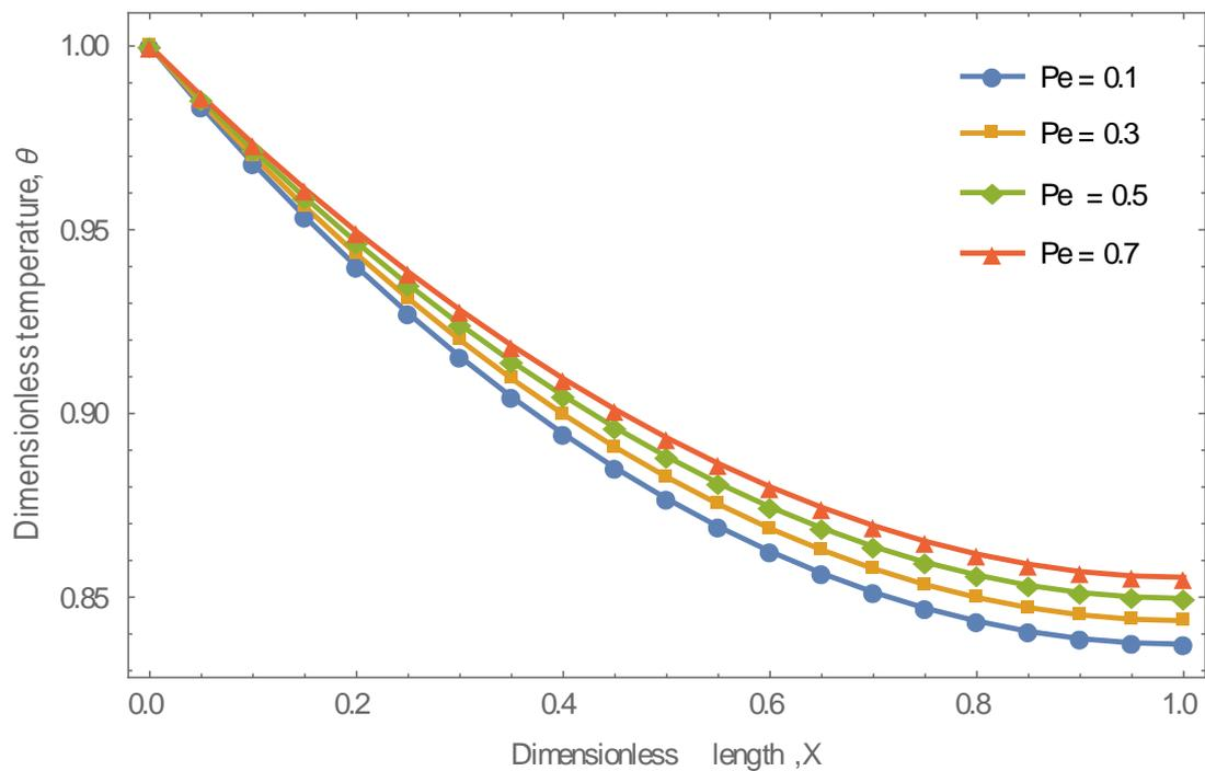
**Fig. 4.** Dimensionless temperature distribution in the fin parameters for varying pecket number when  $\beta = 0.2$ ;  $M = 0.3$ ;  $S_p = 0.5$ ;  $G = 0.4$ ;  $H_t = 0.6$
