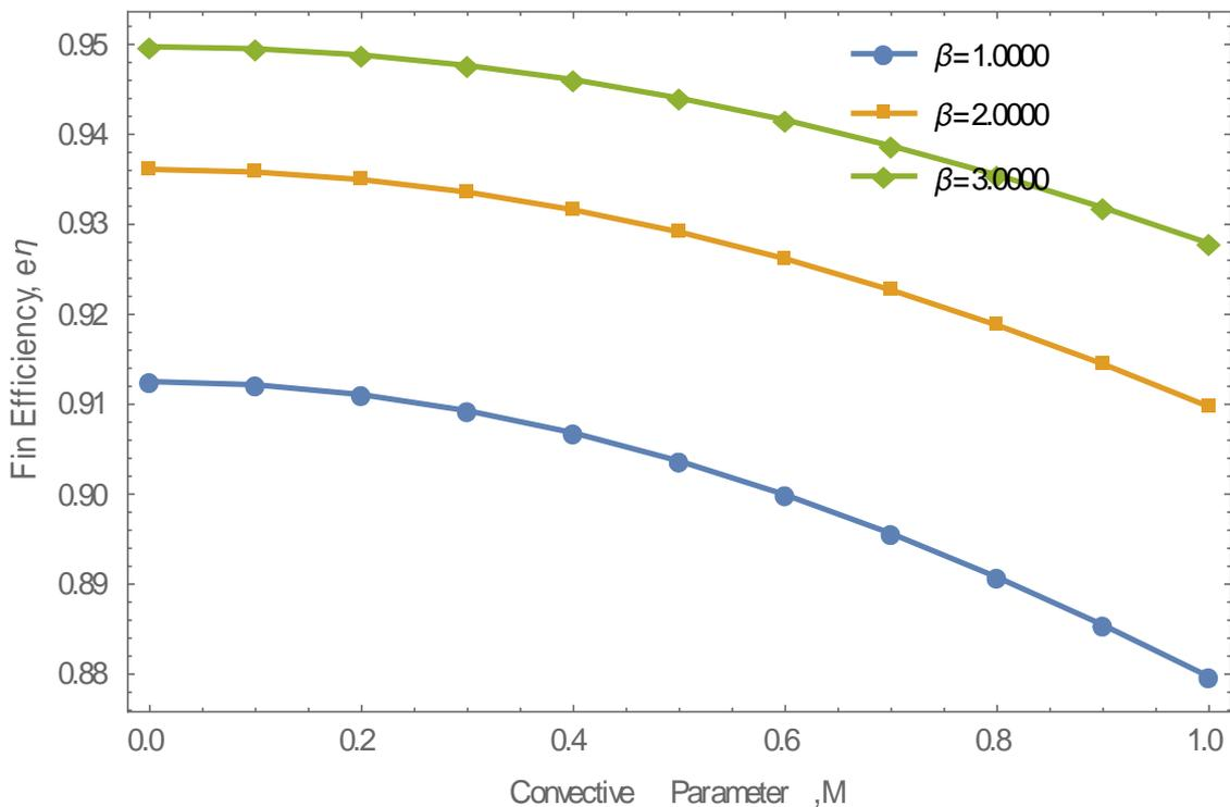
**Fig. 8.** Efficiency versus convective for  $H_t = 0.6$ ;  $S_p = 0.7$ ;  $G = 0.4$ ;  $Pe = 0.5$
