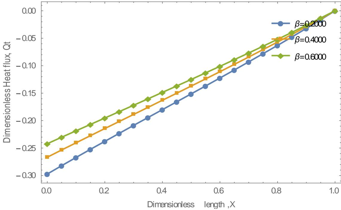
**Fig. 11.** Heat flux across fin length for varying thermal conductivity parameter  $H_t = 0.6$ ;  $M = 0.3$ ;  $S_p = 0.5$ ;  $G = 0.4$ ;  $Pe = 0.5$ ;
