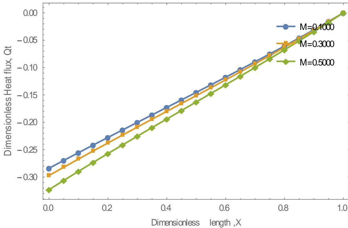
**Fig. 12.** Heat flux across fin length for varying convective parameter  $\beta = 0.2$ ;  $H_t = 0.6$ ;  $M = 0.5$ ;  $G = 0.4$ ;  $Pe = 0.5$
