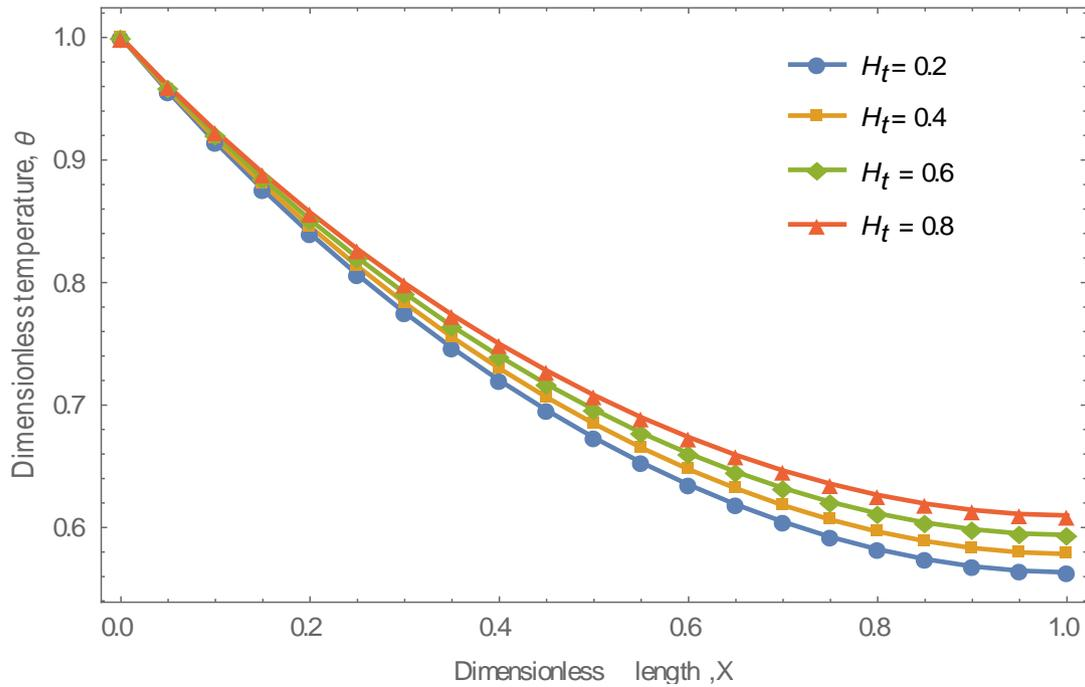
**Fig. 6.** Dimensionless temperature distribution in the fin parameters for varying internal heat generation parameter when  $\beta = 2$ ;  $M = 2$ ;  $S_p = 5$ ;  $Pe = 2$ ;  $G = 0.4$
