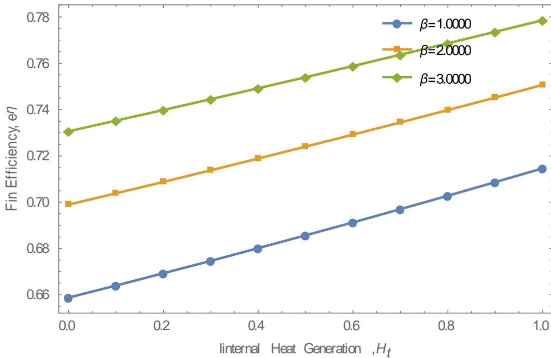
**Fig. 10.** Efficiency versus internal heat generation for varying Thermal conductivity parameter when  $M = 2; S_p = 5; G = 0.4; Pe = 2$
