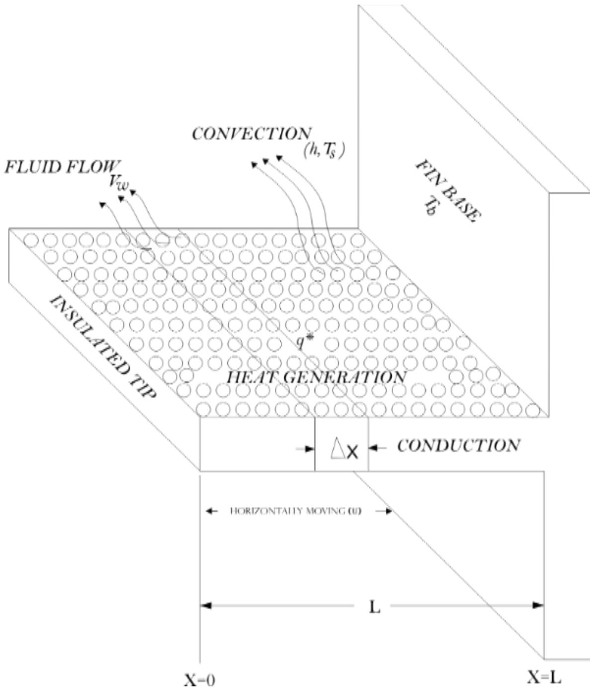
**Fig. 1.** Schematic of the convective longitudinal porous fin.
