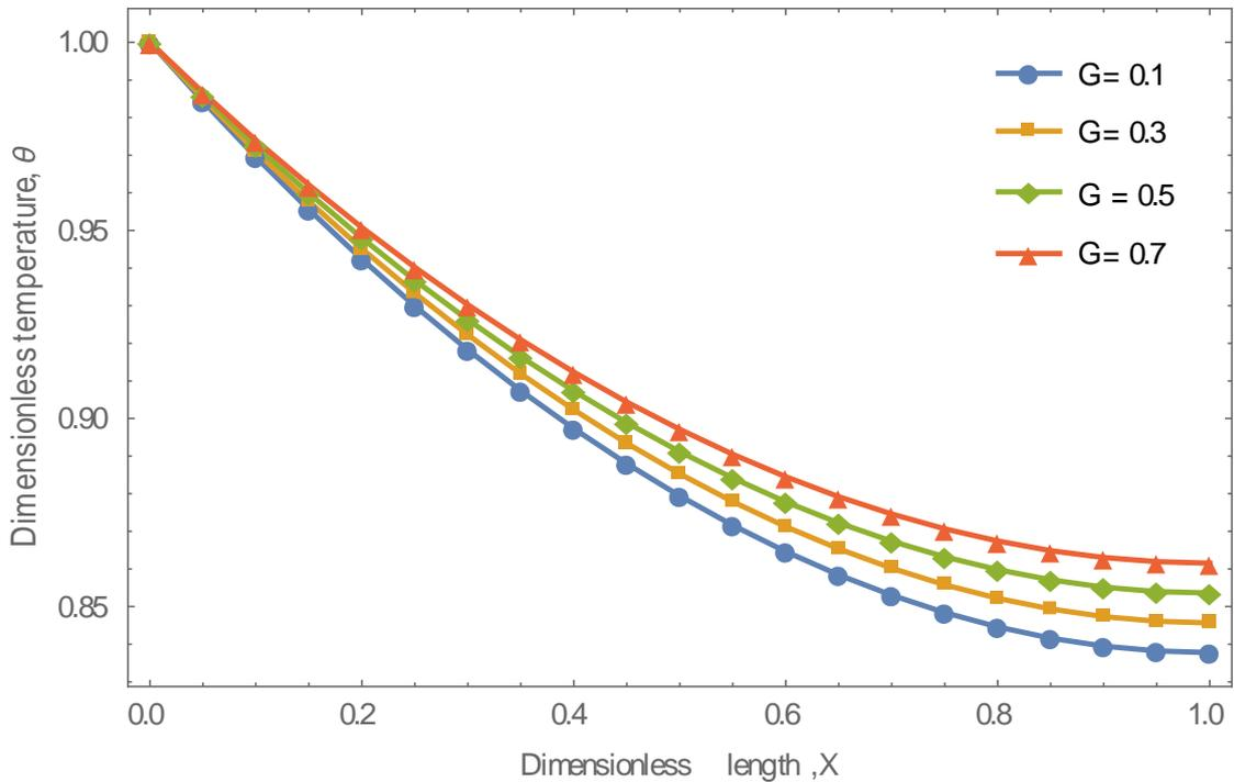
**Fig. 7.** Dimensionless temperature distribution in the fin parameters for varying generation parameter when  $\beta = 0.2$ ;  $M = 0.3$ ;  $S_p = 0.5$ ;  $Pe = 0.5$ ;  $H_t = 0.6$
