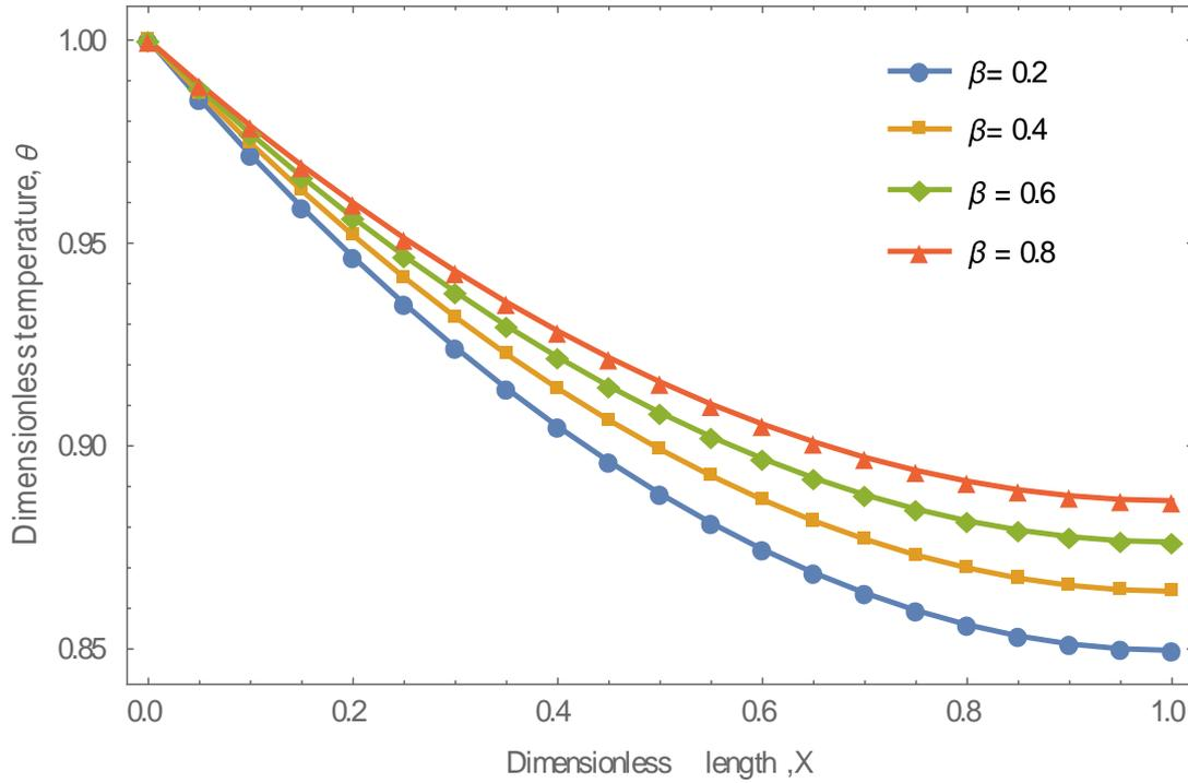
**Fig. 5.** Dimensionless temperature distribution in the fin parameters for varying thermal conductivity parameter when  $S_p = 0.5$ ;  $Pe = 0.5$ ;  $G = 0.4$ ;  $H_t = 0.6$ ;  $M = 0.3$
