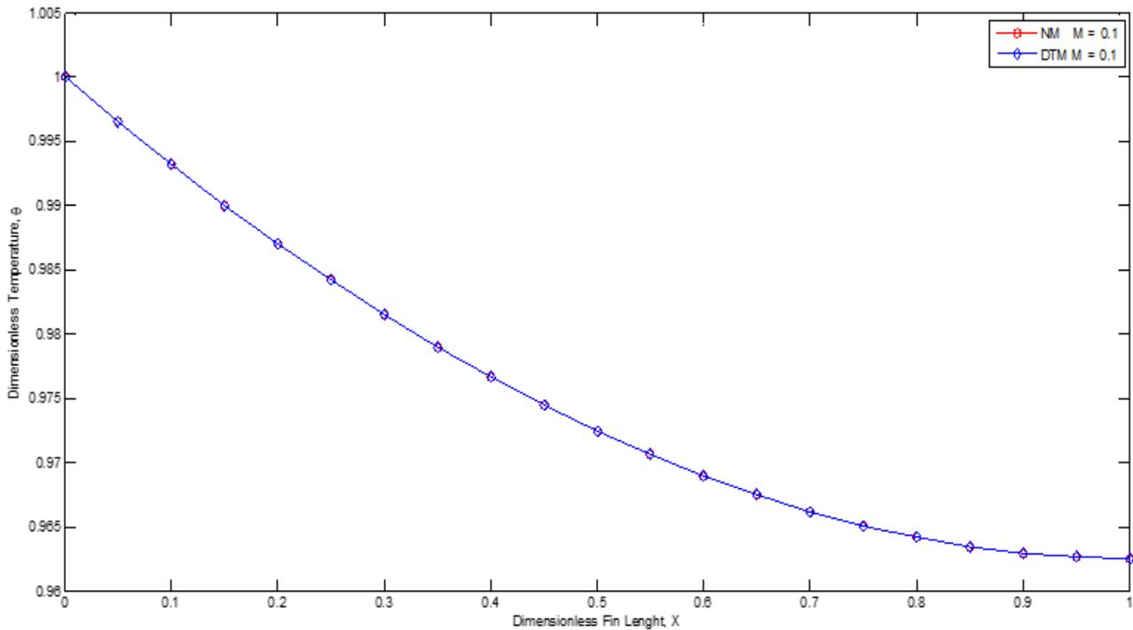
**Fig. 14.** Dimensionless temperature distribution in the fin parameters for varying convective parameter when  $\beta = 0.2$ ;  $S_p = 0.1$ ;  $Pe = 0.5$ ;  $G = 0.1$ ;  $H_t = 0.1$
