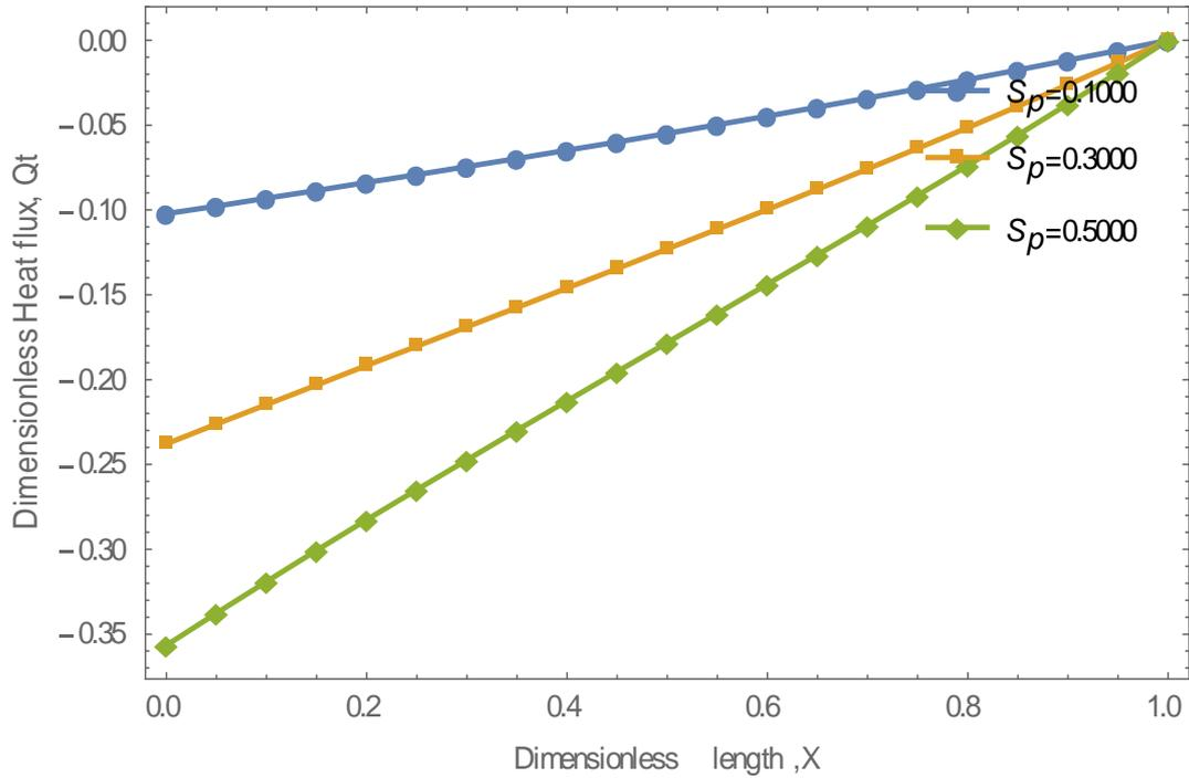
**Fig. 13.** Heat flux across fin length for varying porosity  $\beta = 0.2$ ;  $H_t = 0.6$ ;  $0.5$ ;  $G = 0.4$ ;  $Pe = 0.5$
