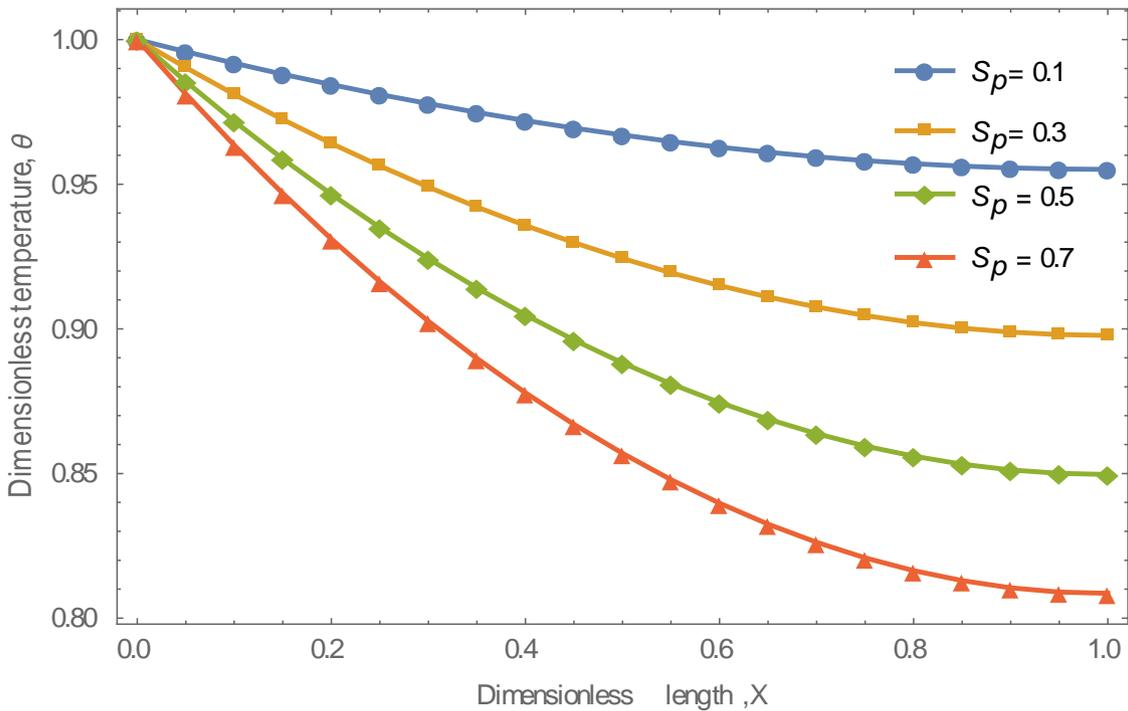
**Fig. 2.** Dimensionless temperature distribution in the fin parameters for varying porosity parameters when  $\beta = 0.2$ ;  $M = 0.3$ ;  $Pe = 0.5$ ;  $G = 0.4$ ;  $H_t = 0.6$
