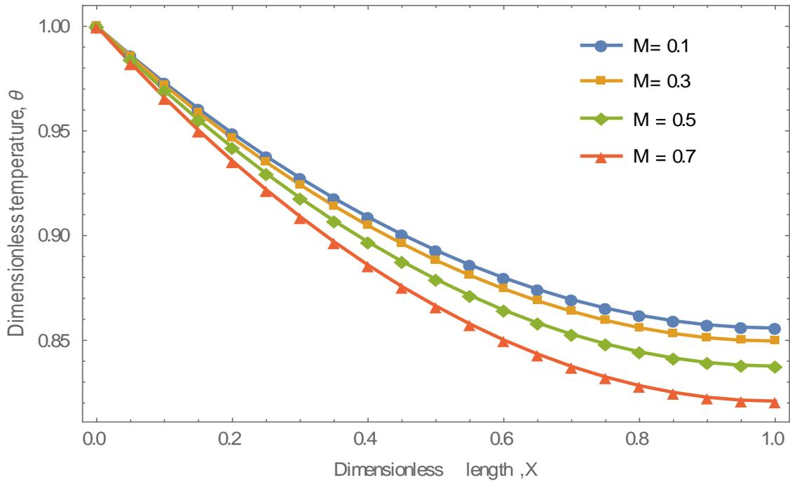
**Fig. 3.** Dimensionless temperature distribution in the fin parameters for varying thermo geometric parameters when  $\beta = 0.2$ ;  $S_p = 0.5$ ;  $Pe = 0.5$ ;  $G = 0.4$ ;  $H_t = 0.6$
