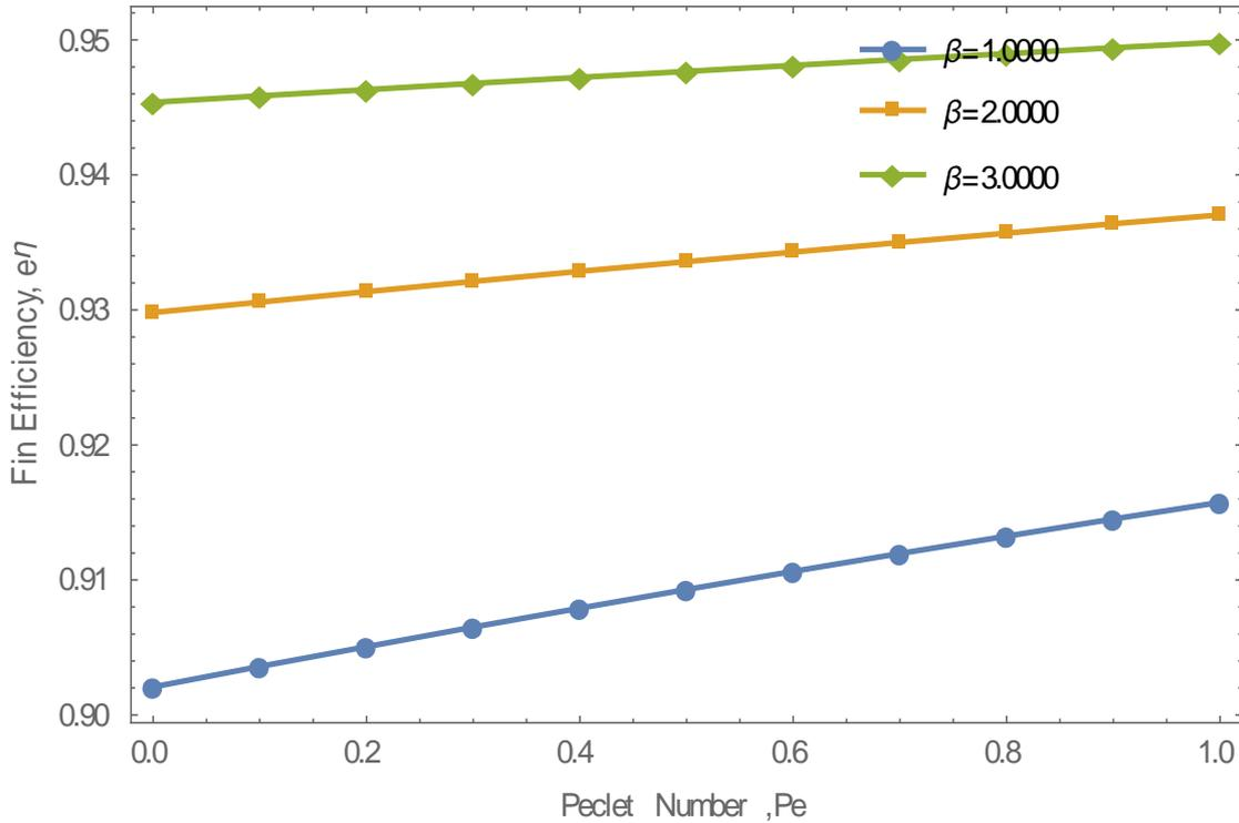
**Fig. 9.** Efficiency versus Peclet number for varying thermal conductivity parameter when  $H_t = 0.6; M = 0.3; S_p = 0.7; G = 0.4$
