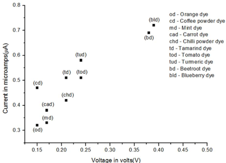
Figure 4. I-V Characteristic curve of DSSC based on natural dyes
