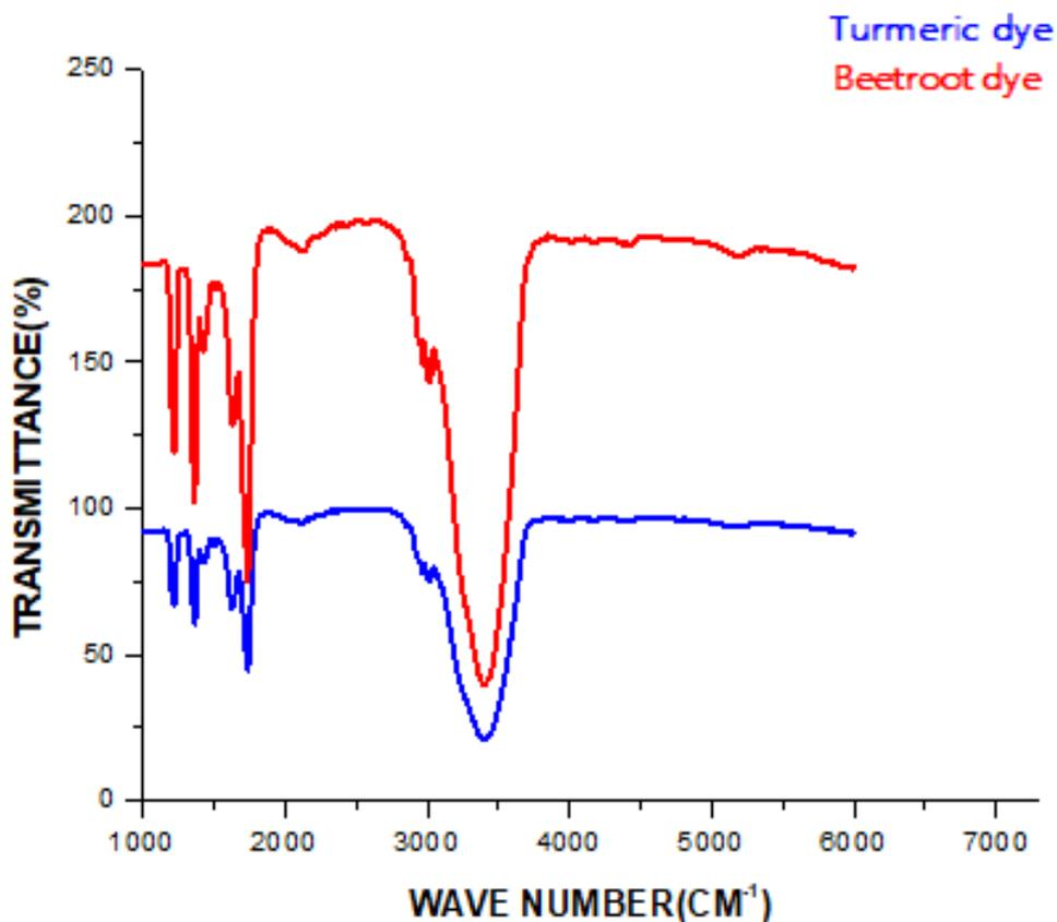
Figure 5. FTIR Spectra of Beetroot and Turmeric Dyes
