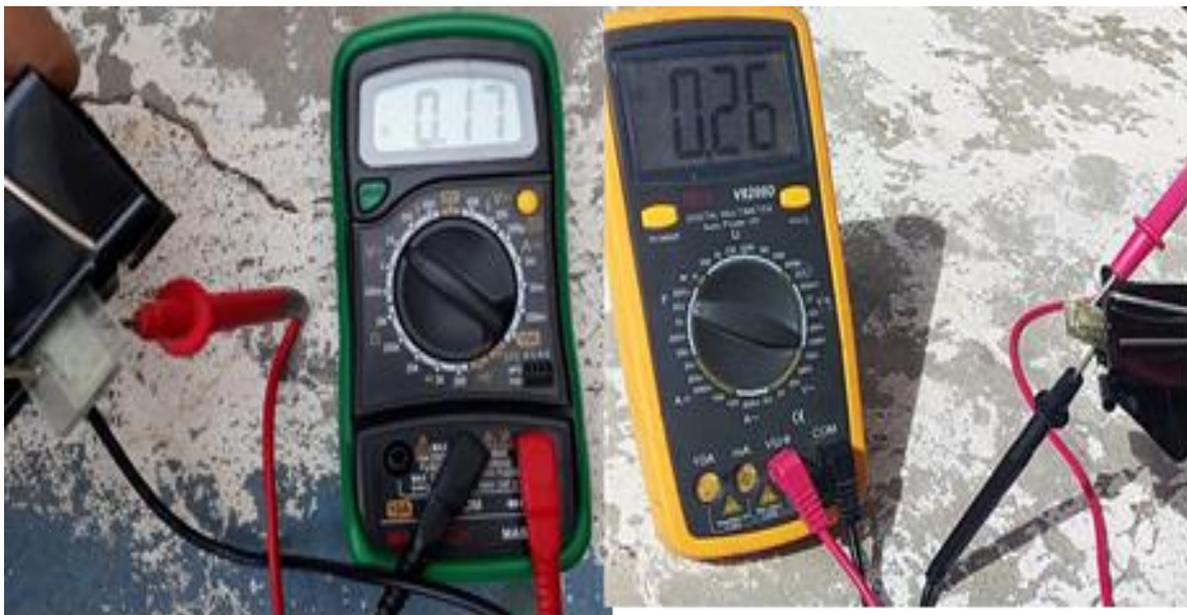
**Figure 3.** Voltage and Capacitance readings of carrot dye
