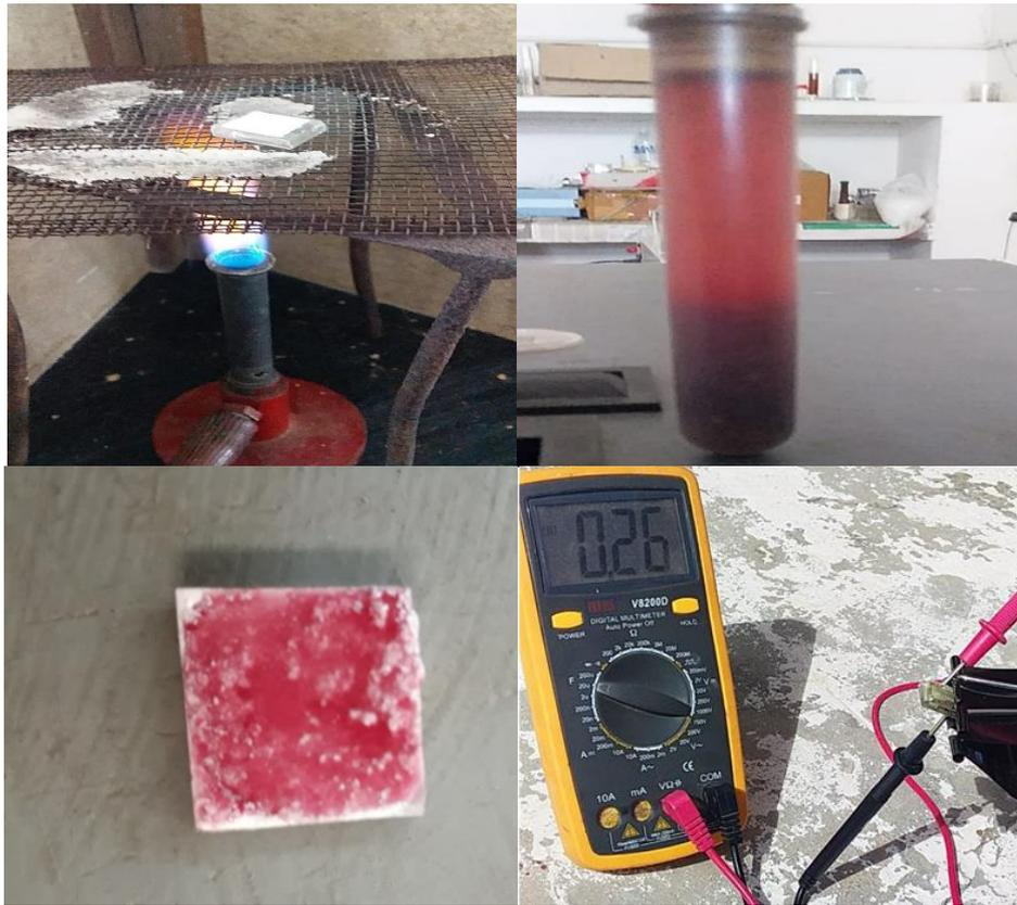
**Figure 2.** Photograph of Dye Sensitized Solar Cell Fabrication
