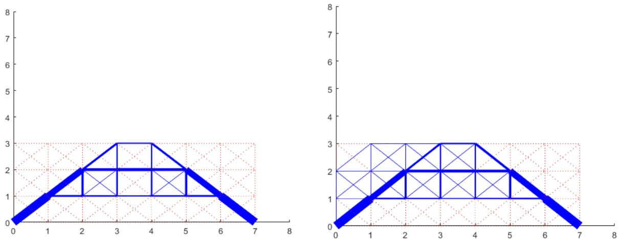
**Figure 5.** Results of Optimal Design for The First Case, Nominal (left) and Robust (right).
