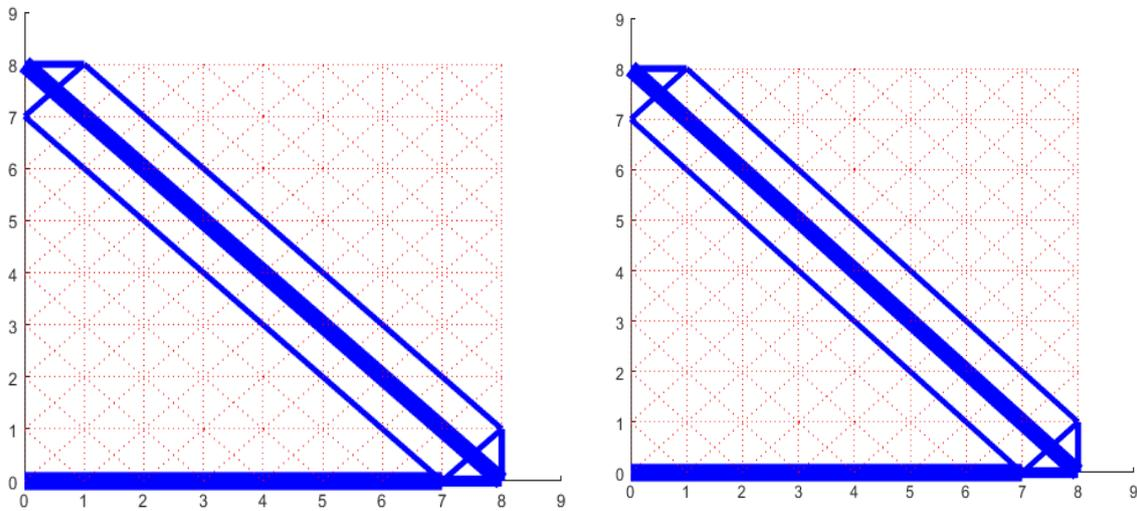
**Figure 3.** Results of Optimal Design for The First Case, Nominal (left) and Robust (right).
