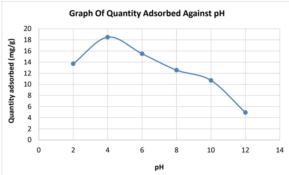
Figure 2. Graph of quantity adsorbed against pH
