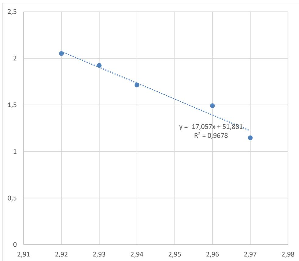
**Figure 6.** A plot of  $\ln q_e$  versus  $\ln C_e$
