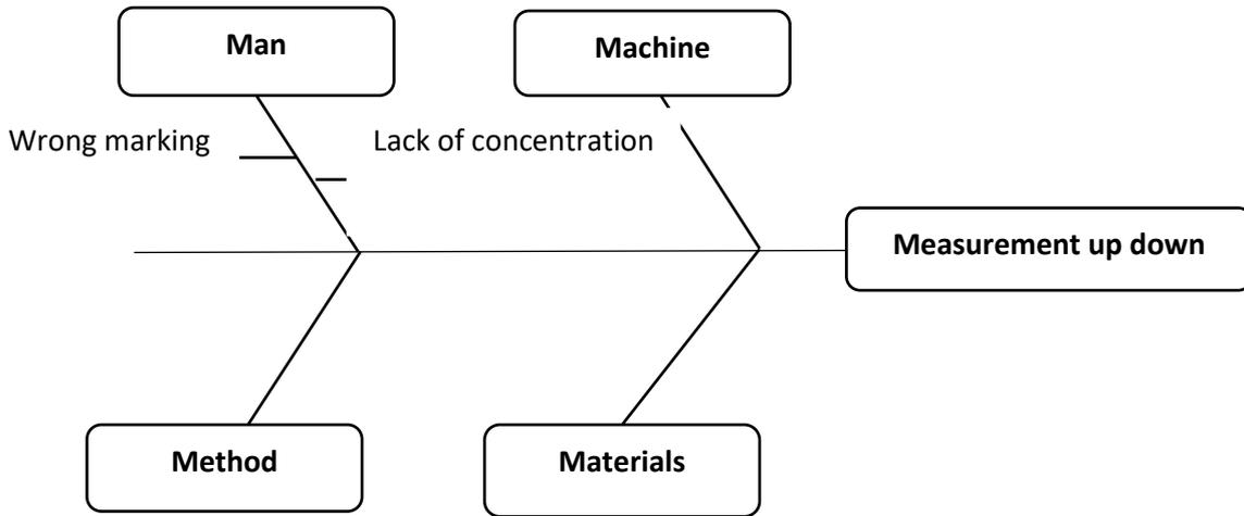
**Figure 9.** Cause effect diagram of Hand Brush placement up/down
