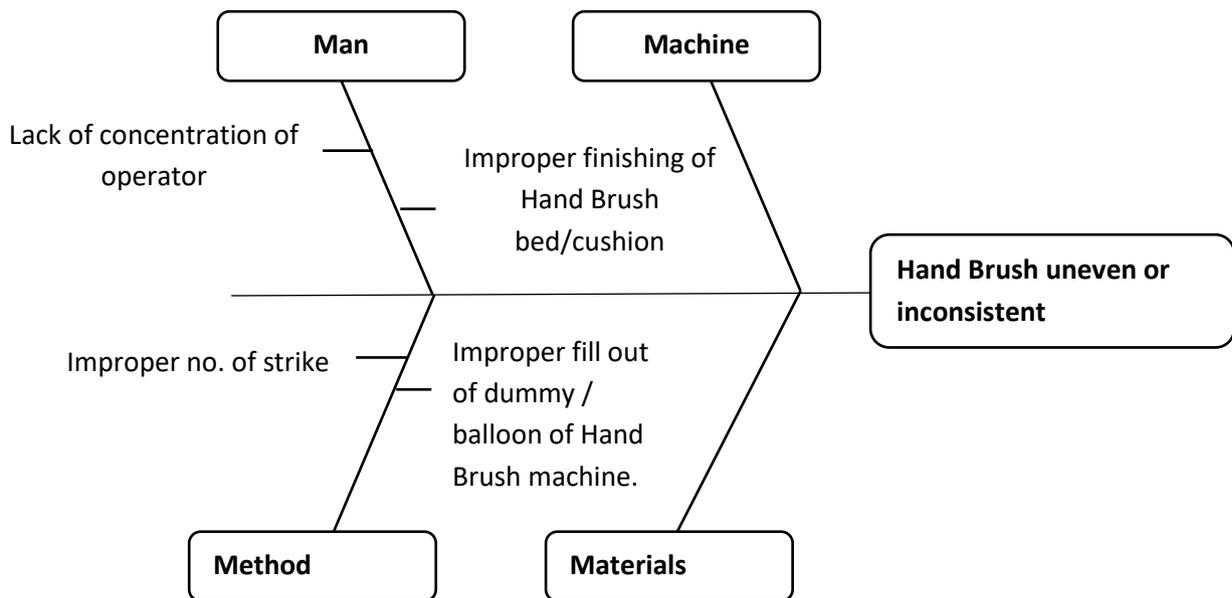
**Figure 8.** Cause-effect diagram of Hand Brush inconsistent
