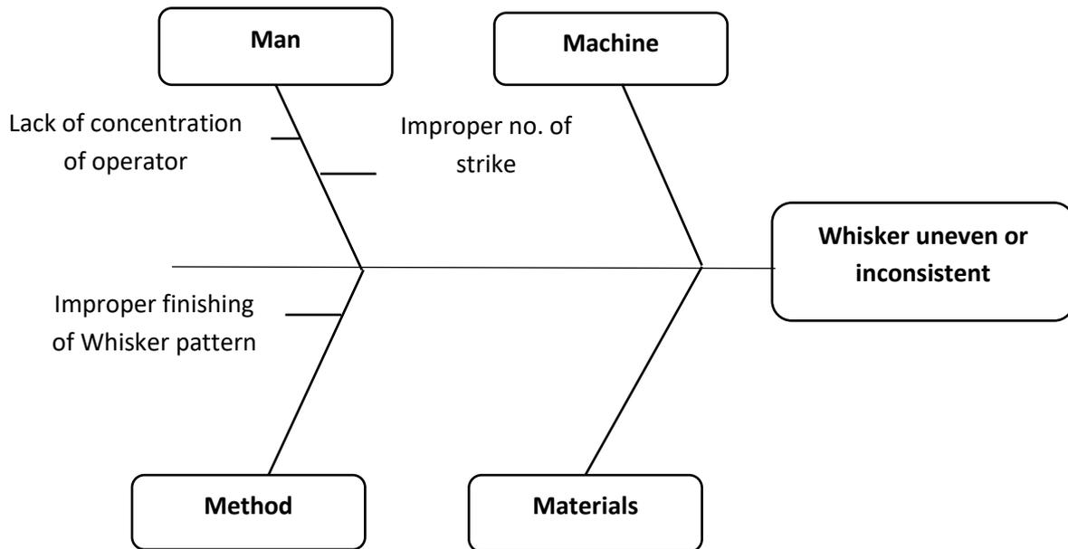
Figure 4. Cause-effect diagram of Whisker inconsistency
