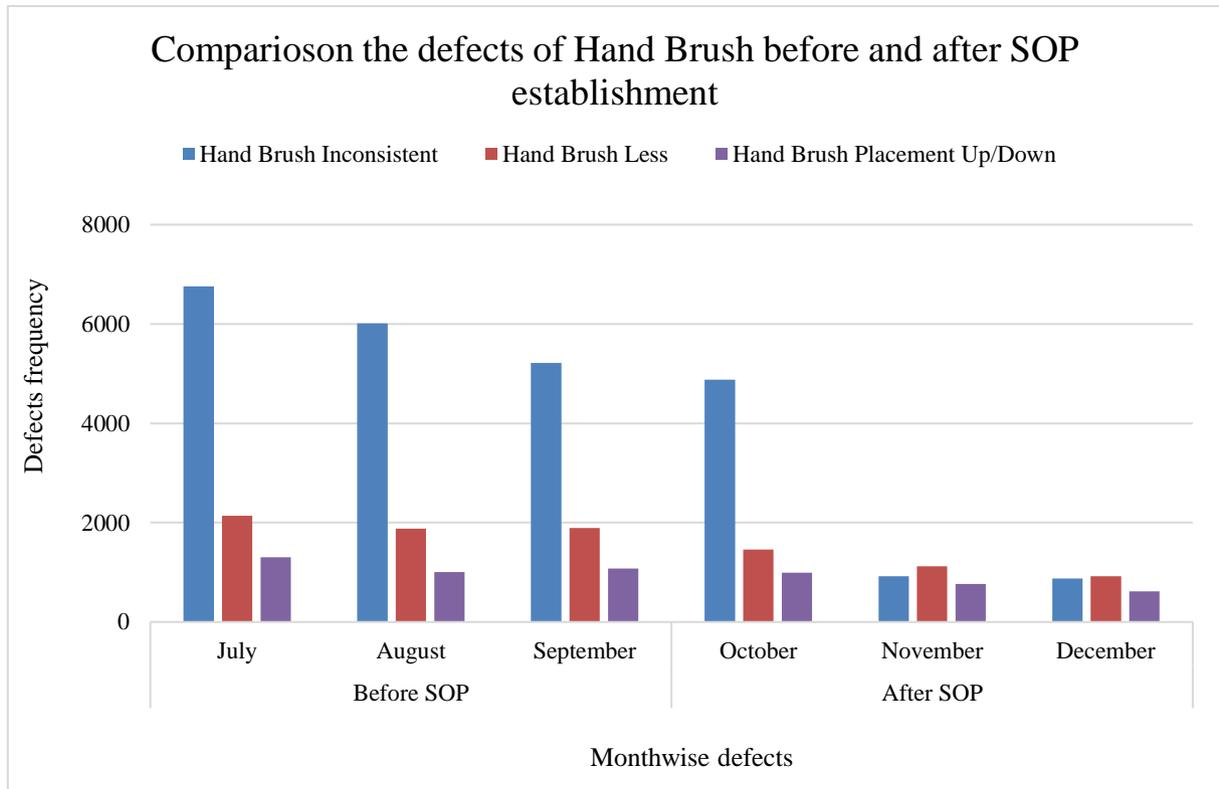
**Figure 12.** Comparing the defects of Hand Brush before and after SOP establishment
