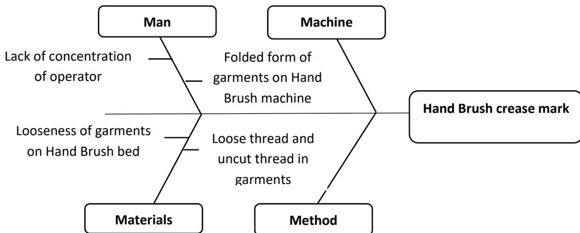
**Figure 10.** Cause-effect diagram of Hand Brush crease mark
