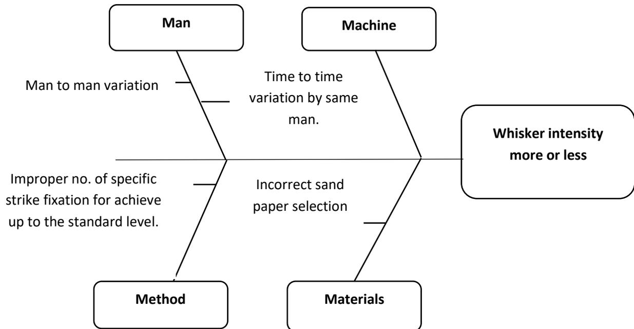
**Figure 5.** Cause-effect diagram of Whisker intensity more or less
