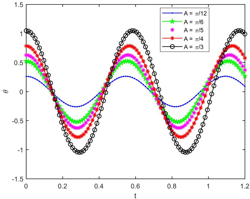
**Fig. 3.** Effect of amplitude on time responses of the system
