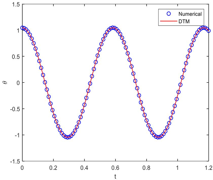
**Fig. 2b.** Time response of the system when  $A = \pi / 3$
