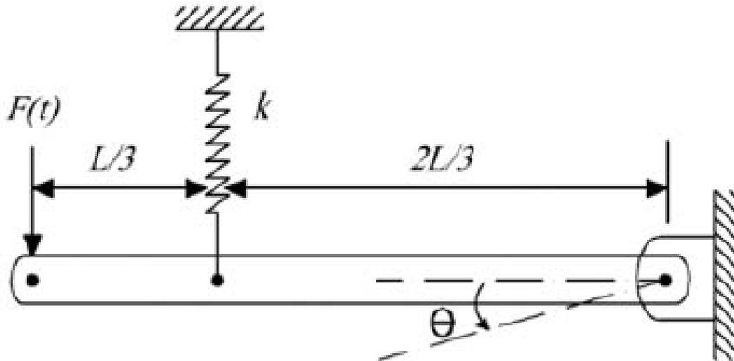
Fig. 1. The physical model of the oscillatory system
