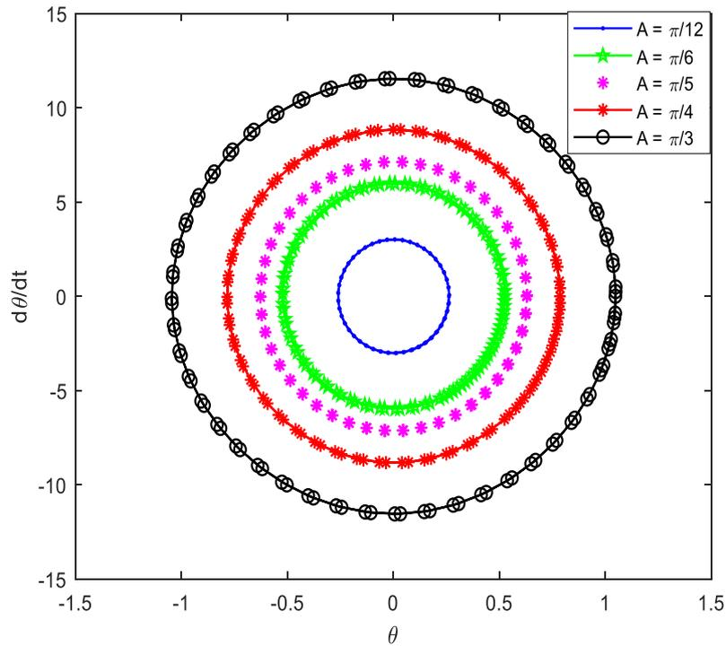
**Fig. 4.** Effect of amplitude on phase plots of the system
