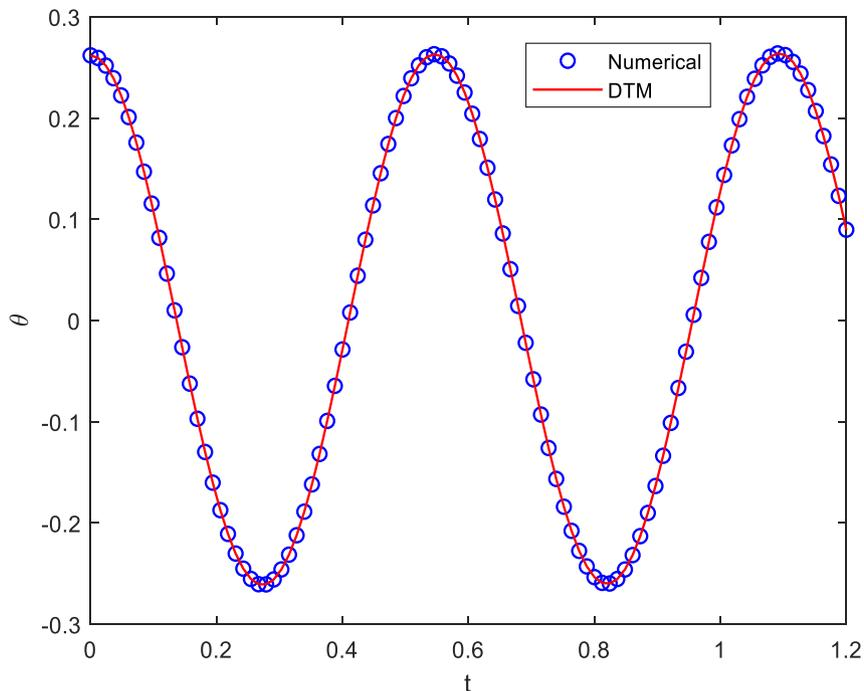
**Fig. 2a.** Time response of the system when  $A = \pi / 12$
