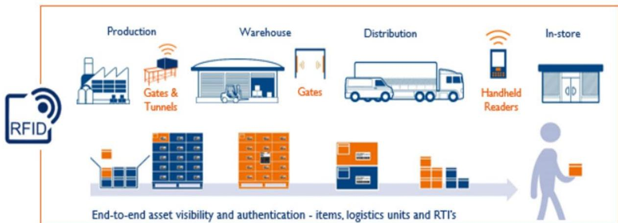
**Fig. 1.** RFID systems in supply chain management.
