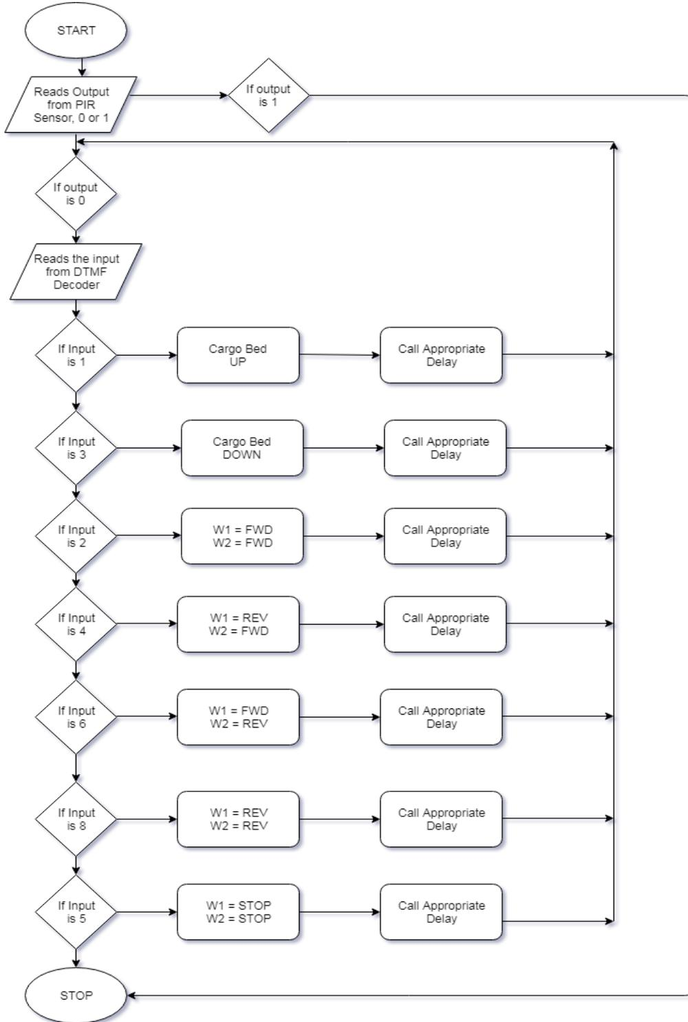
**Figure 8.** Operational Flowchart of the Guided Vehicle.
