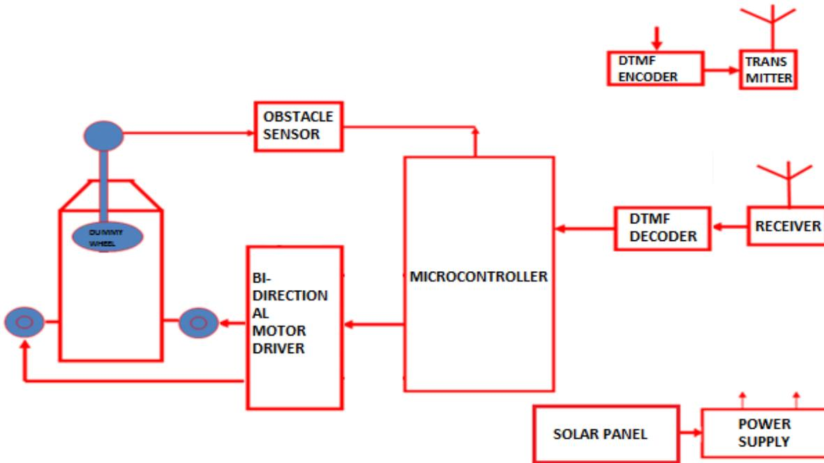
Figure 2. Block Diagram Representation.
