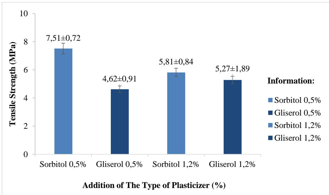
Figure 4. Edible Film Tensile Strength Chart
