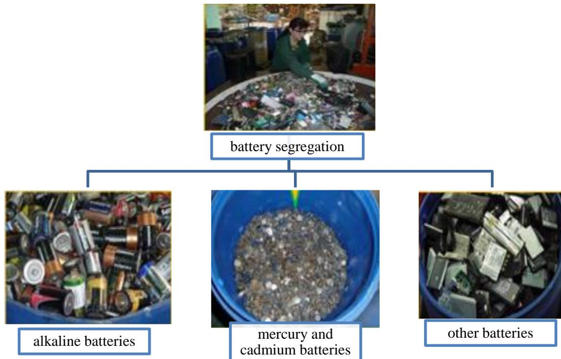
**Figure 1.** Battery segregation.
