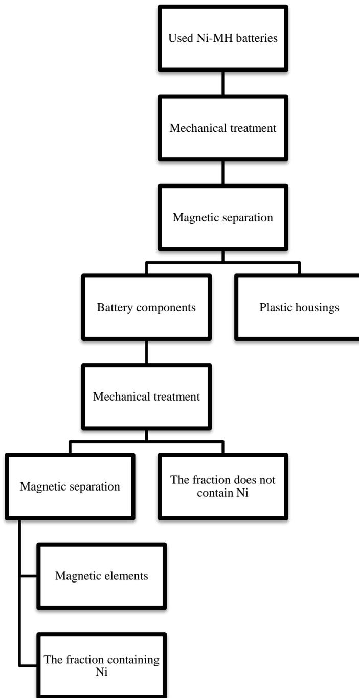
**Figure 3.** An example of a mechanical process for recovering a nickel-rich fraction from the Ni-MH battery stream.
