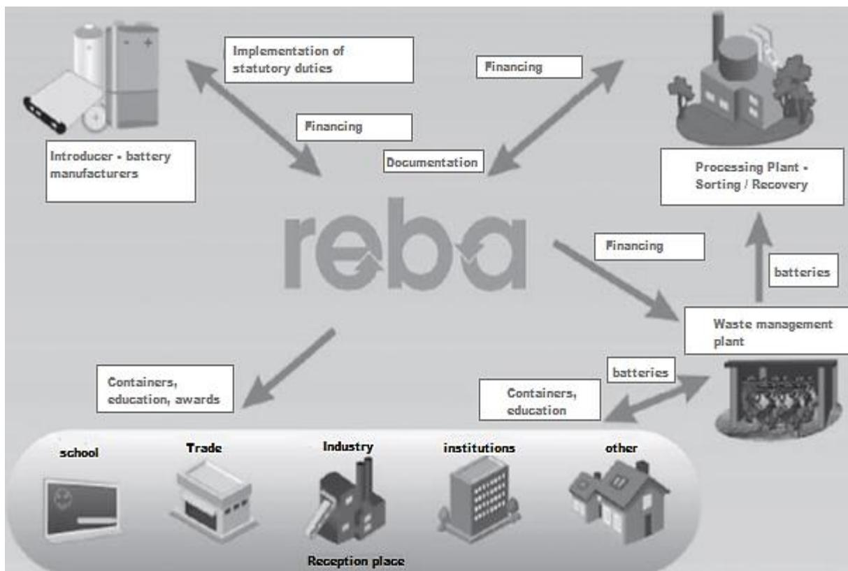
**Figure 4.** Diagram of the operation of the collection and processing system for portable batteries and accumulators promoted by Reba S.A.
