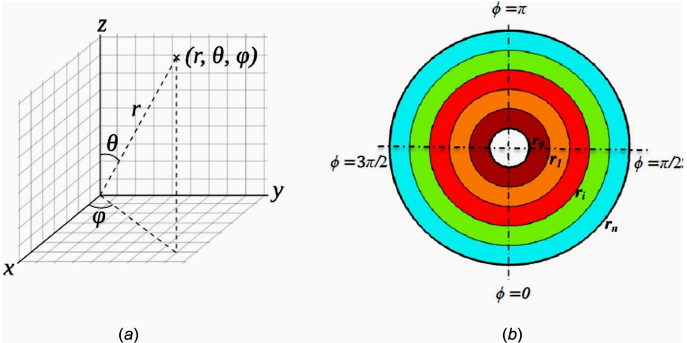
**Fig. 1.** (a) Coordinate system for the problem and (b) 2D cross-sectional view of n concentric spherical layers at 90-degree plane [25].
