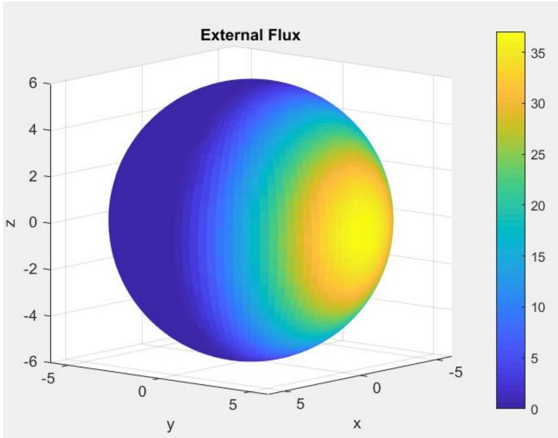
Fig. 3. External heat flux density plot of the sphere (3D).
