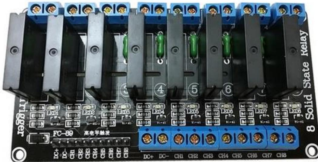
Fig. 3. Solid State Relays 8-channel Module
