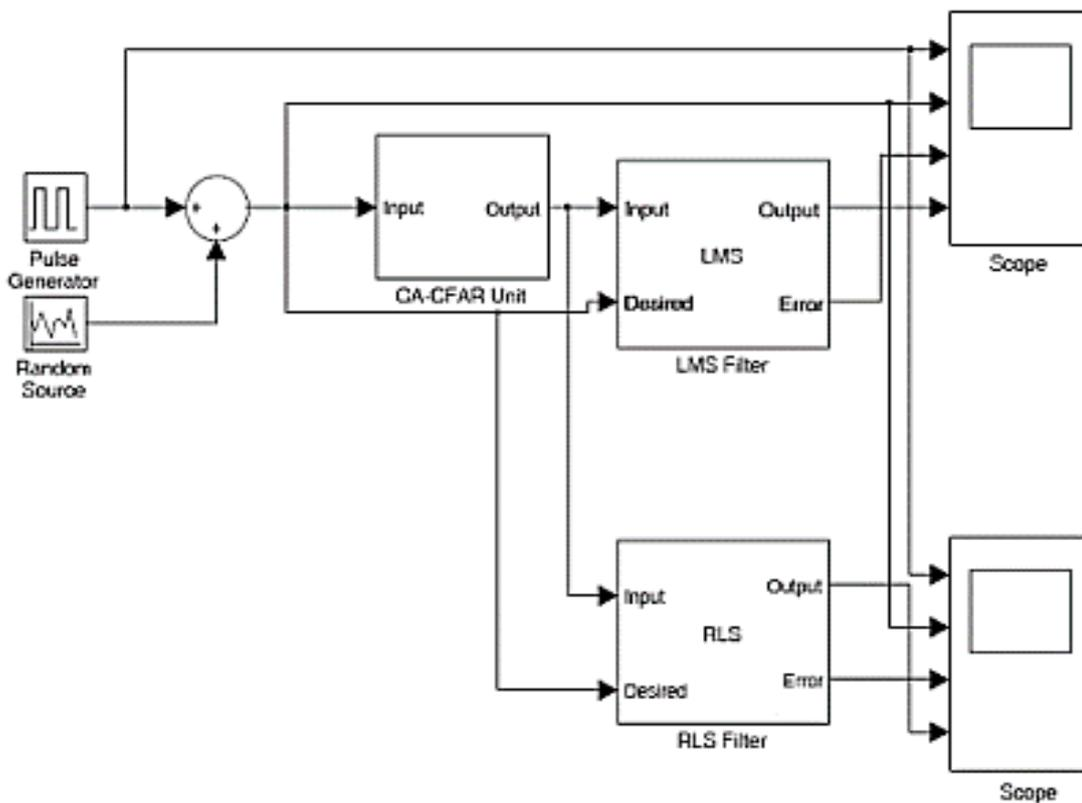
Figure 3. Simulink model of proposed system for the implementation of CA-CFAR fused technique.
