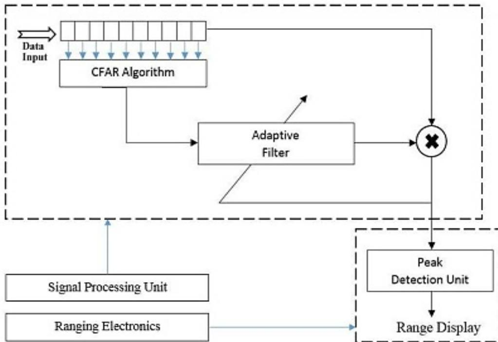
**Figure 2.** Proposed system showing fused CFAR and adaptive techniques.
