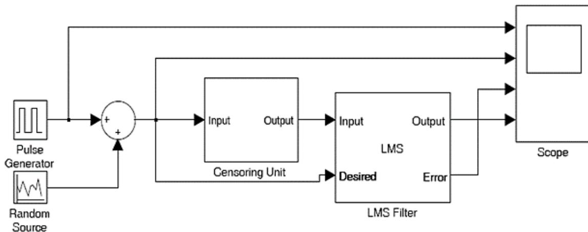
**Figure 4.** Simulink model of proposed system for the implementation of ACCA- CFAR technique.
