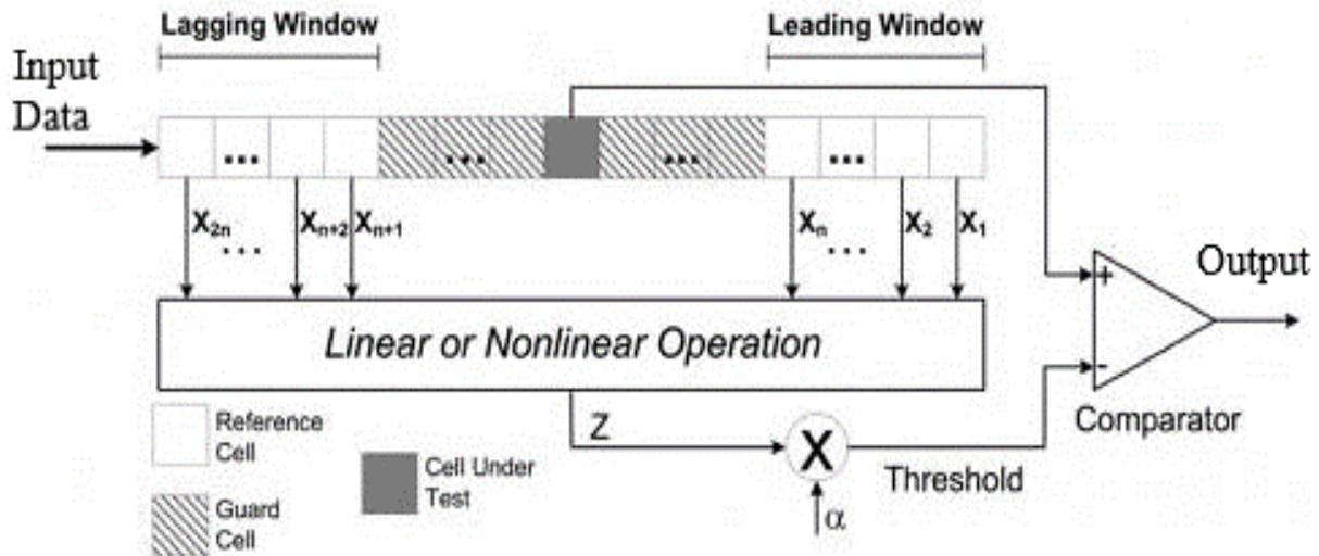
**Figure 1.** General block diagram of a generic range CFAR processor.
