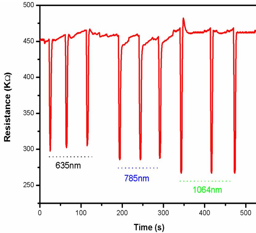
**Figure 1.** Variation of resistance with time for different wavelength of the laser beam.
