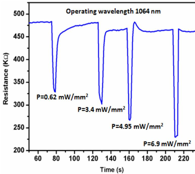
**Figure 2.** Variation of resistance with time for 1064 nm wavelength of the laser beam at varying power density
