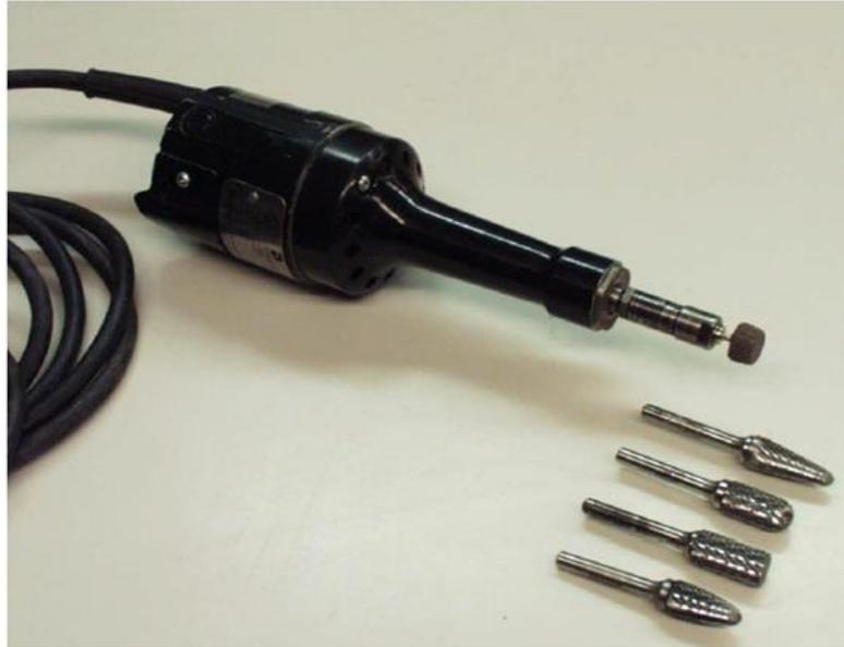
**Figure 4.** Typical Burr grinder [9].
