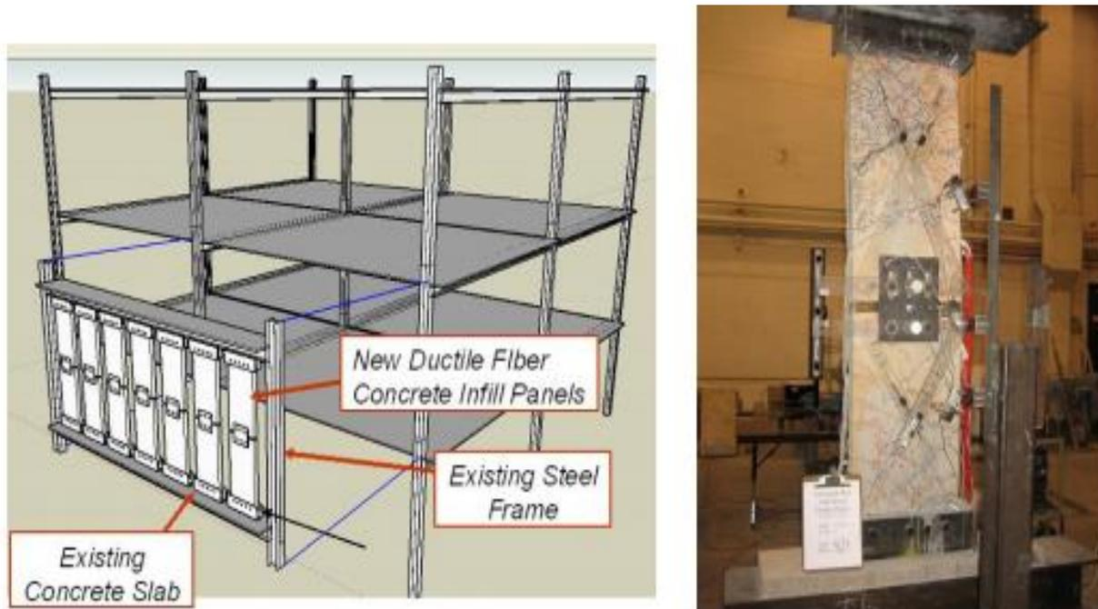
**Figure 8.** HPFRC infill retrofit system and double infill panel specimen after cyclic testing [11].
