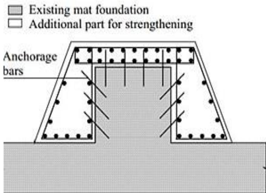
**Figure 9.** A schematic representation of mat foundation strengthening [17].
