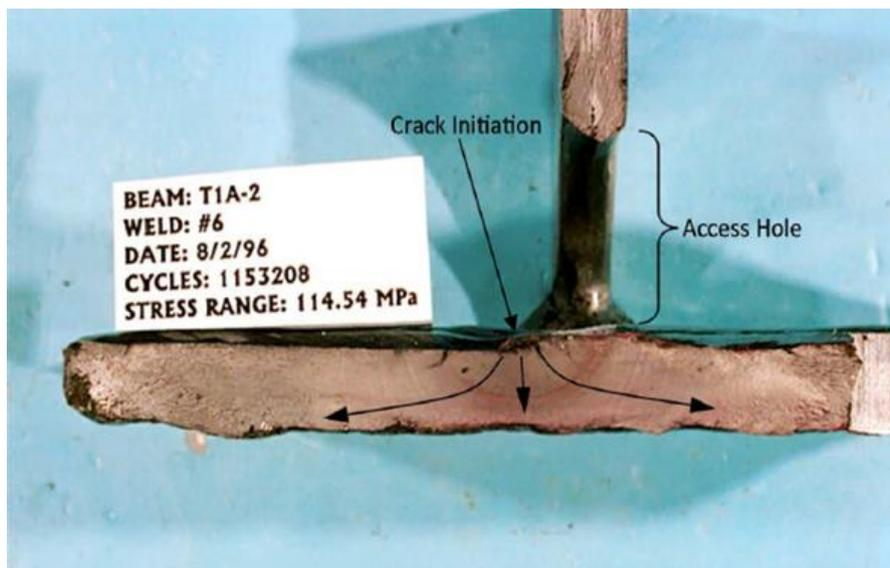
**Figure 1.** The fracture surface of an I-beam flange. Photo courtesy of US coast Guard [5].
