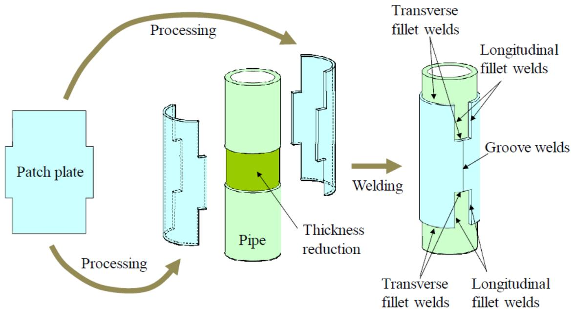
**Figure 7.** A general procedure of welding patch repair [10]
