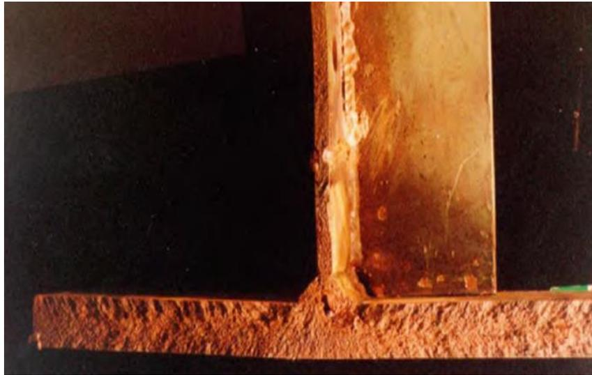
**Figure 2.** Girder flange fracture from Cherokee County, Iowa Bridge [6].
