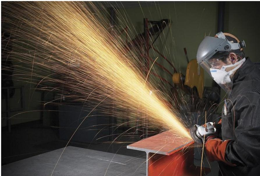
**Figure 3.** Disc grinding operation in steel beam (collected from Google images) [7].
