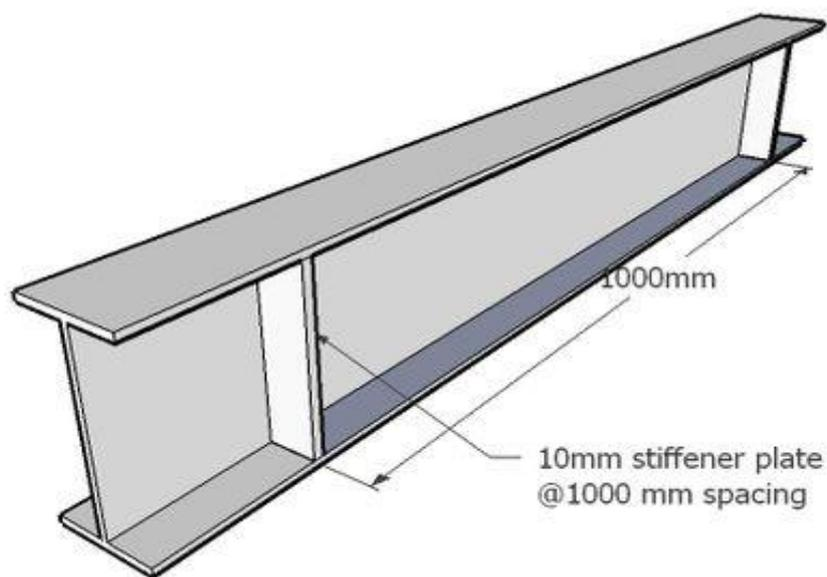
**Figure 11.** Details of using stiffener in steel beam or column [21].
