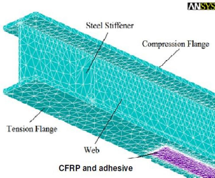
**Figure 10.** 3D simulated specimen [18].
