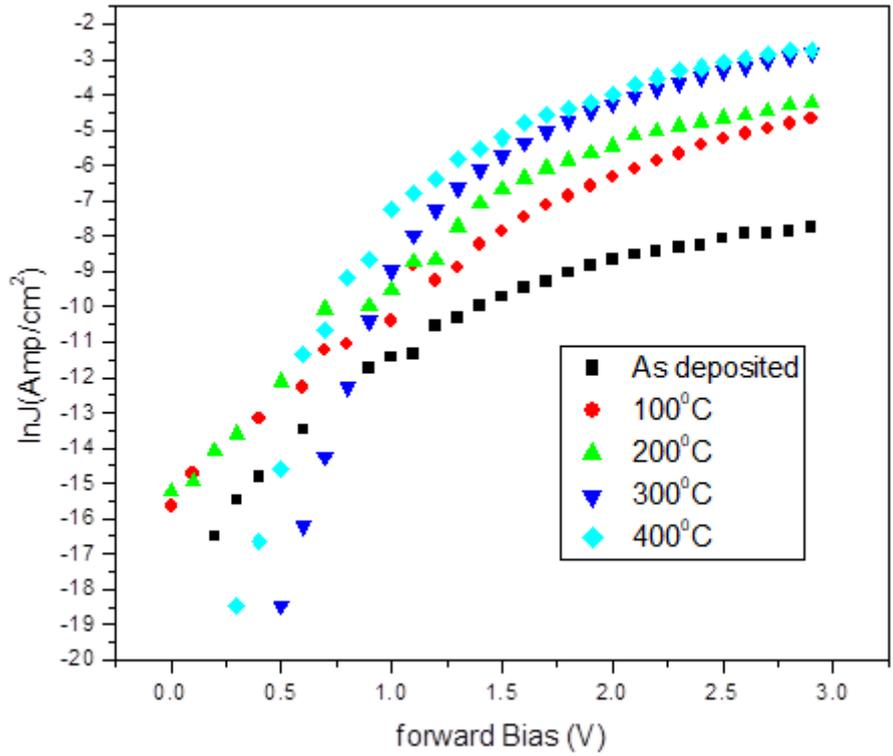
Figure 3. J-V characteristics of Nichrome Schottky diodes after different annealing temperature.
