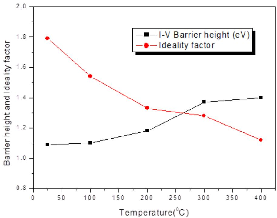
Figure 4. Dependence of I-V Barrier height and Ideality factor on Temperature.
