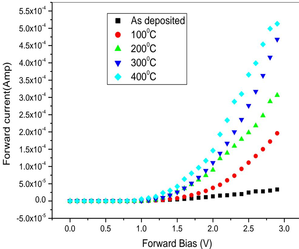
**Figure 2.** Forward I-V characteristics of Nichrome/4H-SiC Schottky diodes at deposited temperature and after annealing process.
