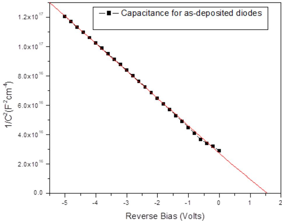
**Figure 5.**  $1/C^2$  vs. voltage plot of the Nichrome/4H-SiC diode.
