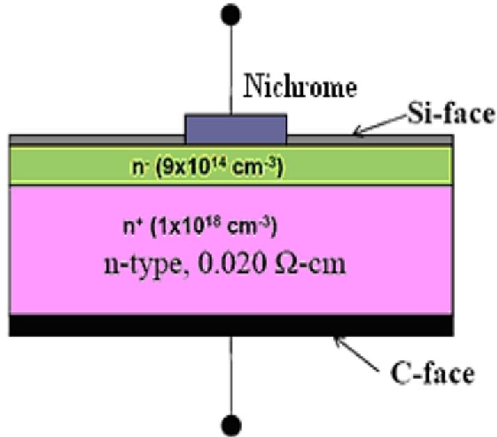
**Figure 1.** Schematic cross-sectional diagram of Schottky barrier diode.
