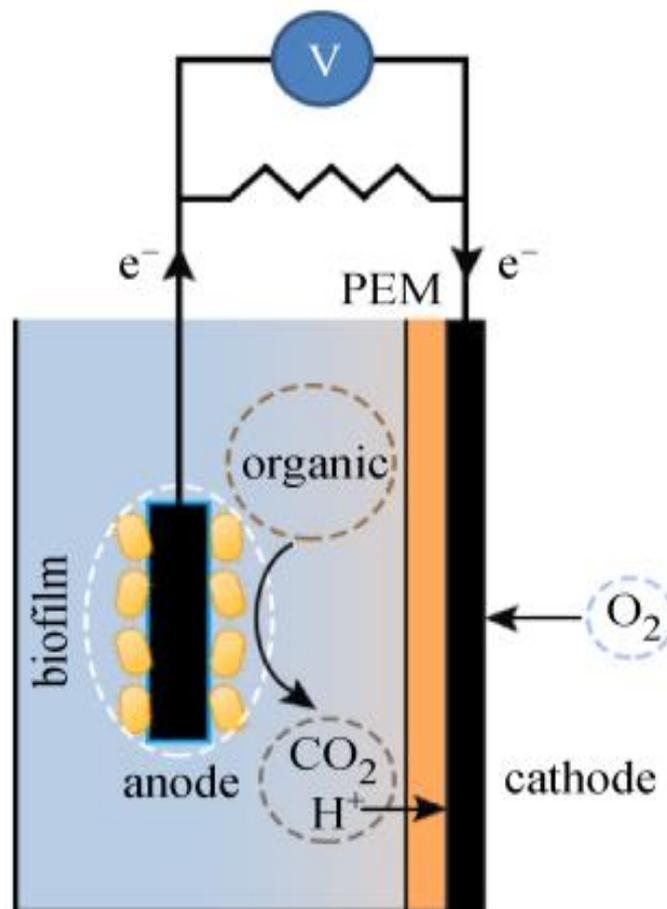
**Figure 3.** Schematic representation of a single-chamber MFC [18]
