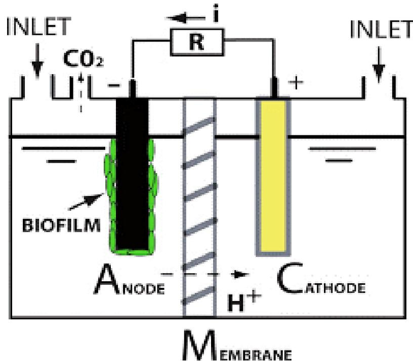
**Figure 4.** Schematic representation of a dual-chambered MFC [18]
