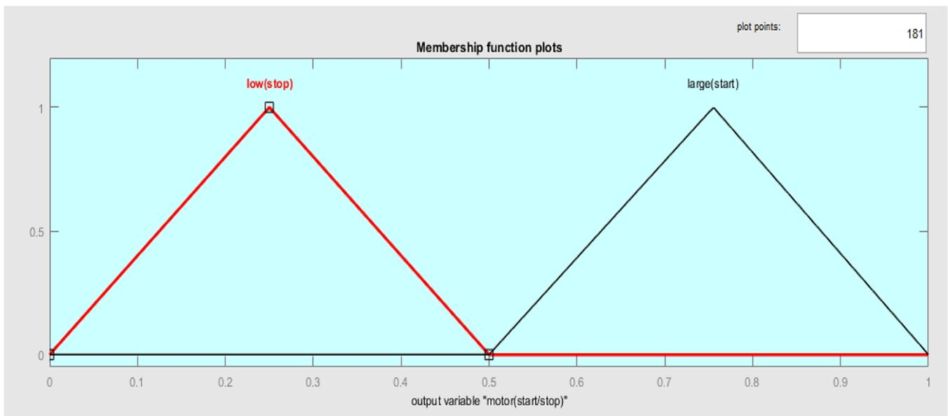
**Figure 11.** Output variable “Motor (Start/Stop)”
