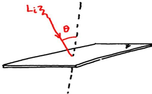
**Figure 6.** Incident insolation at an angle at solar panel due to its tilt
