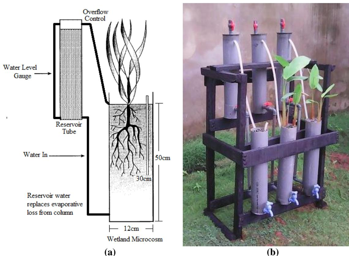
**Figure 1.** (a) Schematic diagram of column design and water delivery system (Adapted from Allen et al., 2002), (b) Experimental setup
