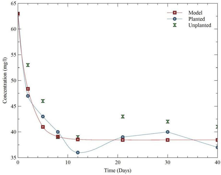
Figure 4. Measured and calibrated  $\text{NH}_4\text{-N}$  dynamics in the HSSF CW column.
