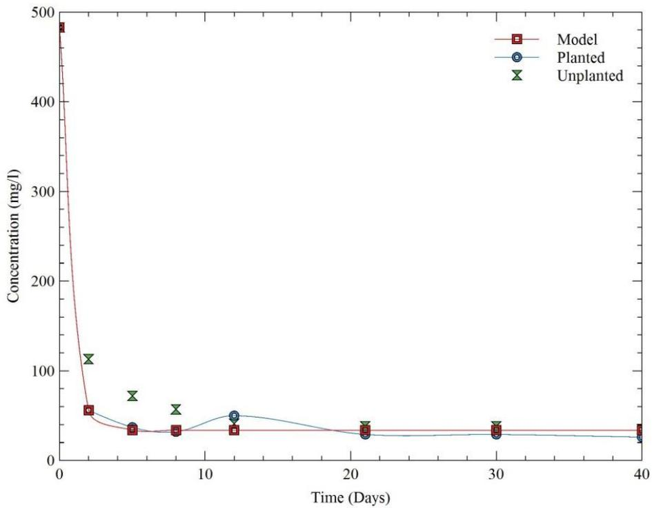
Figure 3. Measured and calibrated TSS dynamics in the HSSF-CW column.
