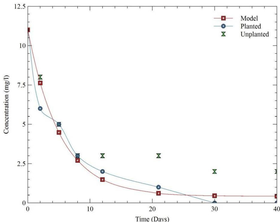
**Figure 6.** Measured and calibrated  $\text{PO}_4^{3-}$  dynamics in the HSSF CW column.
