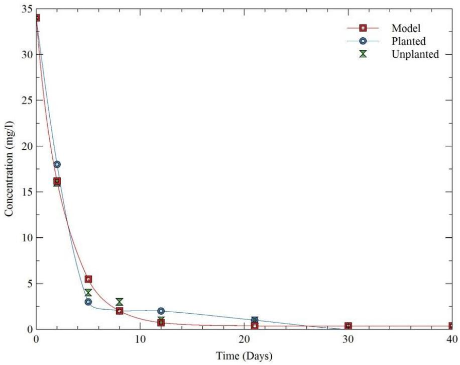
Figure 5. Measured and calibrated  $\text{NO}_3\text{-N}$  dynamics in the HSSF CW column.
