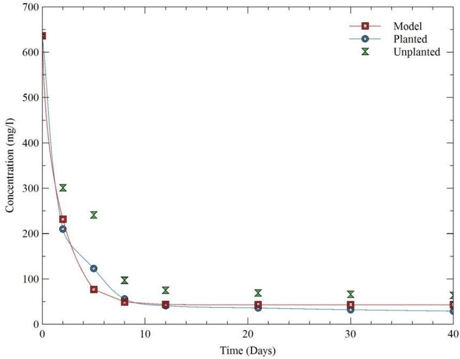
Figure 2. Measured and calibrated BOD dynamics in the HSSF-CW column.
