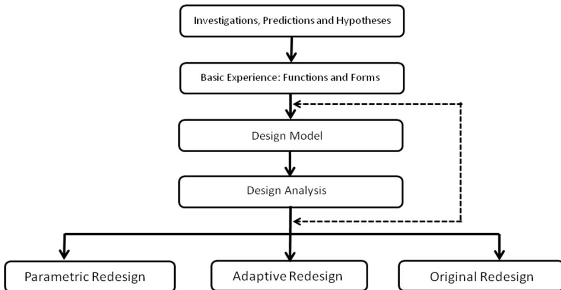
**Figure 1.** The Framework of reverse engineering and redesign methodology
