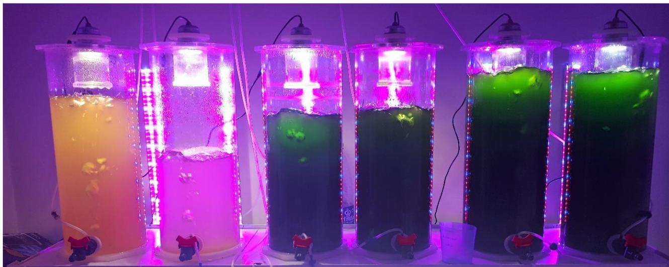
**Picture 1.** Photobioreactors in Laboratory of Marine Organisms Reproduction in West Pomeranian University of Technology in Szczecin, Poland
