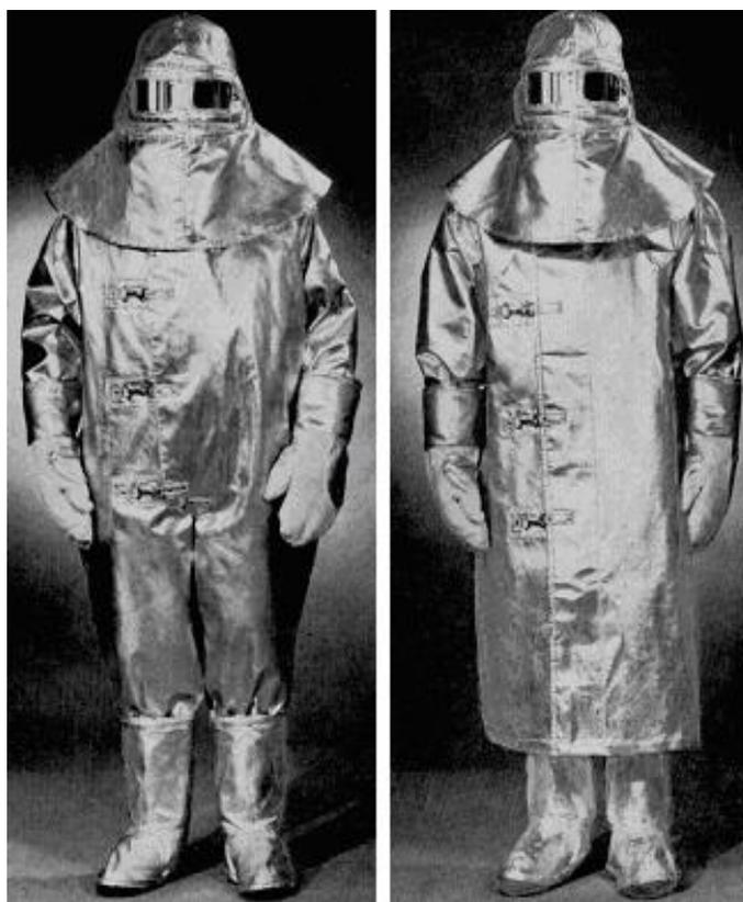
**Fig. 5.** Protective clothing against splashes of molten metal [17]
