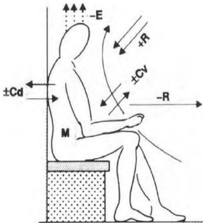
**Fig. 1.** Heat exchanges of the human body [8]
