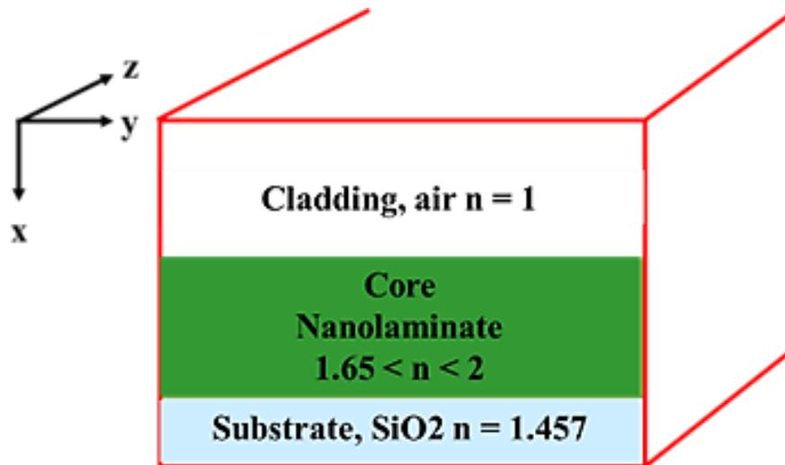
Figure 3. Structure of a slab optical waveguide.
