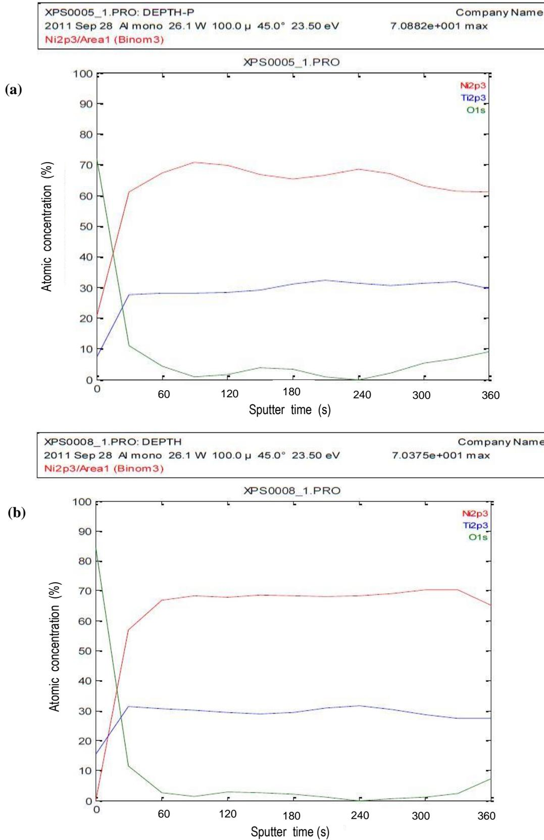
Fig. 3. XPS depth profiles of: (a) EP Nitinol surface, and (b) MEP Nitinol surface
