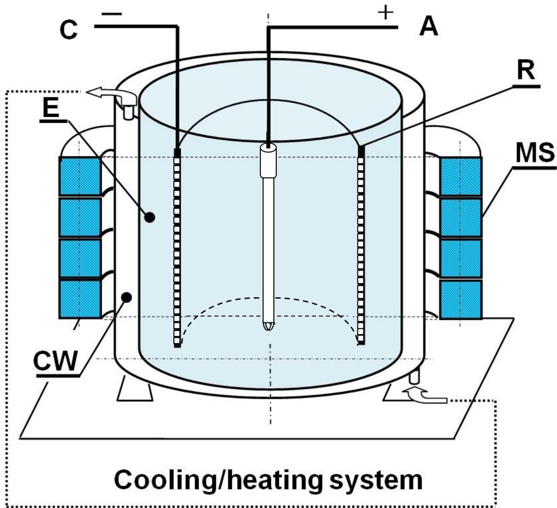
**Fig. 1.** Schematic view of the set-up used for magneto-electropolishing MEP with the sample-Nitinol needle connected to anode A: C – cathode connection, R – cylindrical perforated cathode, MS – magnetic rings, E – electrolyte, CW – cooling water
