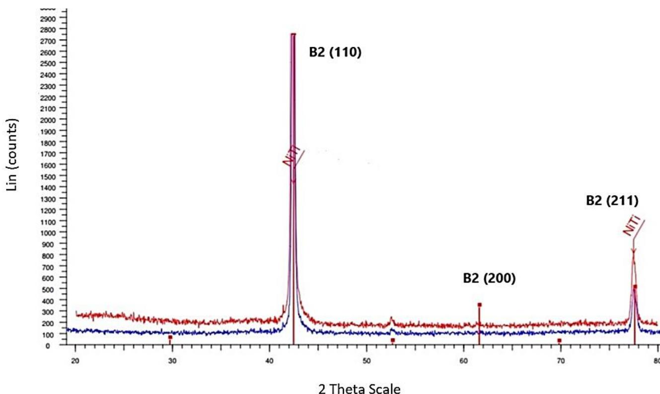
**Fig. 5.** XRD analysis of austenitic Nitinol after EP (blue\_lower) and MEP (red\_higher)
