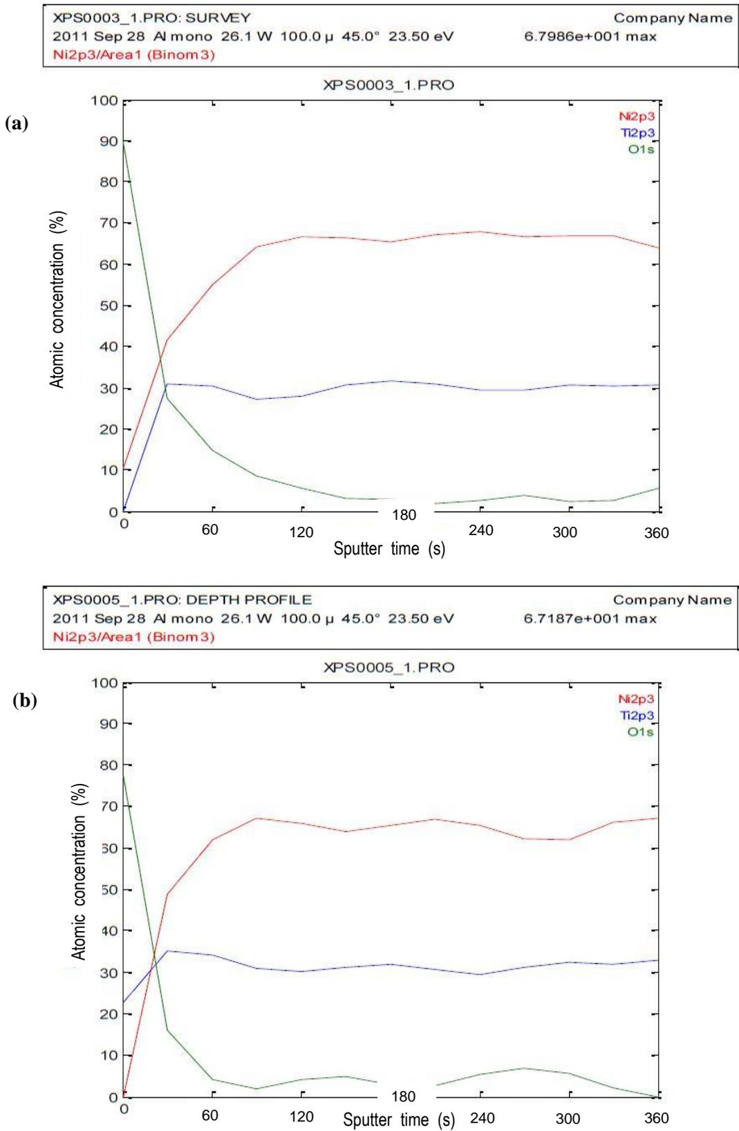
**Fig. 4.** XPS depth profiles of: (a) EP + 6% NaClO Nitinol surface, and (b) MEP + 6% NaClO Nitinol surface
