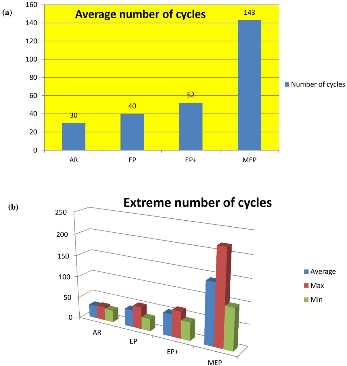
**Fig. 6.** Number of bending cycles of Nitinol needle until fracture: (a) average, (b) extreme values (for 1 push/pull bending cycle, see Fig. 2)
