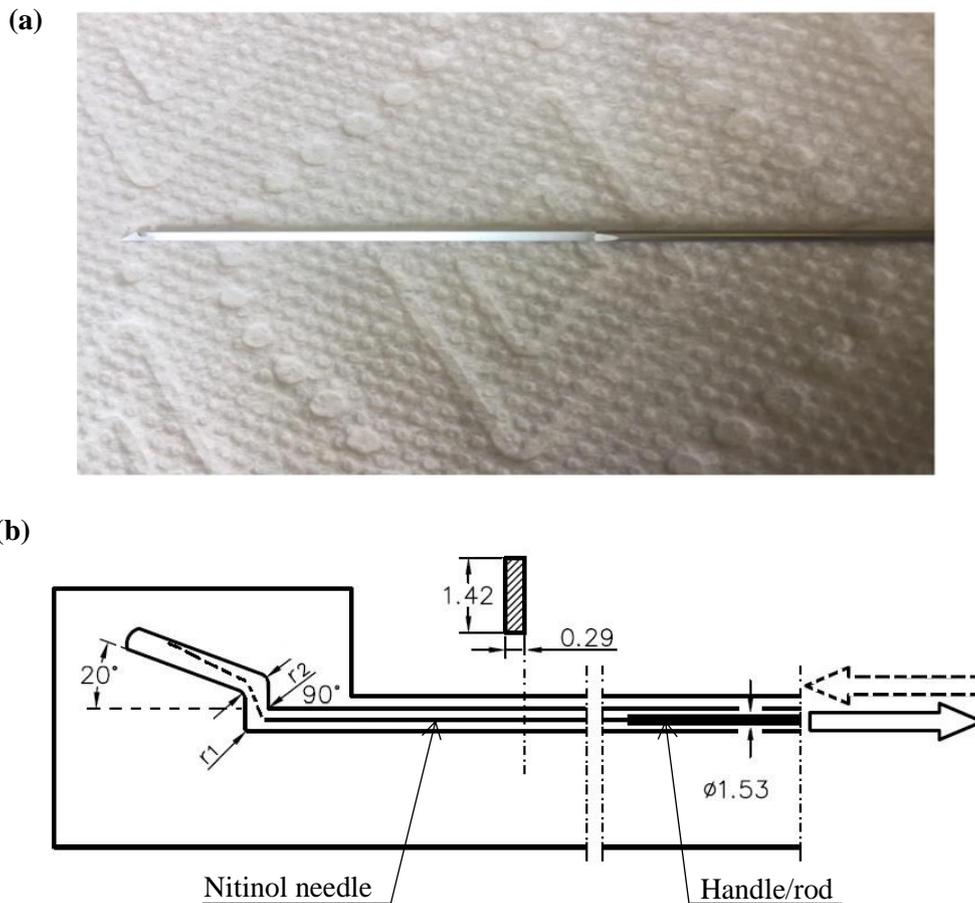
**Fig. 2.** Nitinol needle (a) and the scheme of test site for the needle fatigue testing (b): view from above
