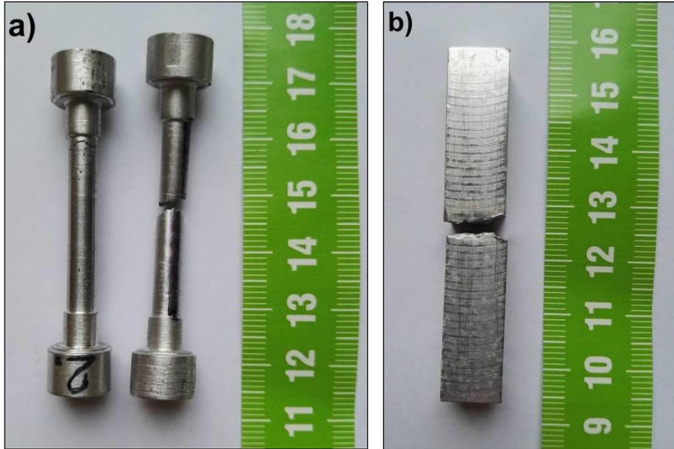
**Fig. 6.** Samples prepared for mechanical properties tests: **a)** tensile test; **b)** Charpy impact test.
