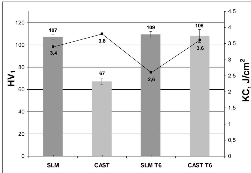
**Fig. 7.** Comparison of hardness and impact energy of AlSi10Mg alloy obtained by casting and SLM method.
