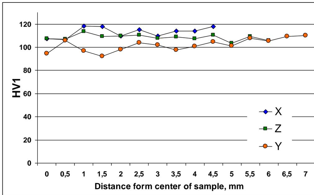
**Figure 4.** Hardness distribution for AlSi10Mg alloy obtained by SLM method depending on building direction.
