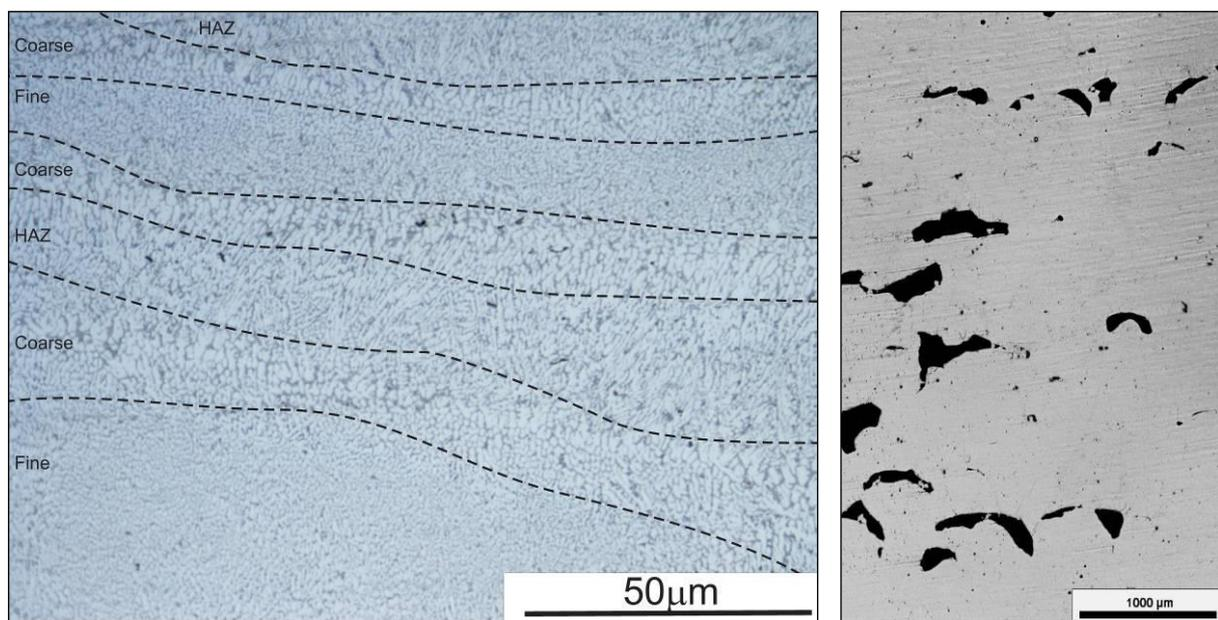
**Figure 2.** a) Microstructure of as-built SLM AlSi10Mg alloy; b) porosity in mounted cross-section of SLM sample.
