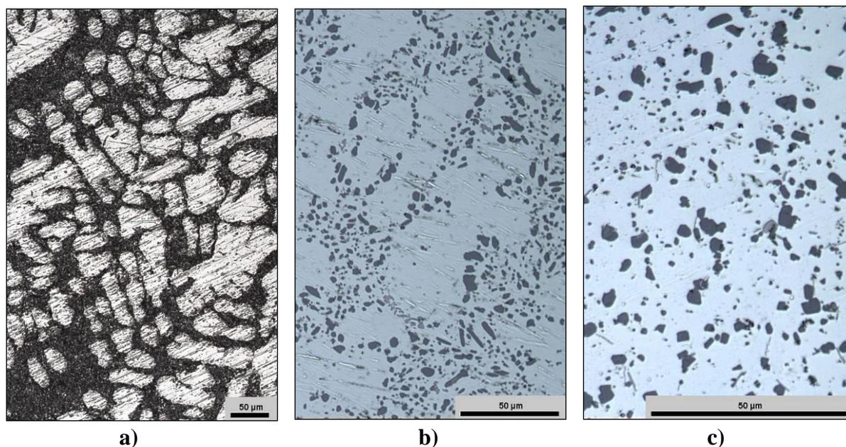
**Figure 3.** a) Microstructure of cast AlSi10Mg alloy in as-delivered condition – etched; b) T6 heat treated cast AlSi10Mg alloy; c) T6 heat treated SLM AlSi10Mg alloy.
