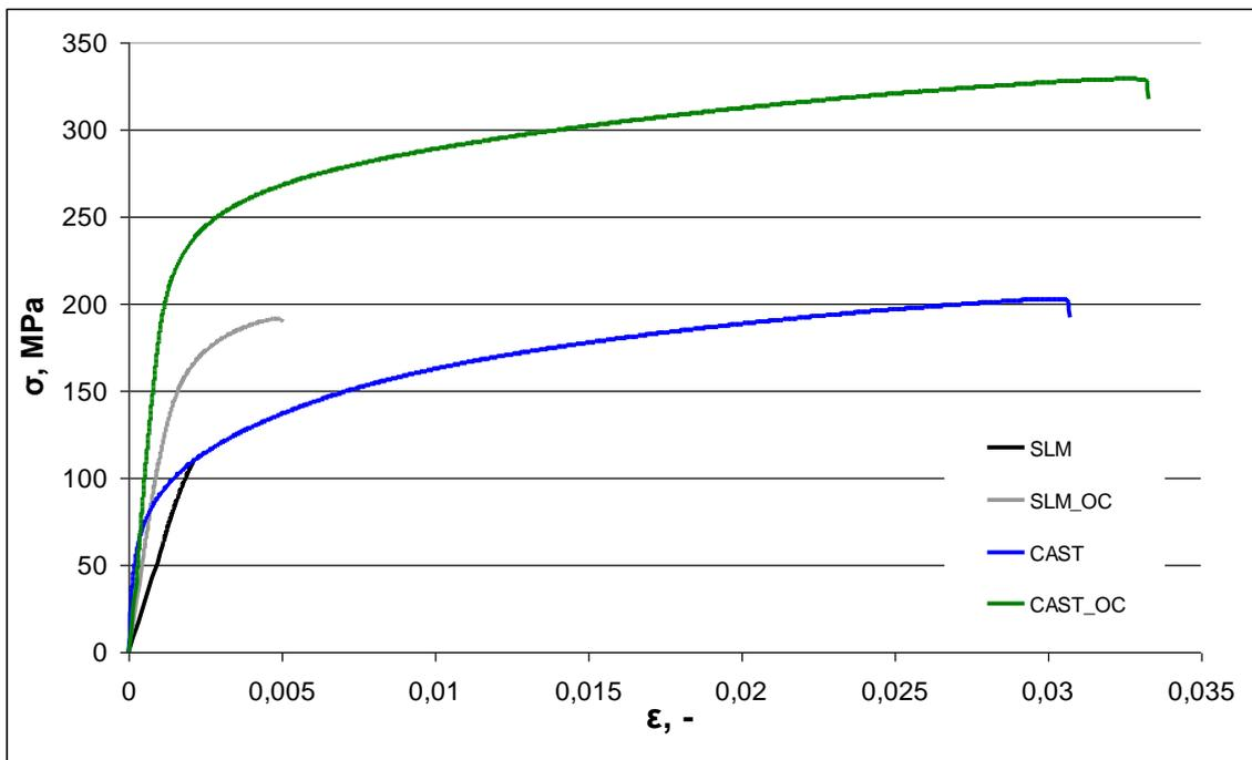
**Fig. 5.** Stress-strain curves for SLM and cast AlSi10Mg alloy in as-delivered condition and after T6 heat treatment.
