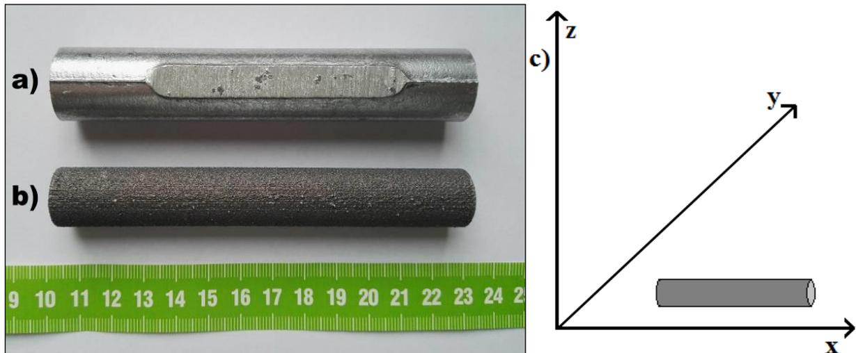
**Figure 1.** As-delivered AlSi10Mg billets: a) casting, b) sintered; c) schematic representation of building directions.
