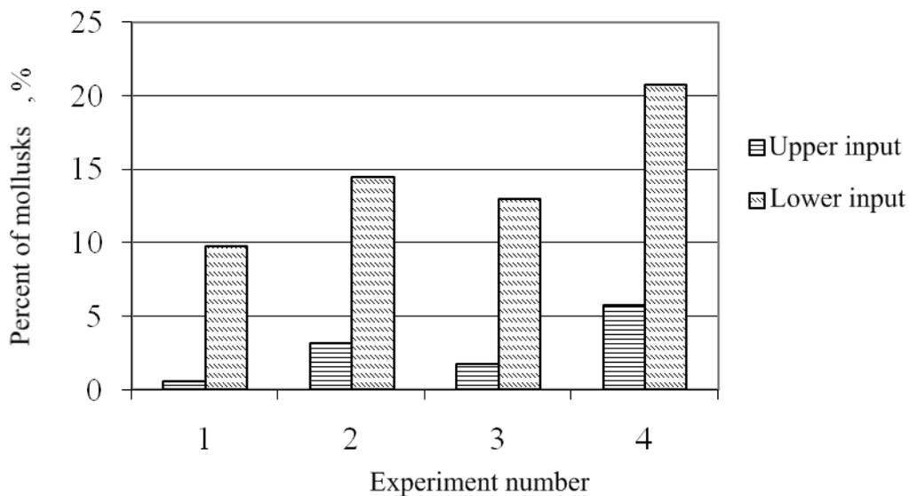
**Figure 7.** Efficiency of traps with different inlets.
