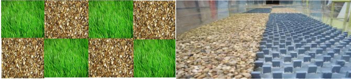
Figure 1. Bed Roughness Configuration Plan View of Roughness Patches for Experiment One and Two
