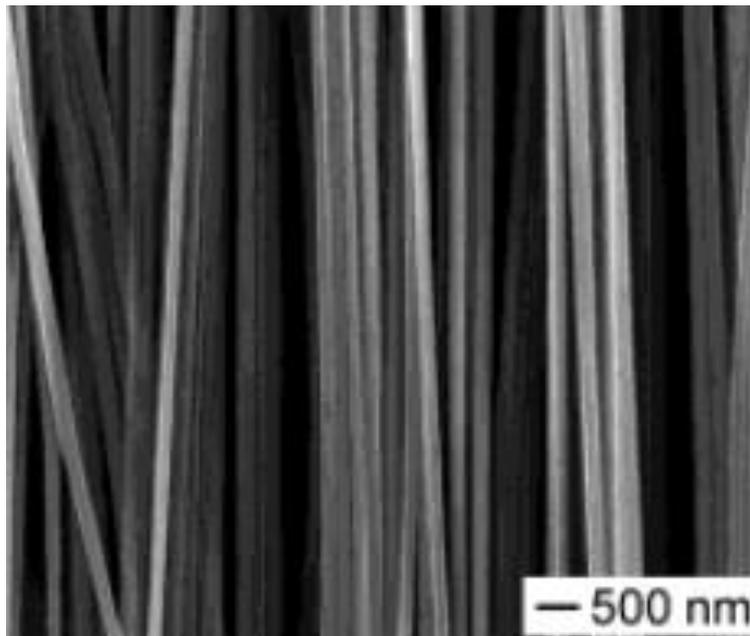
**Figure 1.** SEM image of carbon nanofibers [4]
