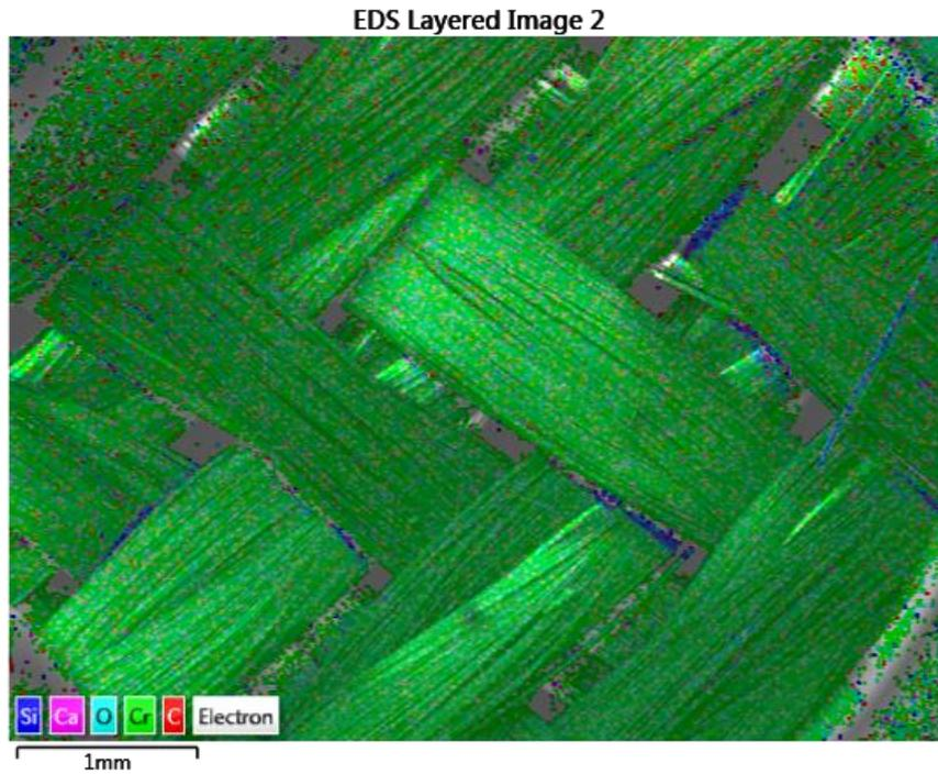
**Figure 6.** A chromium-plated coating with a thickness of 5  $\mu\text{m}$  embedded on the surface of the basalt fabric -SEM
