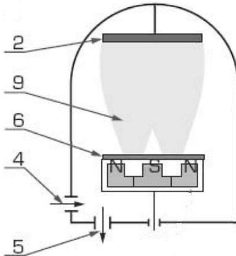
**Figure 3.** Scheme of magnetron sputtering [15]
