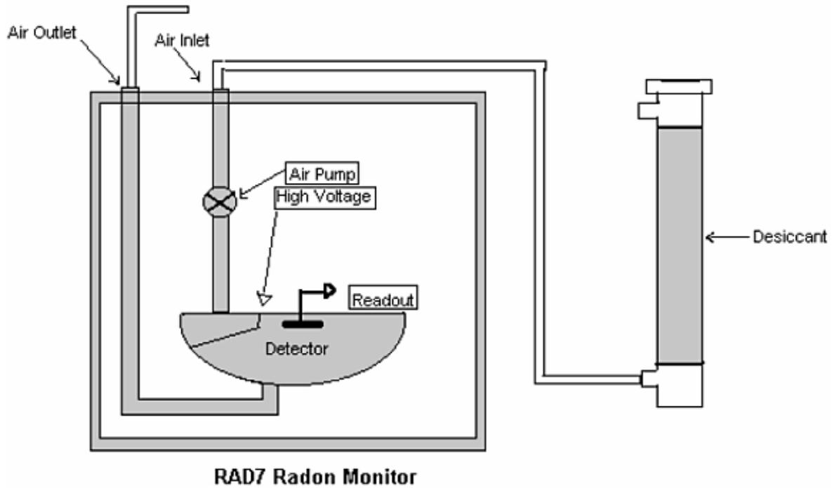
**Figure 1.** Schematic of the RAD-7. Special emphasis is put on the hemispherical shaped periodic-fill cell, the high voltage power supply inside the detector as well as the air pump that samples the air to be analyzed.
