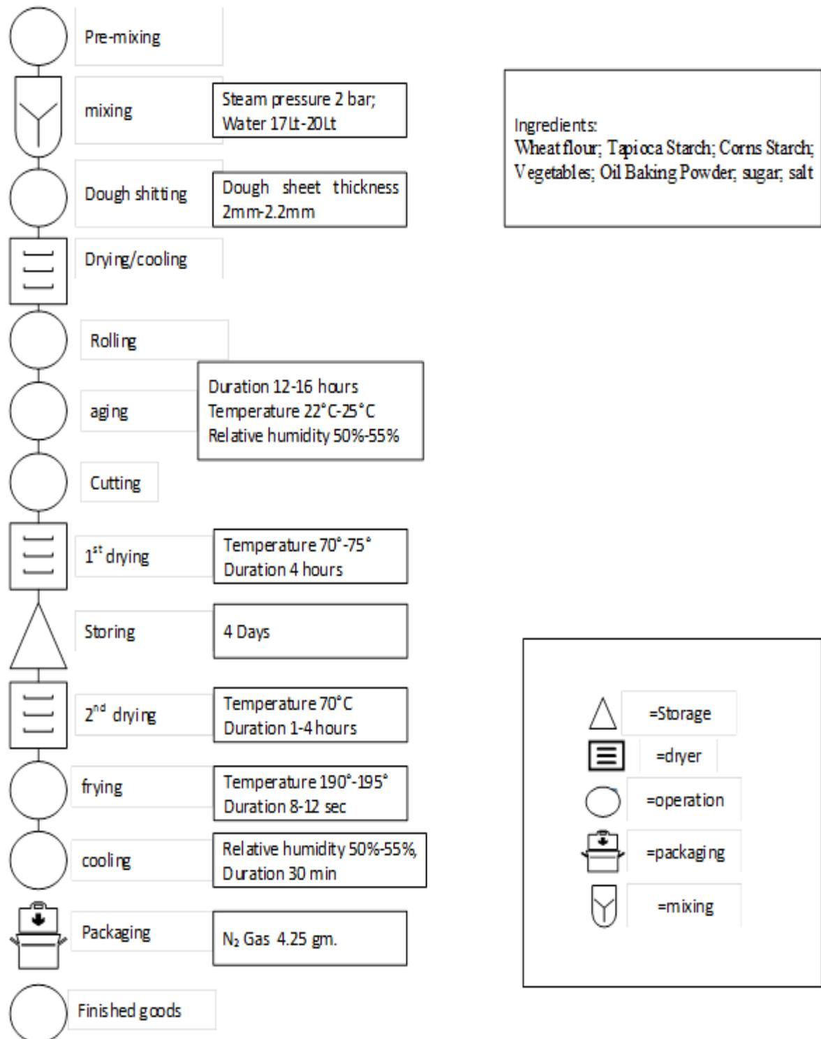
**Figure 4.** Process flow chart for ‘French Fry chips’ manufacturing.
