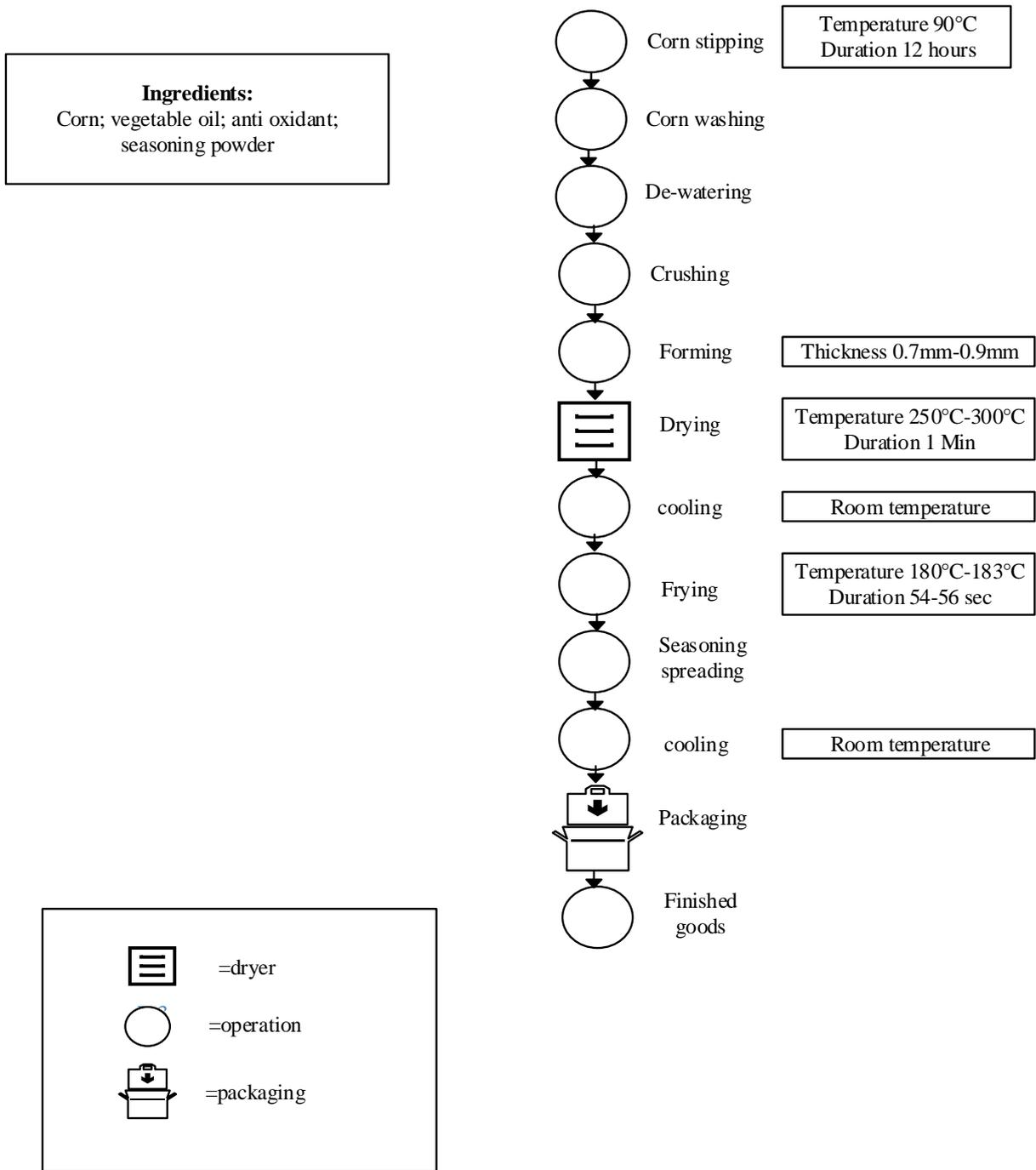
**Figure 7.** Process flow chart for 'Chicken Wing chips' manufacturing.
