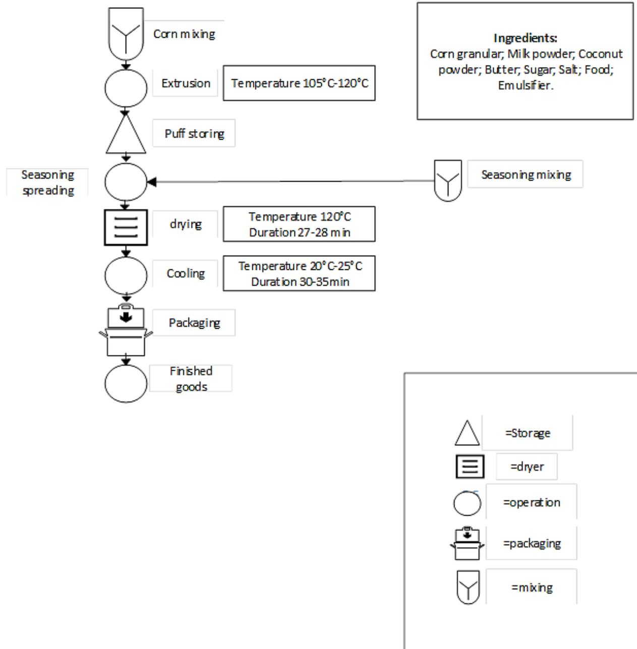
**Figure 5.** Process flow chart for ‘Coconut Crunch’ manufacturing.
