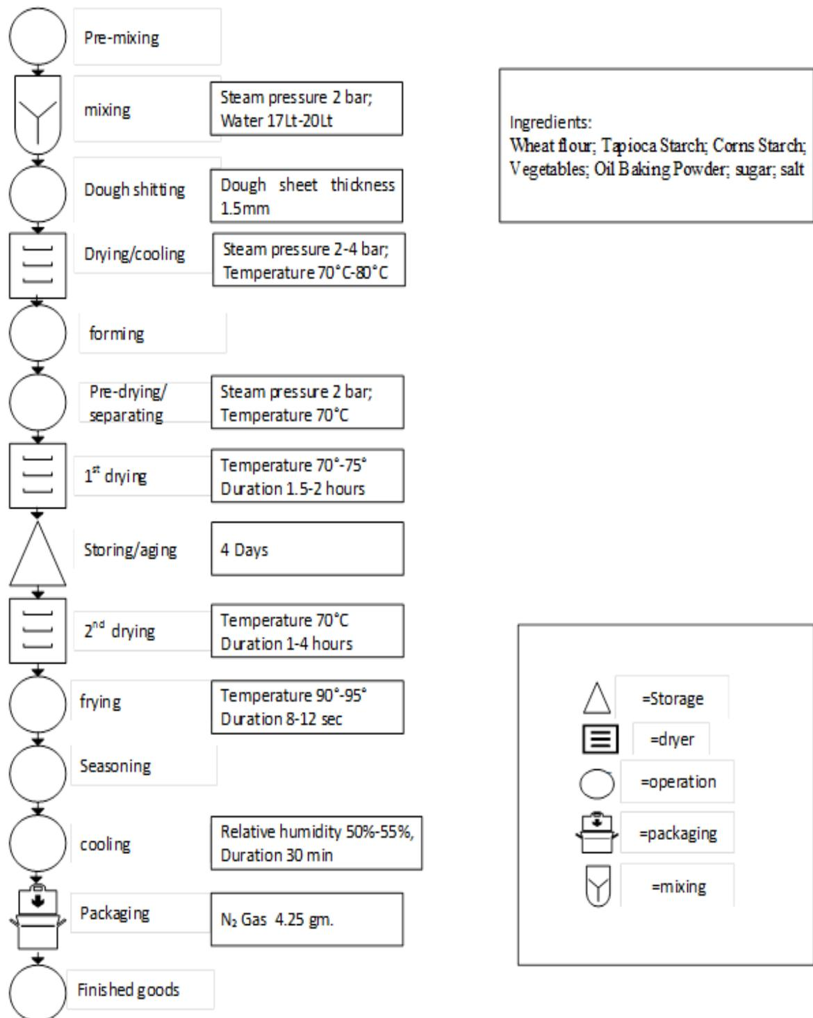
**Figure 3.** Process flow chart for 'Chicken Leg chips' Manufacturing.
