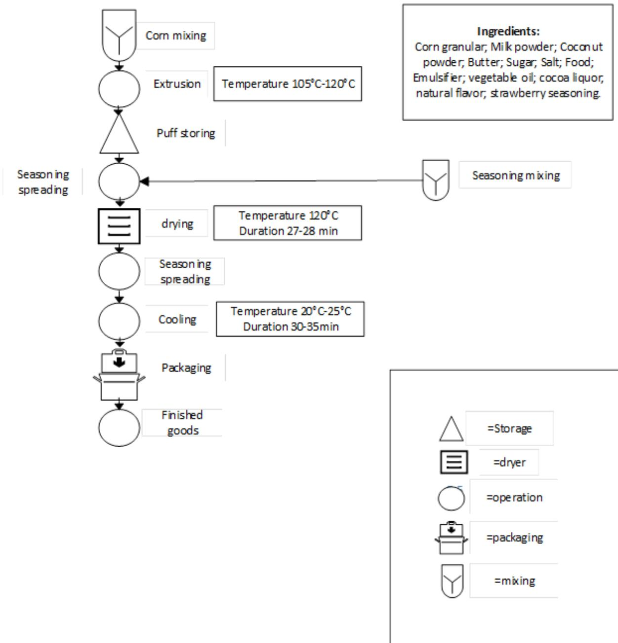
**Figure 6.** Process flow chart for ‘Choco Ring’ manufacturing.
