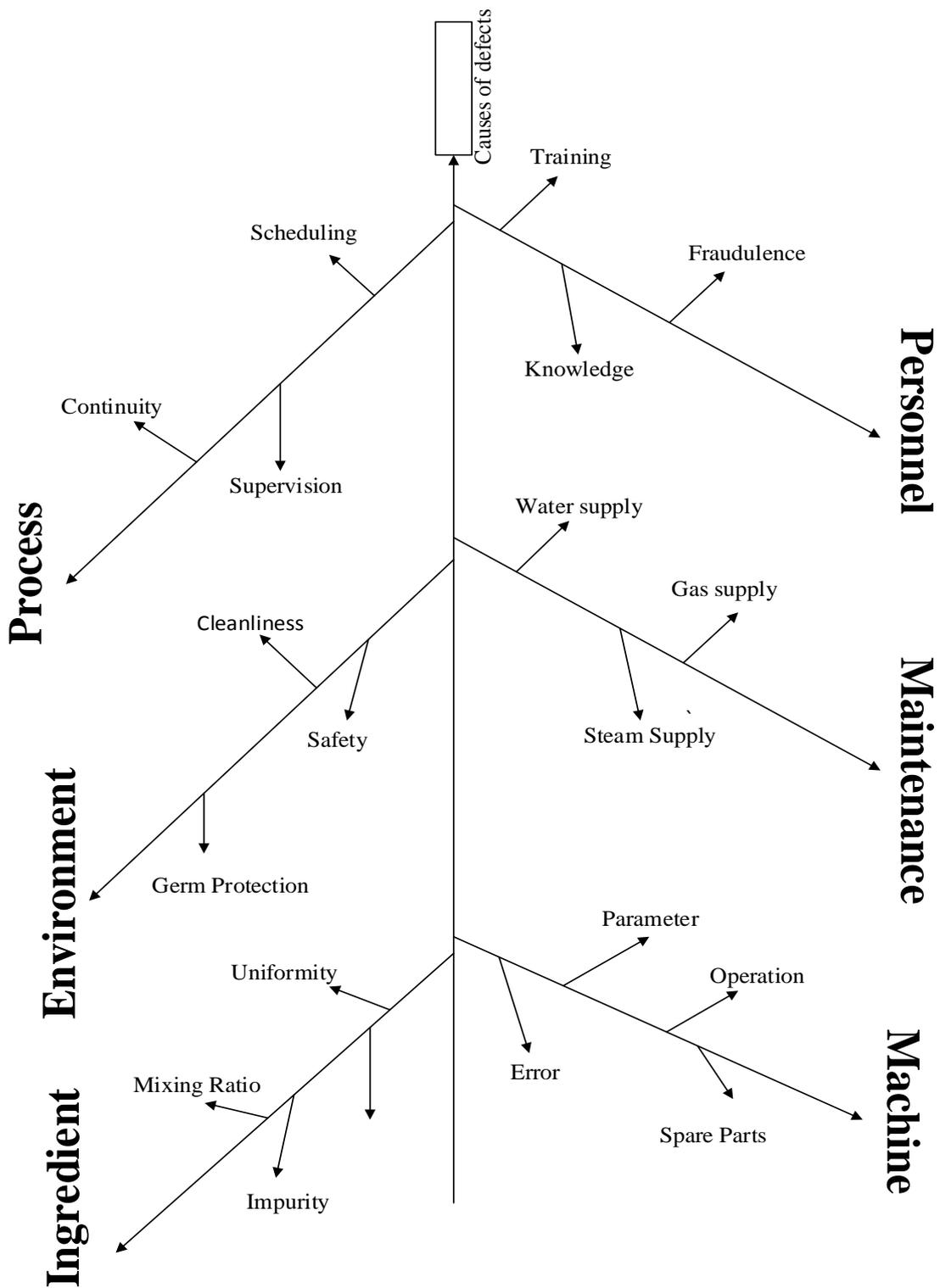
Figure 1. "Fish Bone" diagram for root cause analysis.
