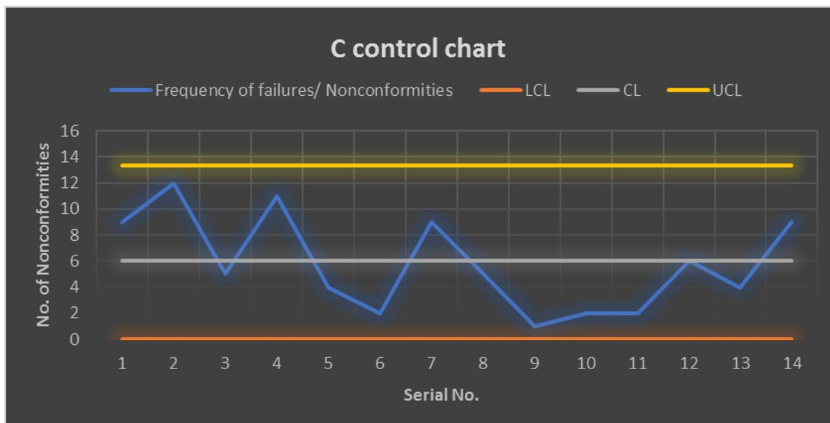
**Figure 11.** c control chart of crackers manufacturing after methodology.
