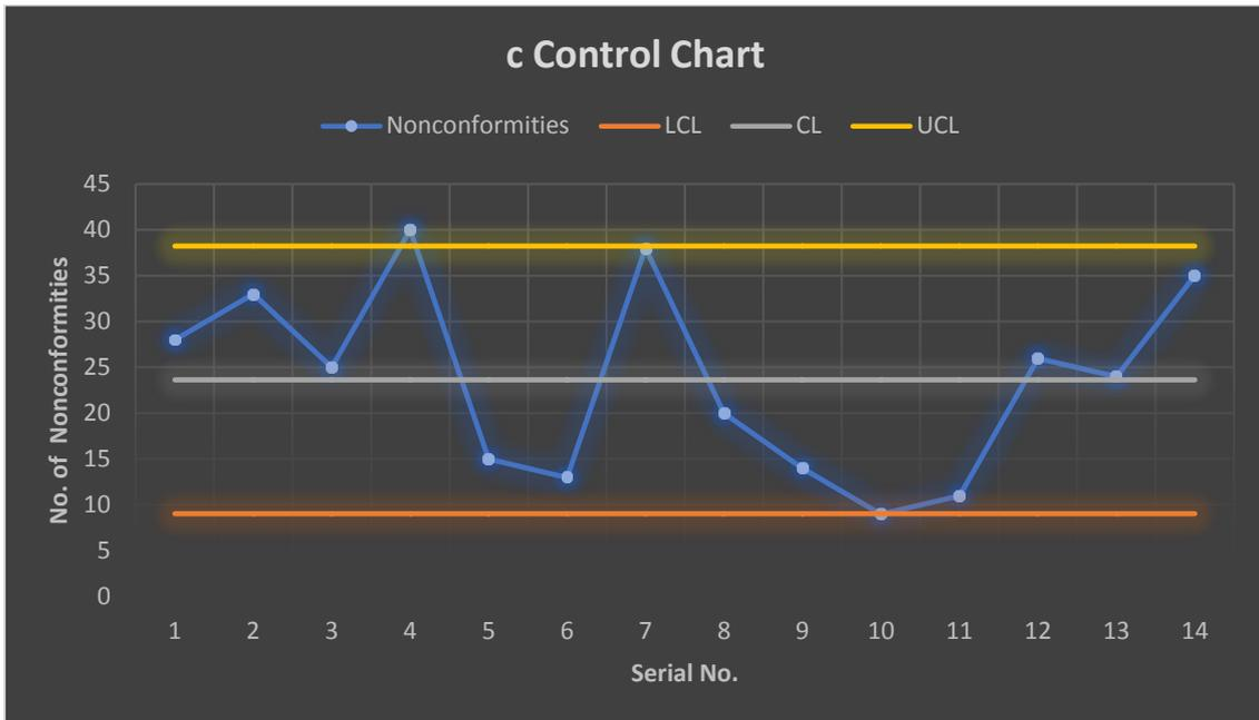
**Figure 10.** c control chart of crackers manufacturing before methodology.
