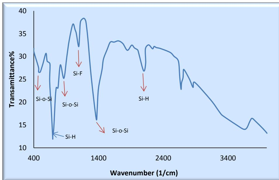
Fig. 4. FTIR spectra of the p-type porous silicon
