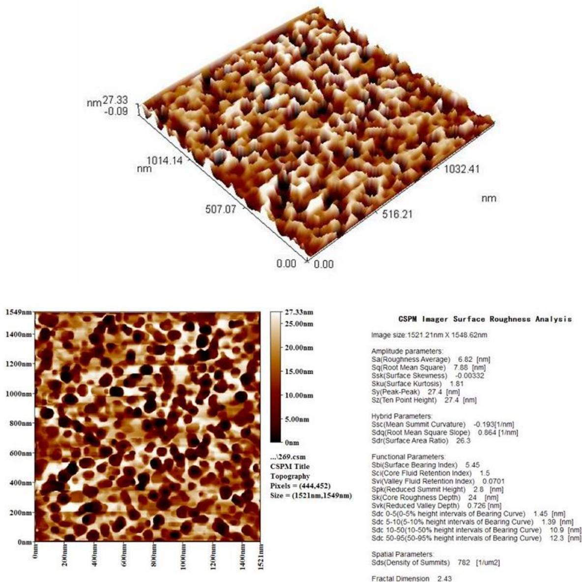
**Figure 2.** 3D & 2D AFM images ( $0.5 \times 0.5$ )  $\mu\text{m}$  of porous silicon samples prepared with etching time of (15) min at current density of (15)  $\text{mA}/\text{cm}^2$
