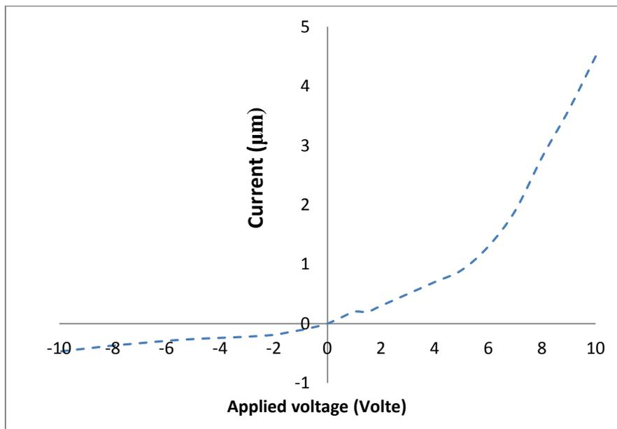
**Fig. 6.** I .V curves in  $15\text{ }\mu\text{A}/\text{cm}^2$  current density, at etching time(15) min p-type after the addition of nickel oxide
