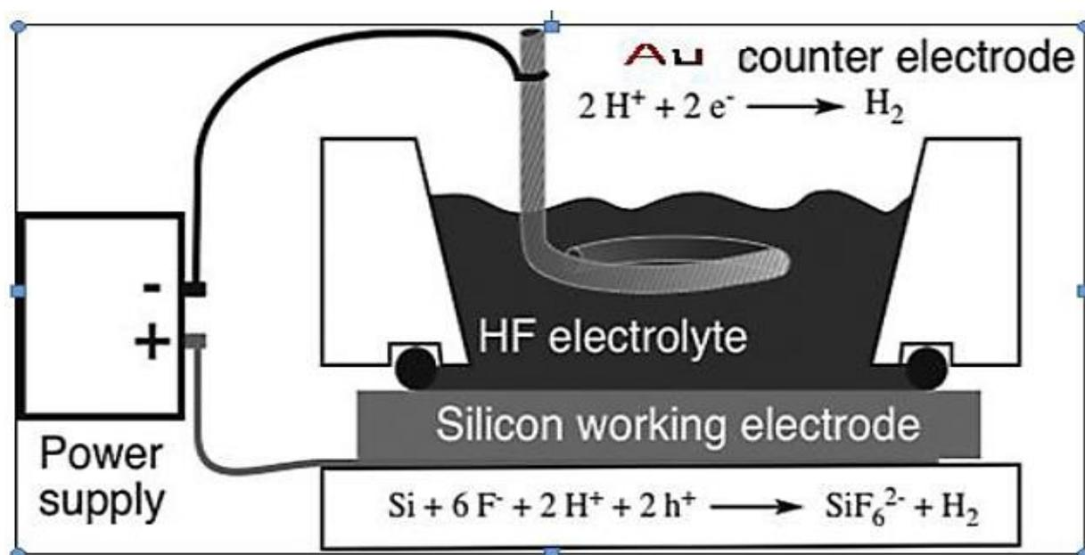
**Figure 1.** Cross-sectional view of a lateral anodisation cell [6].
