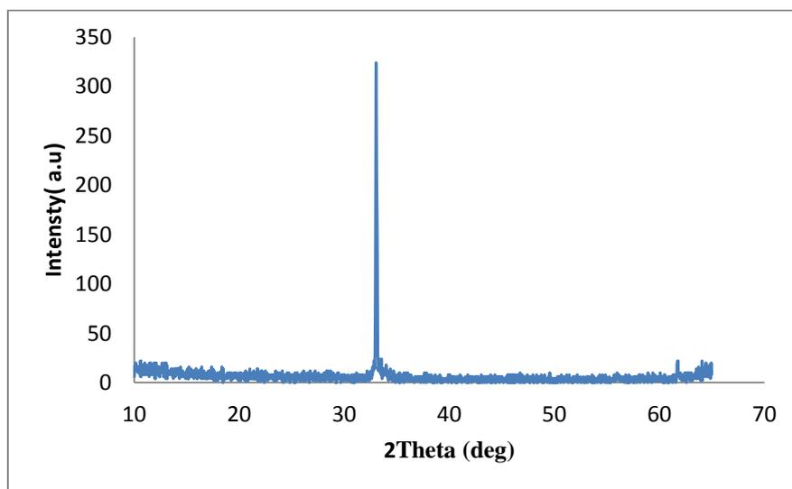
**Fig. 3.** XRD spectra of PS sample at for 15 mA/cm<sup>2</sup> current density and (15 min) etching time.
