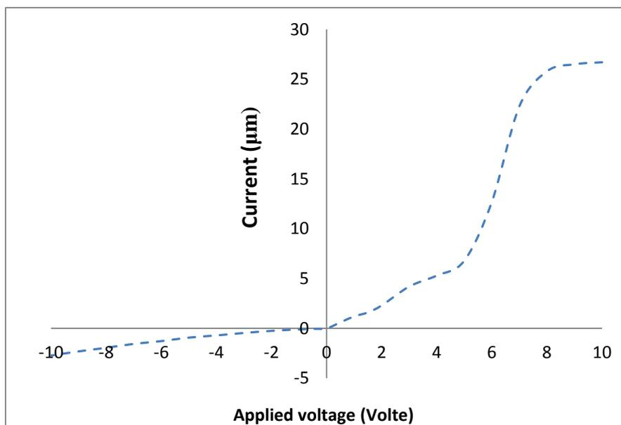
Fig. 5. I.V curves in  $15 \mu\text{A}/\text{cm}^2$  current density, at etching time (15 min) p-type before the addition of nickel oxide
