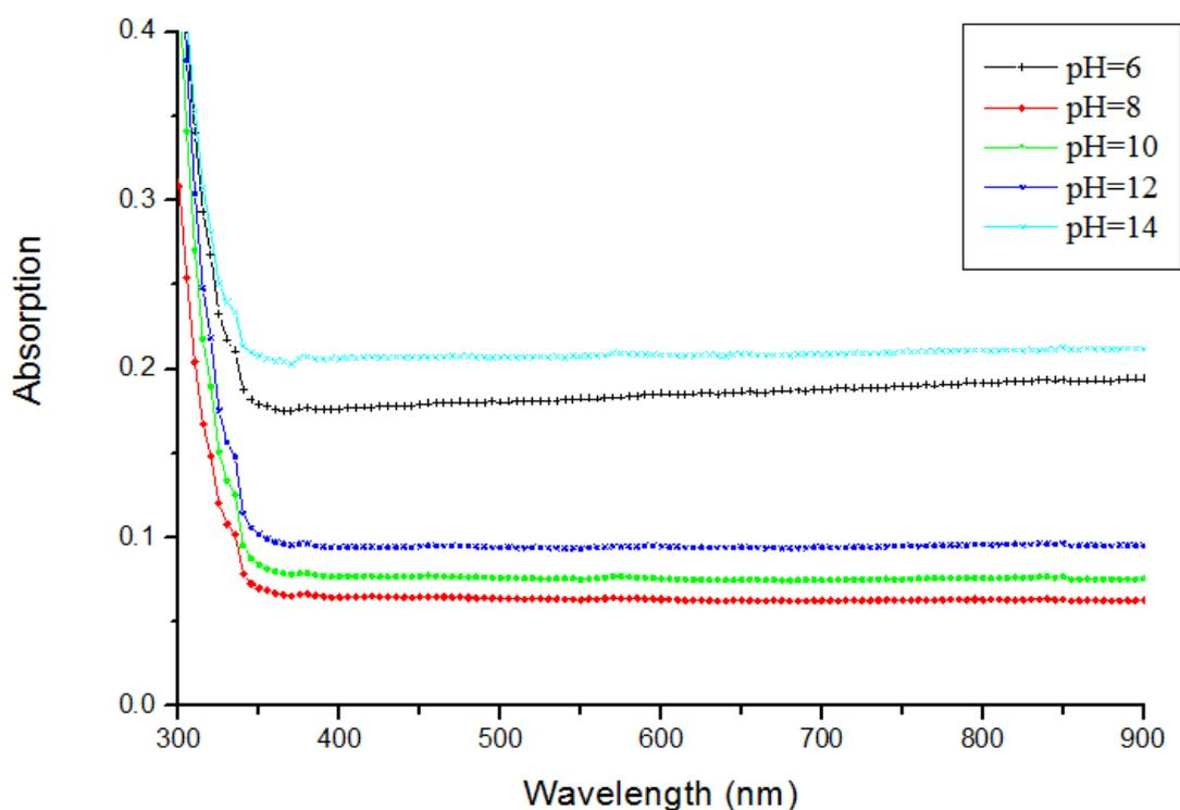
**Fig. 5.** UV-visible absorption spectrum of silver Nanoparticles (AgNPs) synthesized by reducing silver ion with ginger extract for different values of pH.
