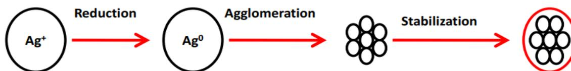
Fig. 2. Synthesis mechanism of AgNPs.
