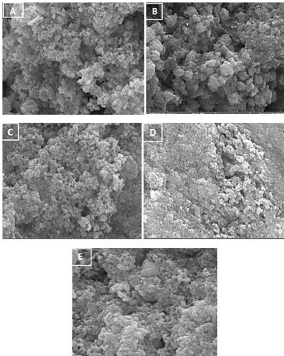
**Fig. 4.** SEM images of Ag Nanoparticles under different pH conditions
