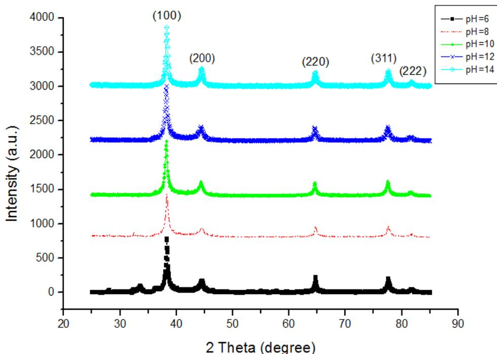
**Fig. 3.** XRD pattern of synthesized Ag nanoparticles using fresh ginger extract under different pH conditions.
