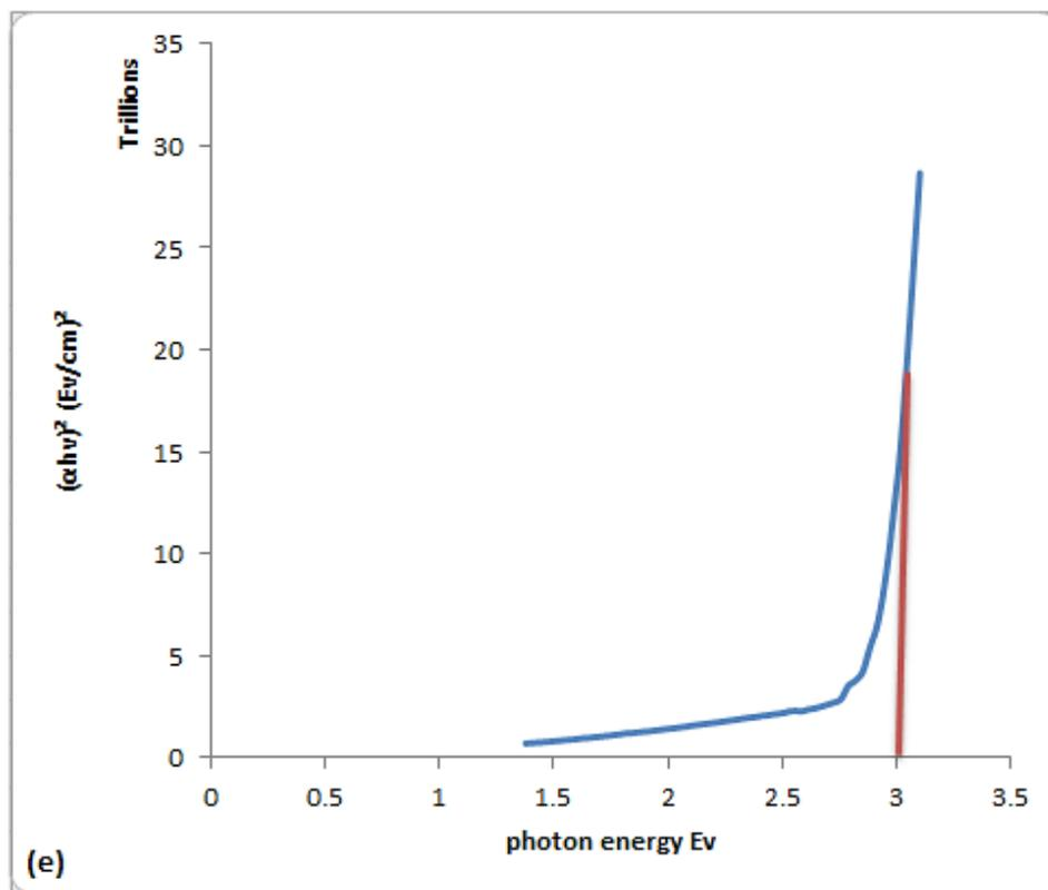
**Fig. 6.** The optical band gap of Ag nanoparticles under different pH conditions
