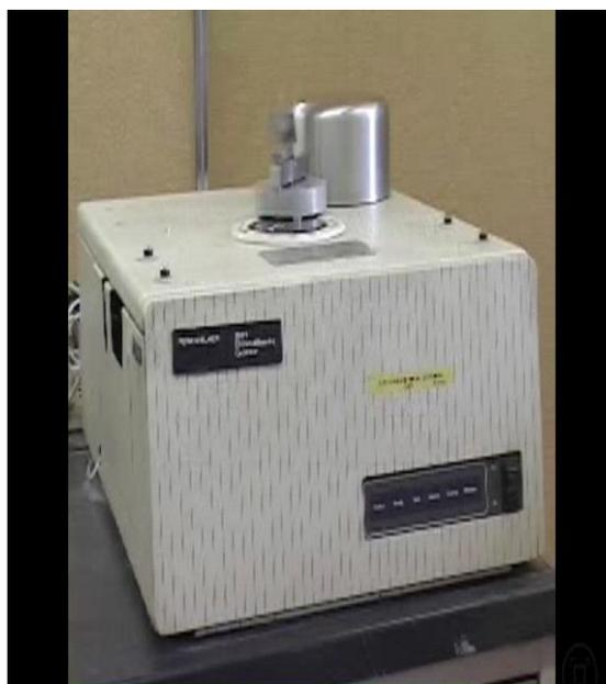
**Fig. 5.** DSC30 cell of a TC10 thermal analyzer.
