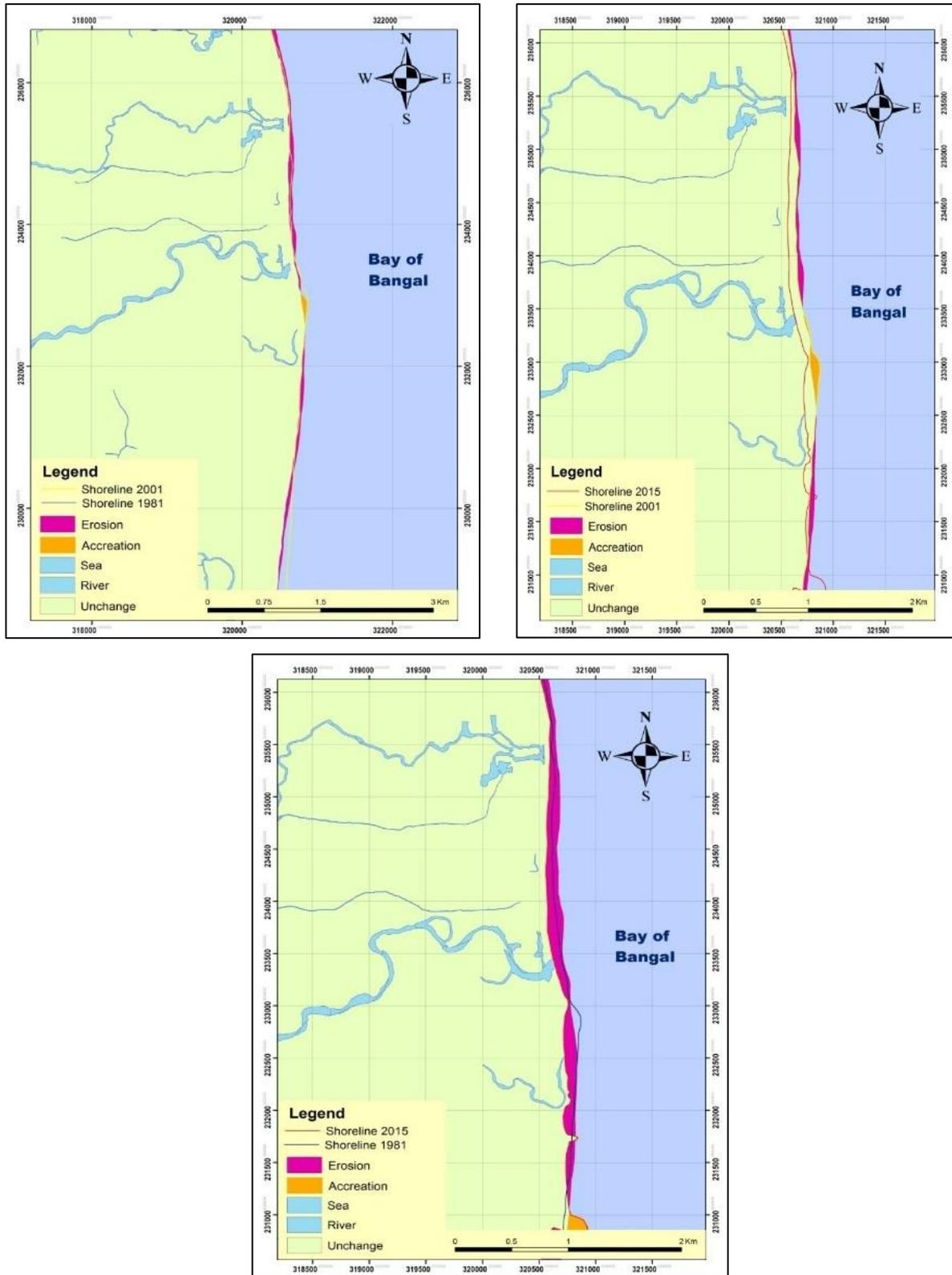
**Figure 4.** Coastal morphodynamics from 1981 to 2015 between Oluvil Harbor Northwards to Nochchiyadi
