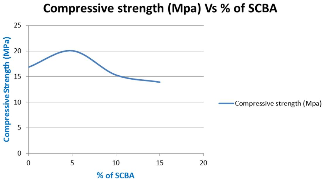
**Figure 3.** Compressive strength for 7 days.
