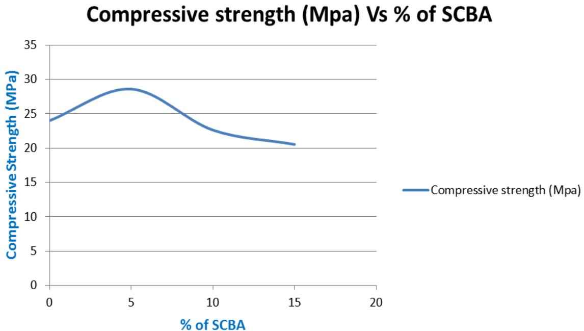
**Figure 4.** Compressive strength for 28 days.
