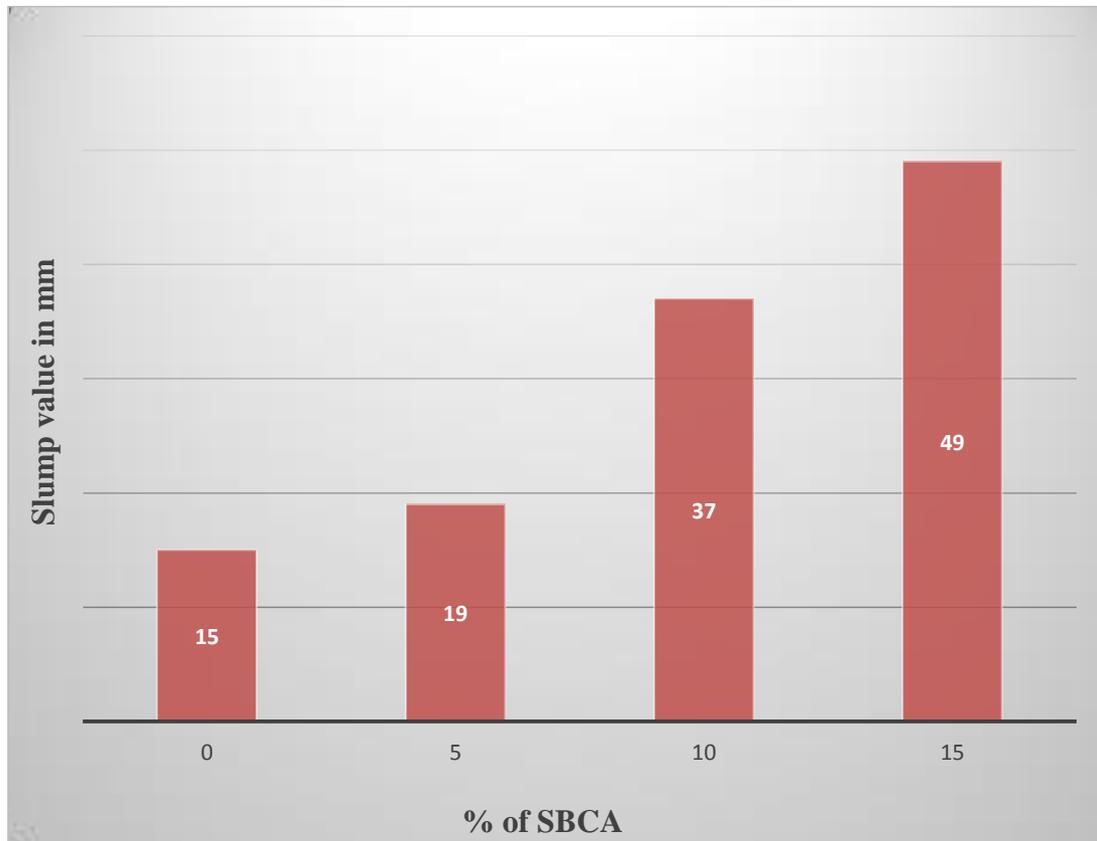
**Figure 2.** Slump value vs. % of SCBA
