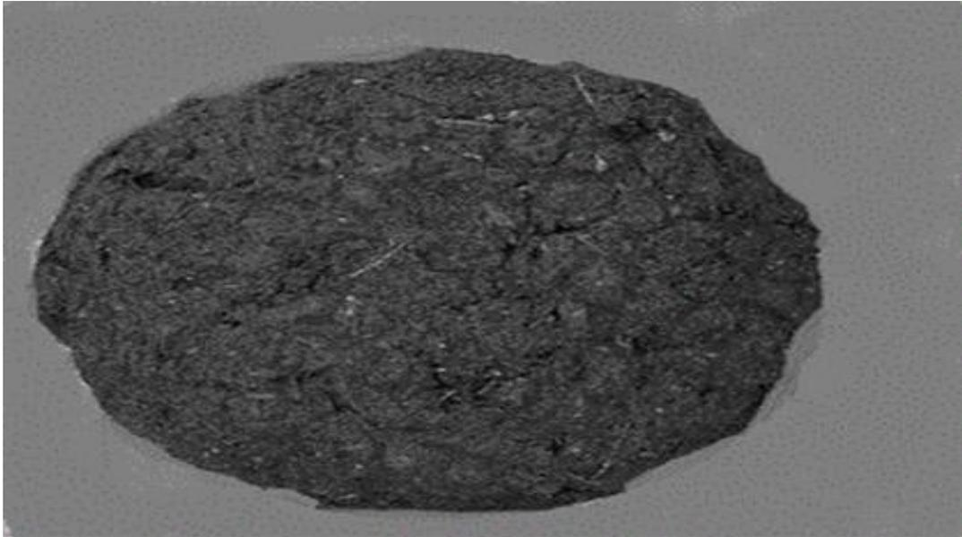
**Figure 1.** Sugarcane bagasse ash
