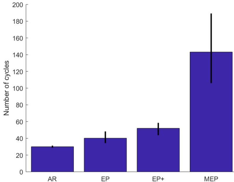
Fig. 5. Chirurgical needle bending cycles till fracture after electropolishing processes
