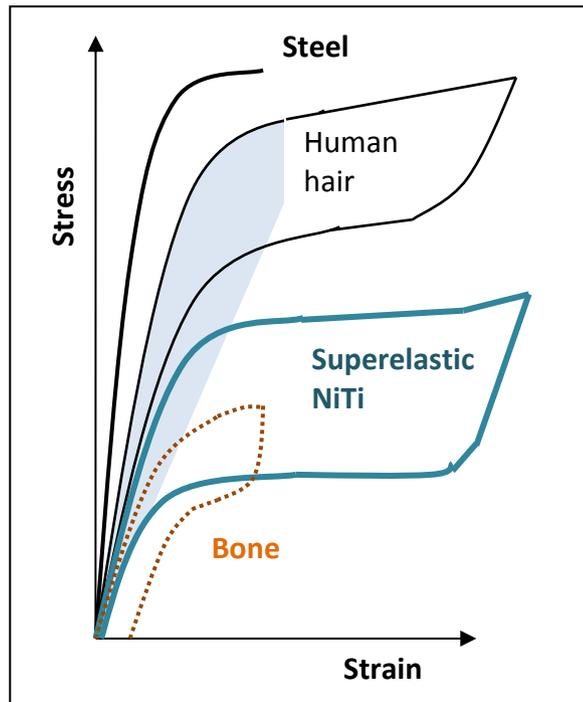
**Fig. 3.** The stress-and-strain hysteresis loop of superelastic nitinol in comparison to steel and some biological materials. When stress is released the shape of material is recovered
