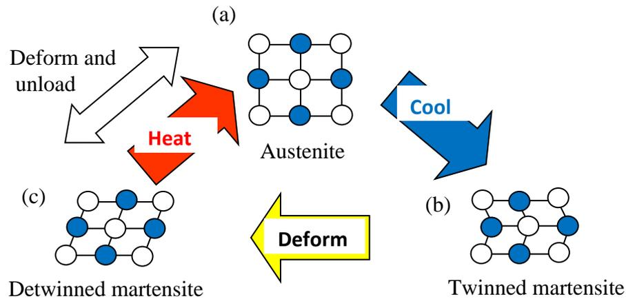
**Fig. 1.** Schematic illustration of shape memory effect
