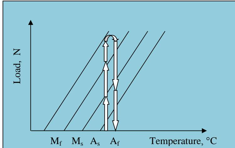
Fig. 2. Load diagram of pseudoelasticity of nitinol
