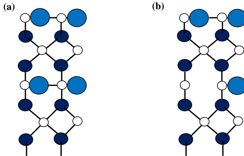
**Fig. 6.** Stick-and-ball diagram of perfect crystal lattice of TiO<sub>2</sub> (a), and defected crystal lattice with missing oxygen ion in the second row (b)
