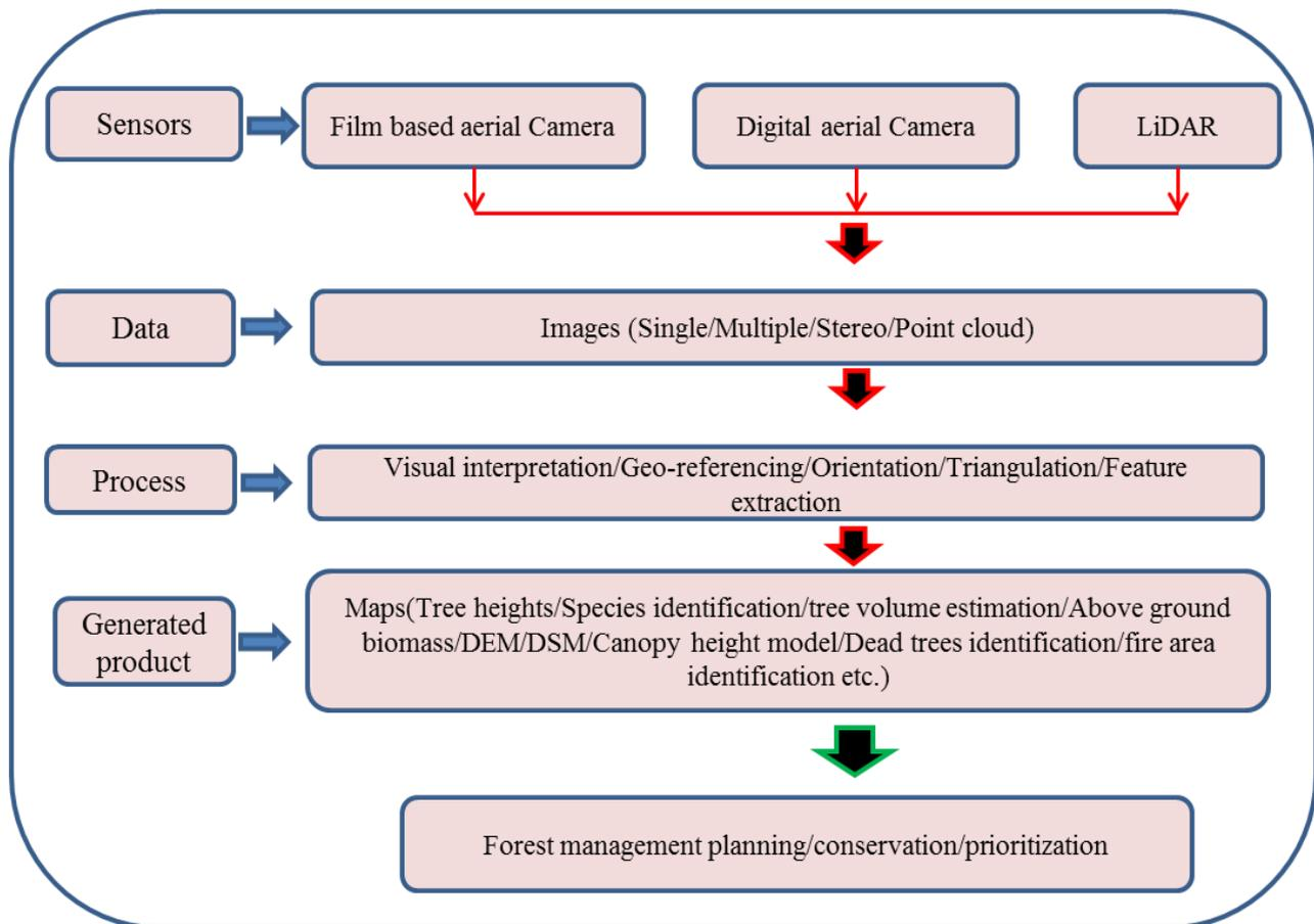
**Figure 1.** A general flow diagram of photogrammetry/LiDAR for forestry application.
