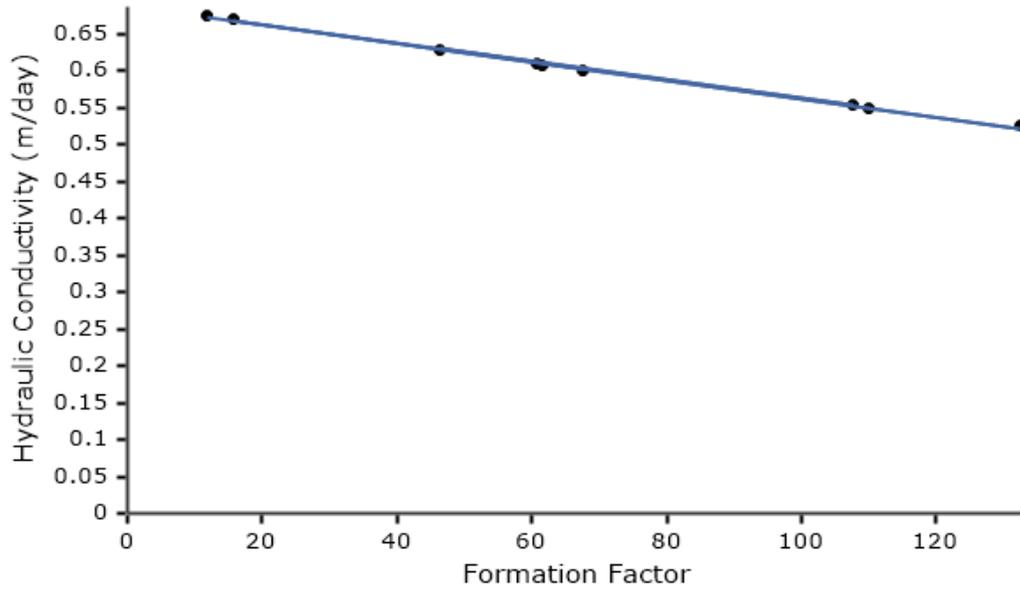
Figure 6. Linear relationship between Hydraulic Conductivity and Formation Factor
