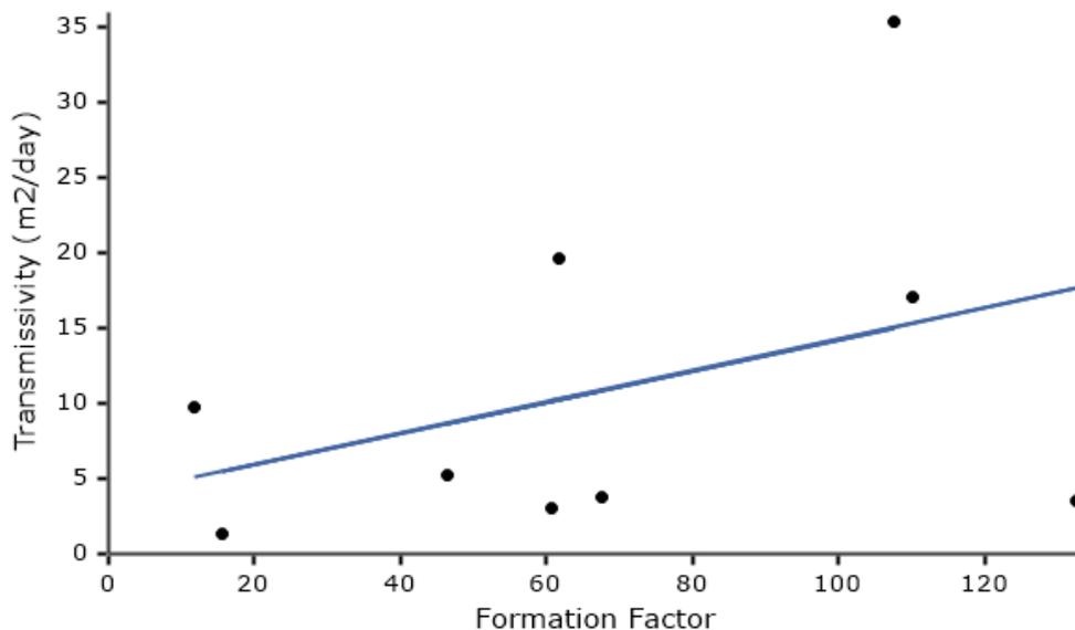
**Figure 3.** Linear relationship between Transmissivity and Formation Factor
