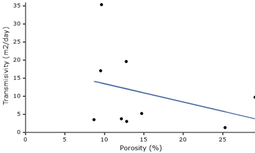
**Figure 4.** Linear relationship between Transmissivity and Porosity
