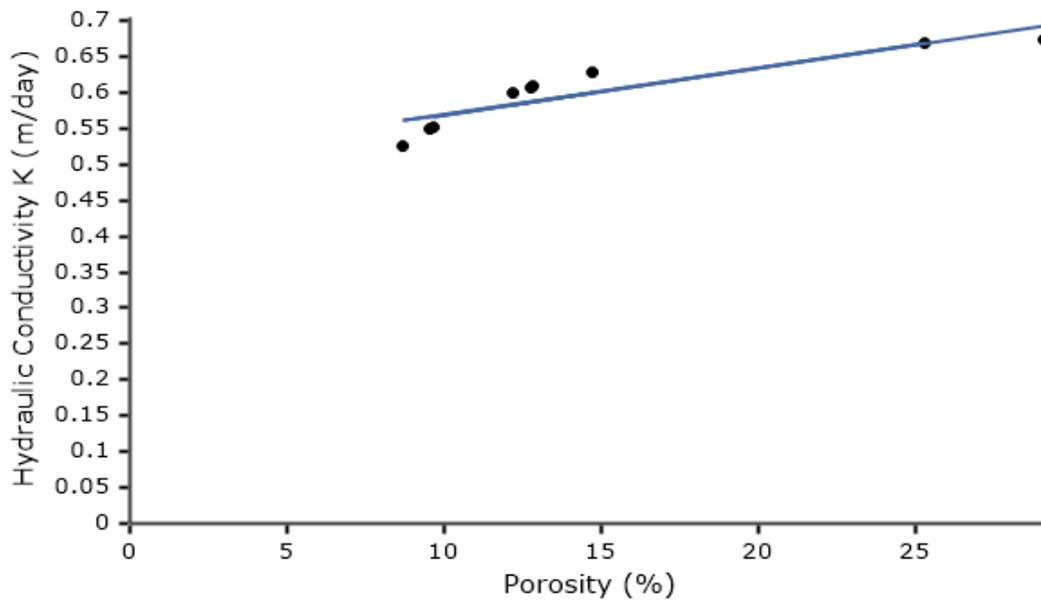
**Figure 5.** Linear relationship between Hydraulic Conductivity and Porosity
