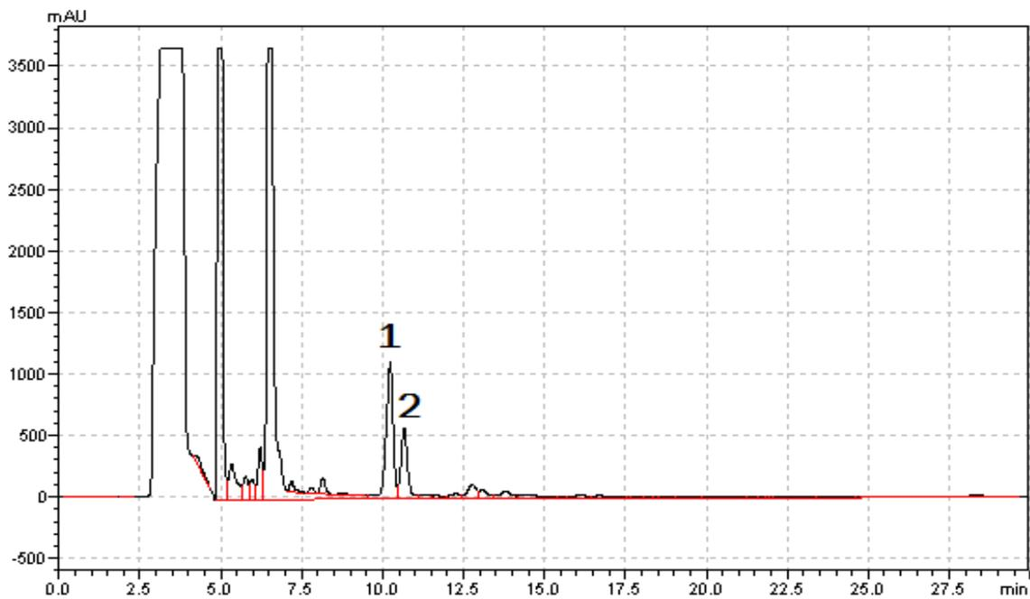
**Figure 2.** The chromatogram obtained during the analysis of whole stevia leaves from Poland, 1 - rebaudioside A, 2 - stevioside.
