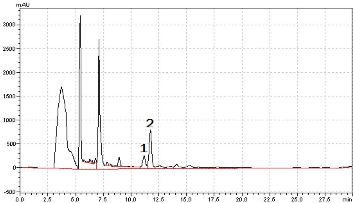
**Figure 1.** The chromatogram obtained during the analysis of shredded stevia leaves from European Union countries, 1 - rebaudioside A, 2 - stevioside.
