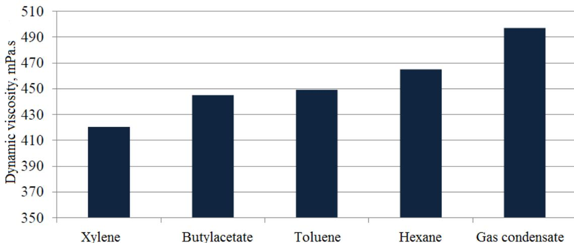
**Figure 2.** Change of dynamic viscosity of oil of the field Shikbagi after introduction of 2% of mass reagent
