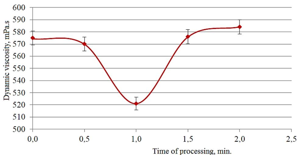
**Figure 1.** Change of dynamic viscosity of crude oil of the field Shikhabagi depending on test processing time
