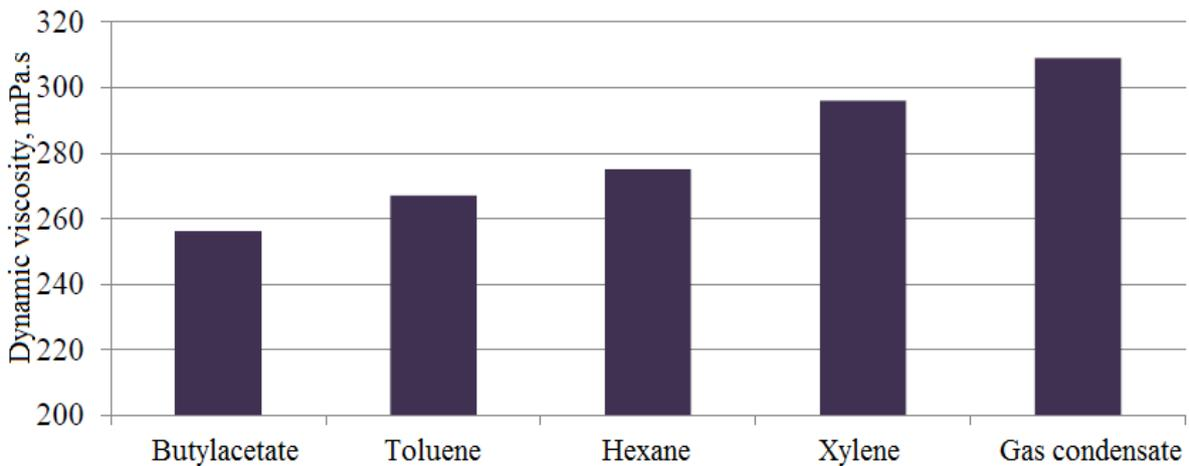
**Figure 5.** Change of dynamic viscosity of oil of the field Bulla-deniz after introduction of 2% of mas reagent
