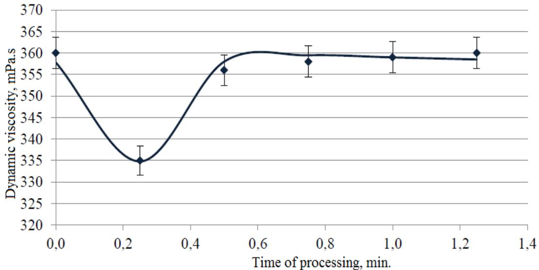
**Figure 4.** Change of dynamic viscosity of crude oil of the field Ashchisay in dependence on test processing time
