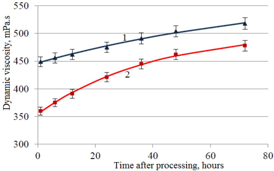
**Figure 3.** Change of dynamic viscosity of oil of the field of Shikbagi from a test storage time after introduction of 2% of masses. toluene and hashing: 1-without cavitation processing; 2-after cavitation processing
