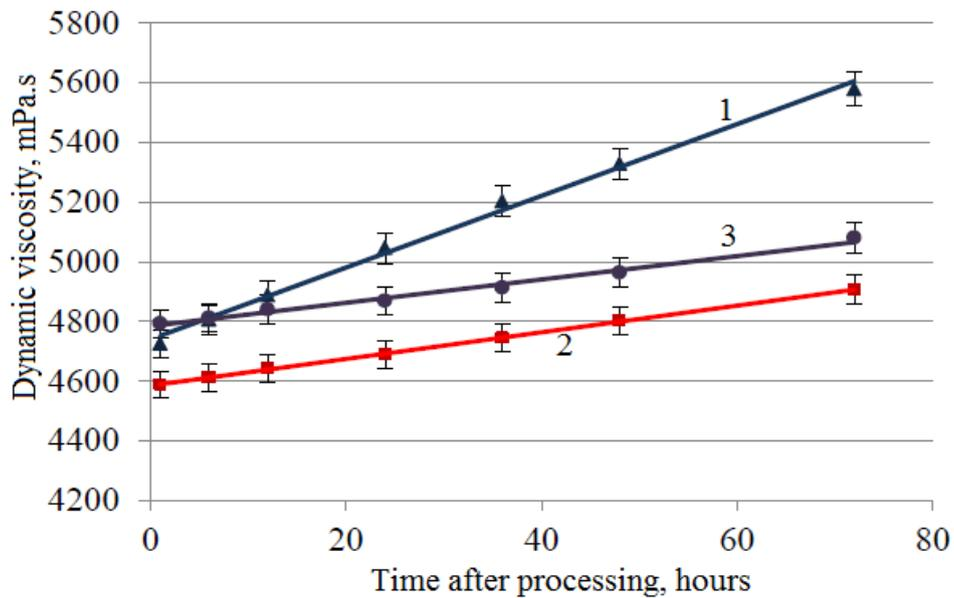
**Figure 7.** Change of dynamic viscosity of oil of the field Shirvan from a test storage time after introduction of 2% of mass. butylacetate and hashing: 1 – without cavitation processing; 2 – after cavitation processing within 1 min.; 3 – after cavitation processing within 3 min.
