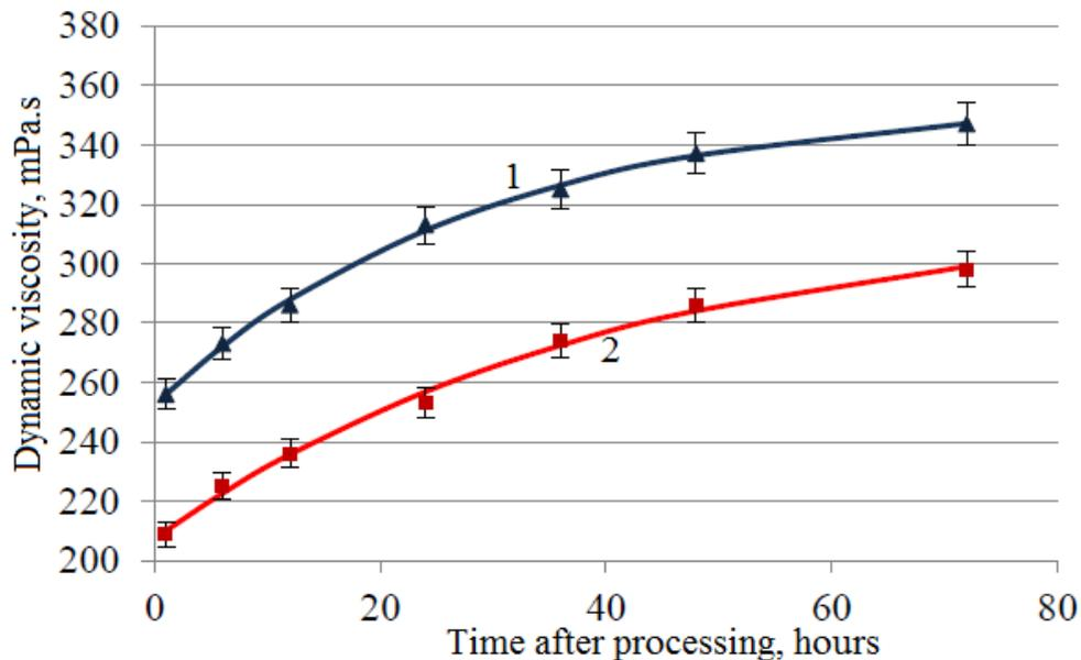
**Figure 6.** Change of dynamic viscosity of oil of the field Bulla-deniz from a test storage time after introduction of 2% of masses. butylacetate and hashing: 1 – without cavitation processing; 2 – after cavitation processing
