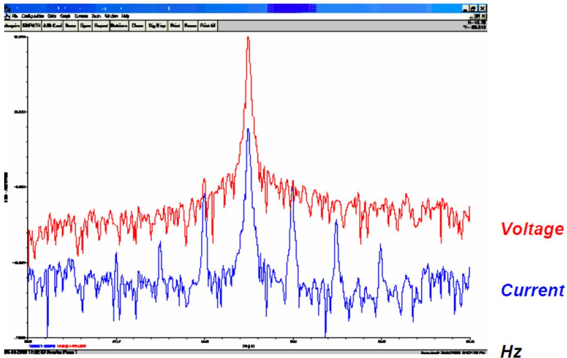
Figure 3. Spectrum of severely damaged rotor
