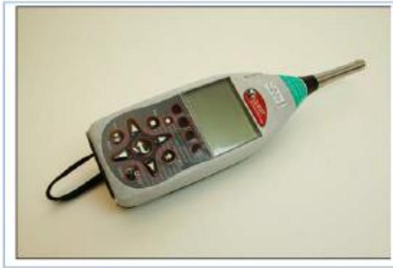
**Figure 5.** Acoustic noise meter
